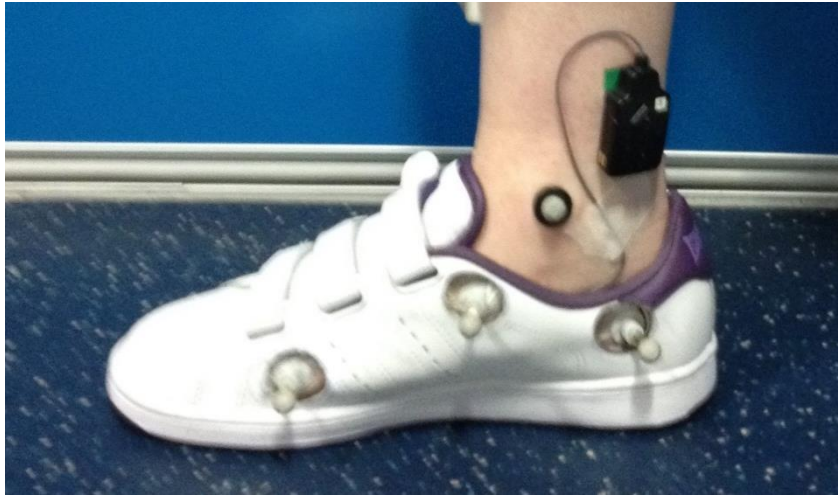
Figure 4-11. Marker set up showing the wand markers on the 1 st metatarsal head, navicular tuberosity and the medial aspect of the calcaneus for medial longitudinal arch angle calculation
