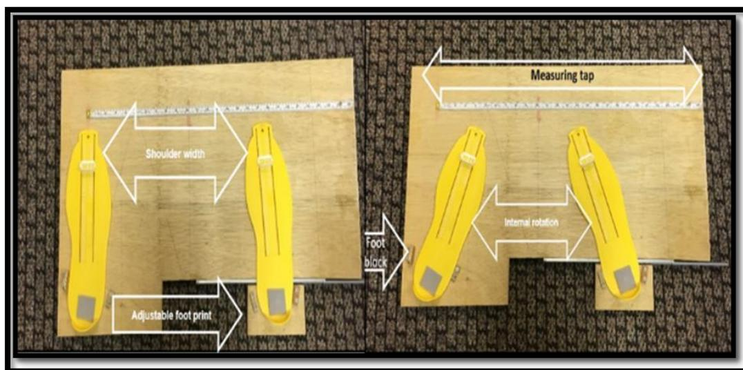
**Figure 4-10:** Feet standardisation tool. This allows each participant to stand with their feet at shoulder width apart and provides a consistent 20° of internal rotation.
