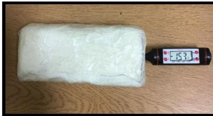
**Figure 6-5:** A thermometer was inserted into the lard for measuring the internal temperature. The results showed that the lard had a stable HU at room temperature. Moreover, at room temperature the CT density of lard was -100 HU which was closer to human adipose tissue. Even at the freezer temperature (-14°C) the CT density was -64 HU which is within the range of the fat HU previously reported in the literature (see **Figure 6-6**).
