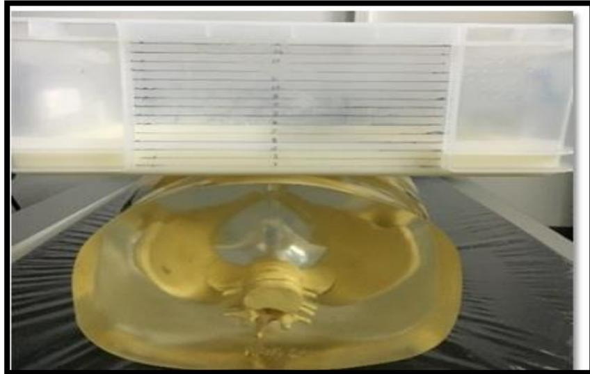
**Figure 6-9:** Experimental setup for the pelvis phantom and additional fat container (scaled 1 cm increment box). This photograph is taken from the superior aspect of the phantom looking inferiorly.
