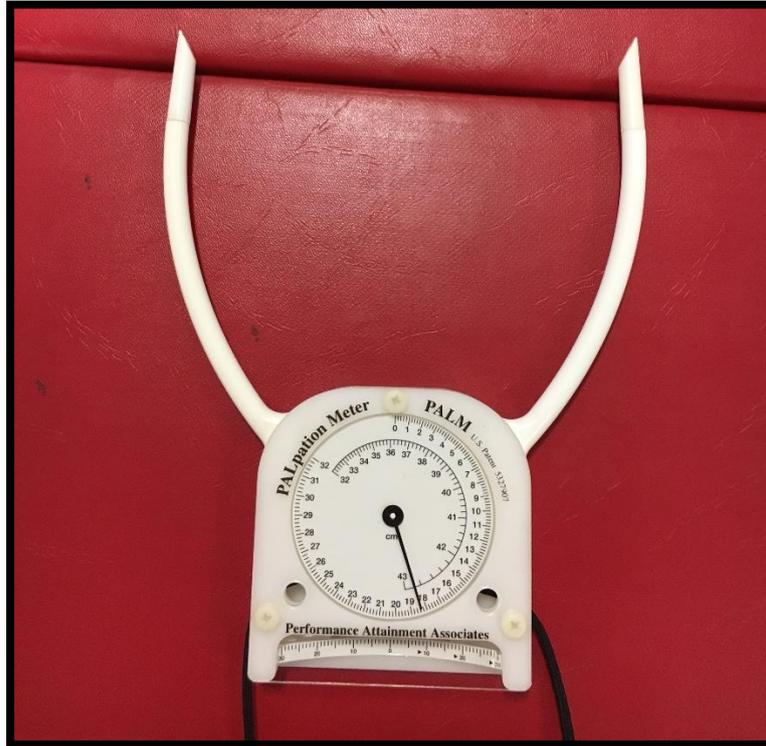
**Figure 4-4:** Inclinator and its main components (Palm meter).
