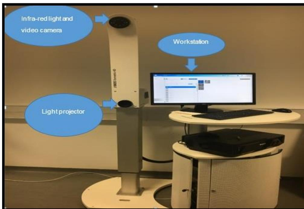
**Figure 4-6:** Diers system. This consists of a recording camera and light projector. The uneven back surface alters the straight projected light. The camera detects this distorted light from different angles of view and undertakes measurements.
