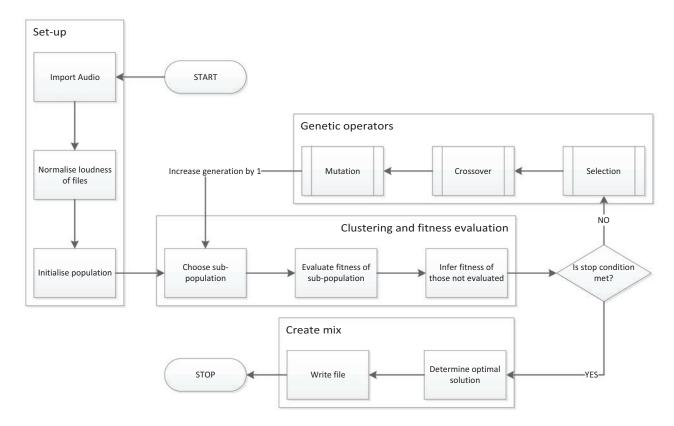
Fig. 1. Flowchart illustrating the design of the system.
