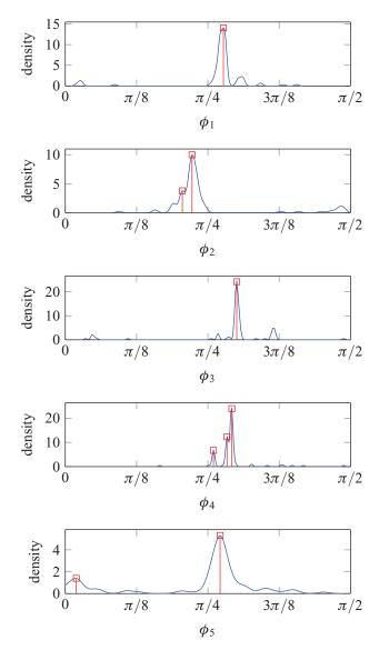
Fig. 4. Univariate KDE result from one of the sessions. Peaks in each distribution are marked. Taking the greatest peak in each provides a 5-element  $\Phi$  vector (on  $\mathbb{S}^5$ ) which is transformed to a 6-element gain vector (in  $\mathbb{R}^6$ ).
