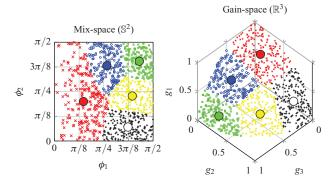
Fig. 2. 1,000 solutions to a 3-track mixing problem, clustered using spherical *k*-means. The solutions closest to each of the cluster centroids form the sub-population to be evaluated, and the fitness of remaining samples is inferred based on these ratings and distance to the centroid.
