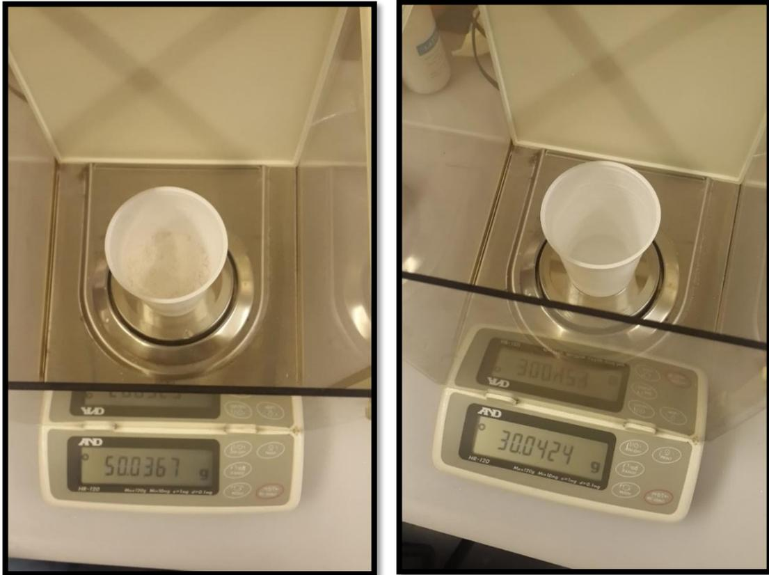
Figure 4.6: The scale used to weigh the plaster powder (on the left) and the water (on the right).
