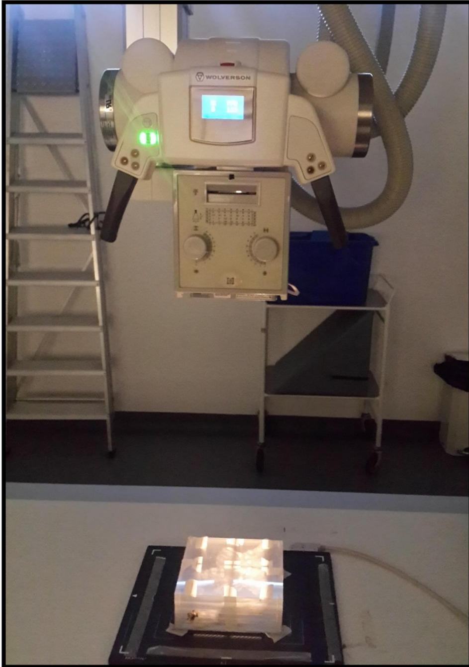
Figure 5.1: Experimental setup of the 1-year-old phantom, DR detector and X-ray tube.
