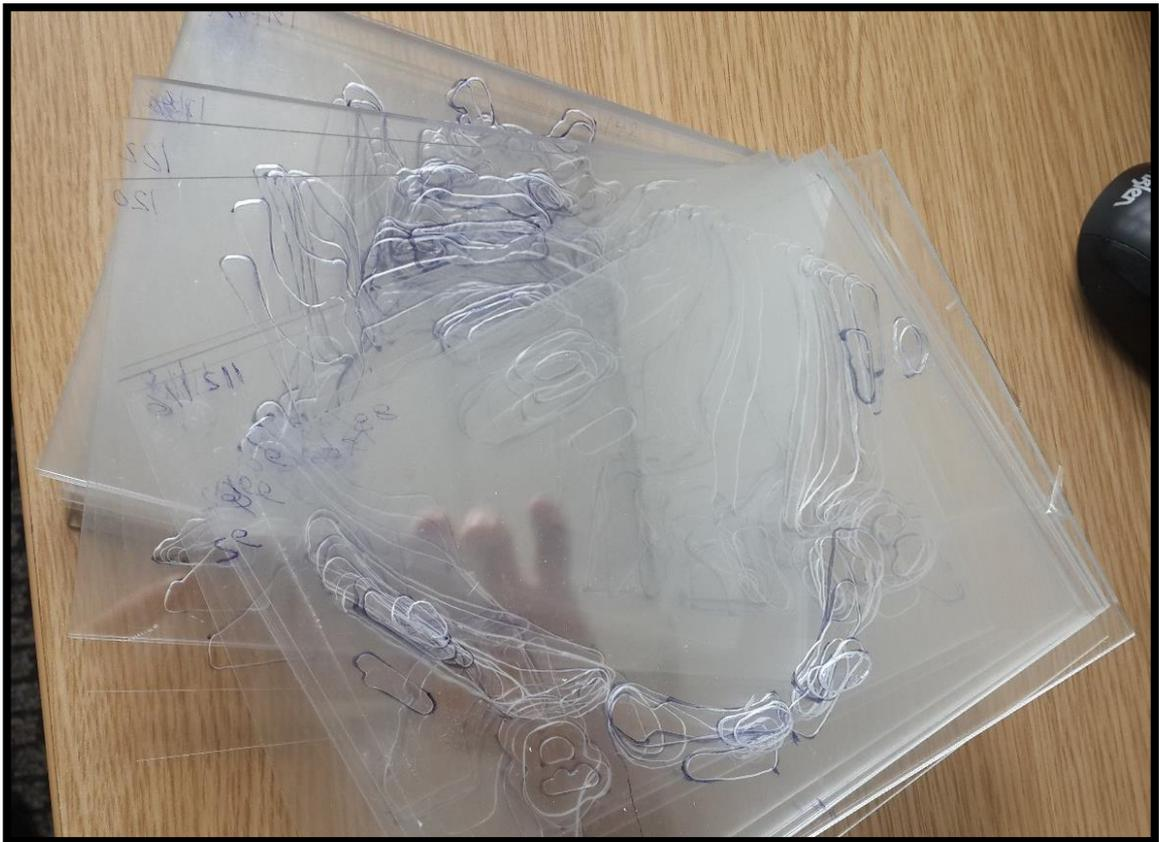
Figure 4.1: An illustration of the PMMA sections used to form the first prototype phantom. Within each slice, shapes have been removed (using a milling machine) from which PVC (bone) shapes would be inserted.
