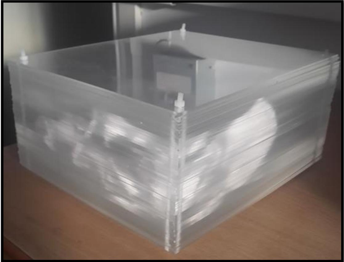
Figure 4.8: All of the PMMA slices assembled together.
