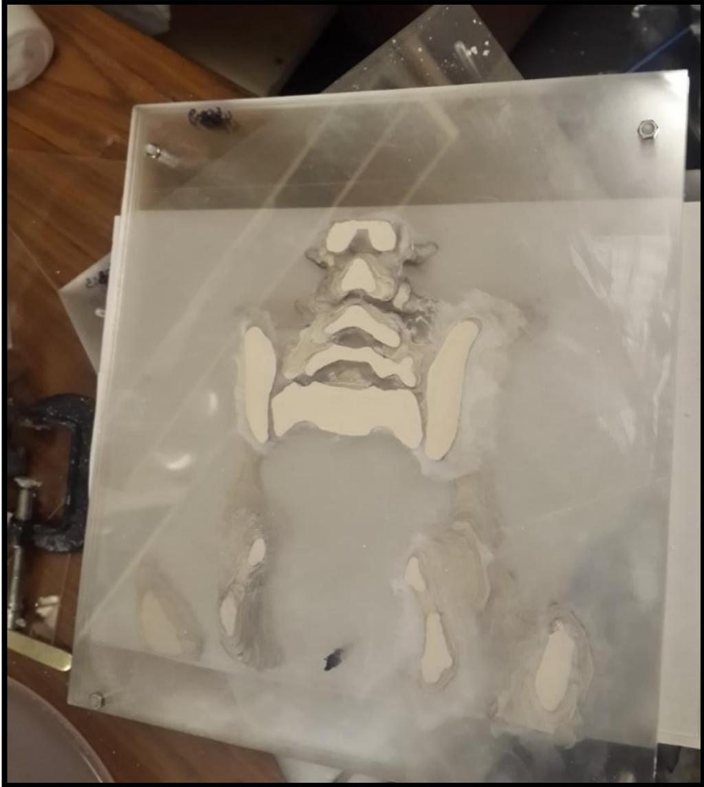
Figure 4.7: PMMA block filled with PoP and flattened to the PMMA surface.
