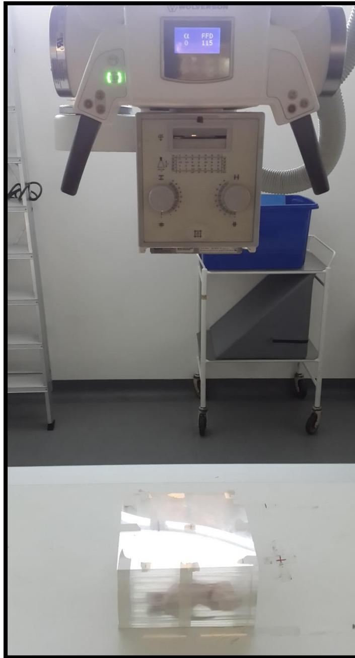
Figure 5.3: Experimental setup of the 10-year-old phantom and X-ray tube. The table Bucky was used for **all** examinations involving this phantom.
