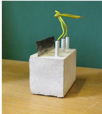
**Figure 5.1** Configuration of CP experimental specimen (Oleiwi, 2018).
