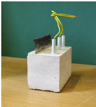
**Figure 6.1** Configuration of CP experimental specimen (Oleiwi, 2018).
