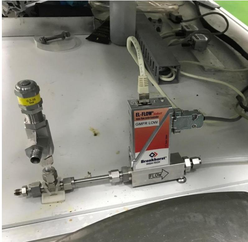
Figure 4.23 Bronkhorst mass flow meters and a pressure relief valve
