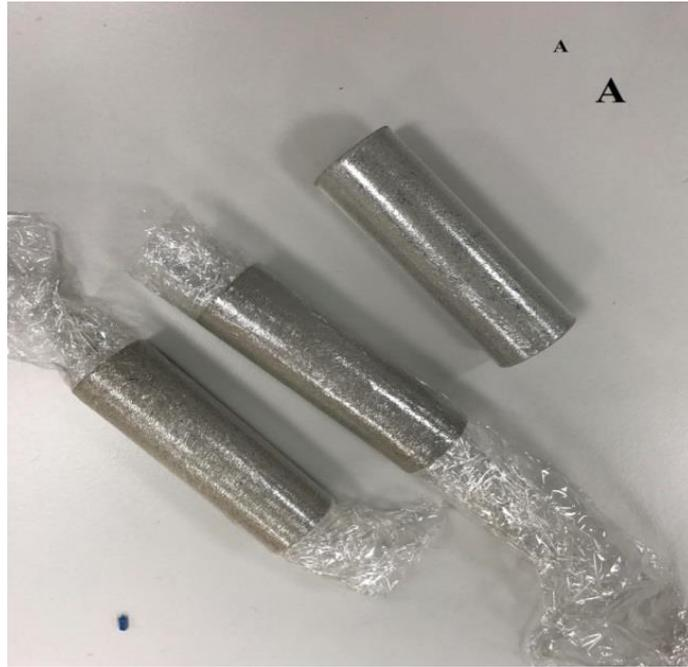
**Figure 3.5** Process of core samples wrapping in cling film
