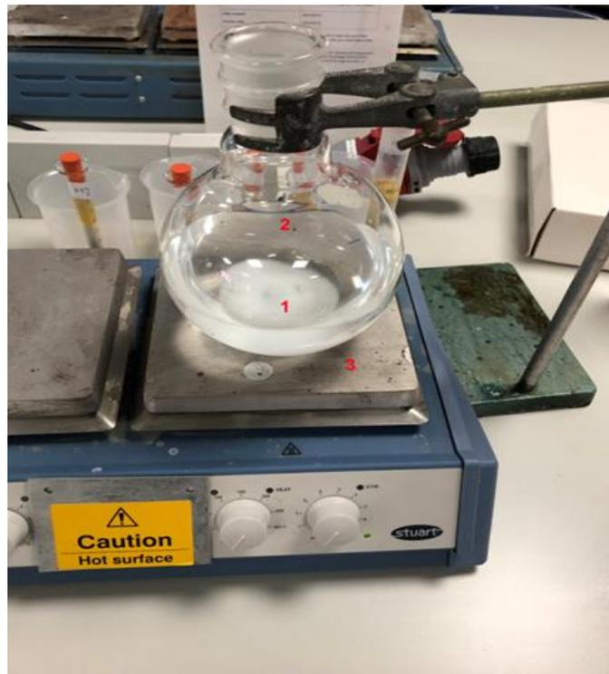
Figure 3.3 Brine preparation set up
