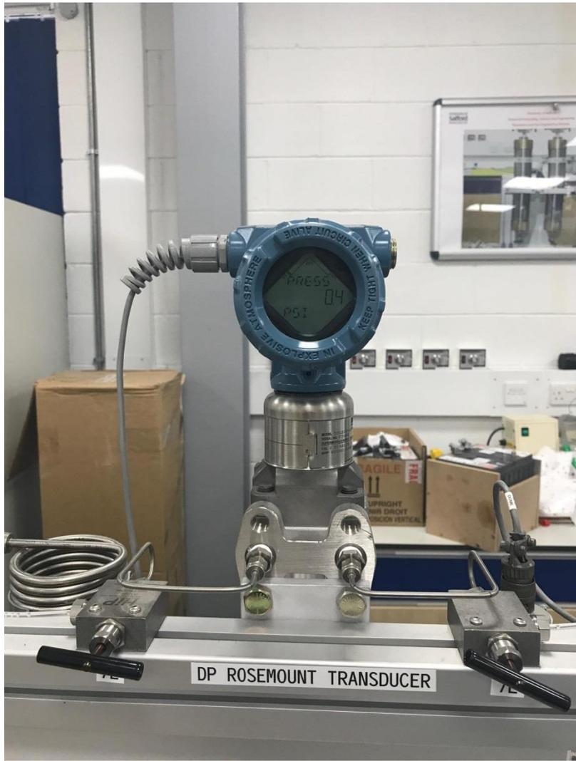
**Figure 4.22** Rosemount pressure transducer system
