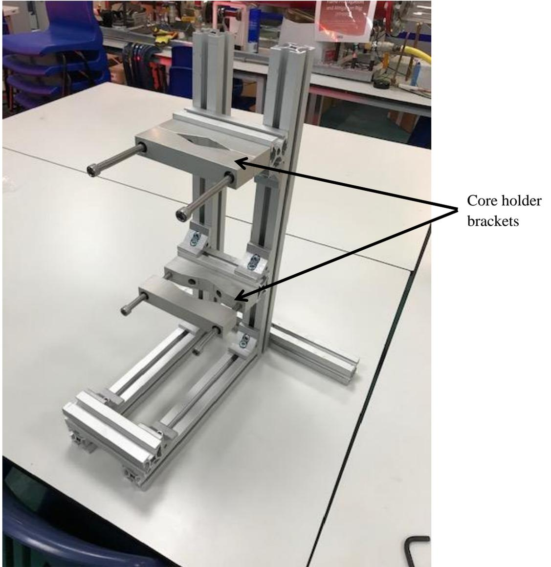
**Figure 4.26** Constructed stand for the core holder to be situated vertically
