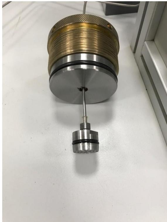
**Figure 4.17** Fixed end component of the core holder showing the distribution plug
