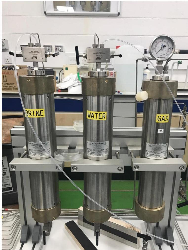
**Figure 4.21** Floating piston accumulators and a gas humidifier
