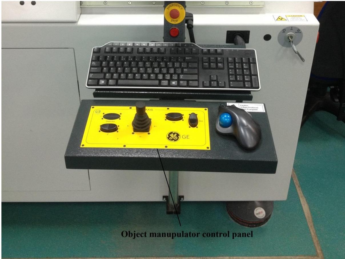
**Figure 4.8** Object manipulator control panel of the CT scanner
