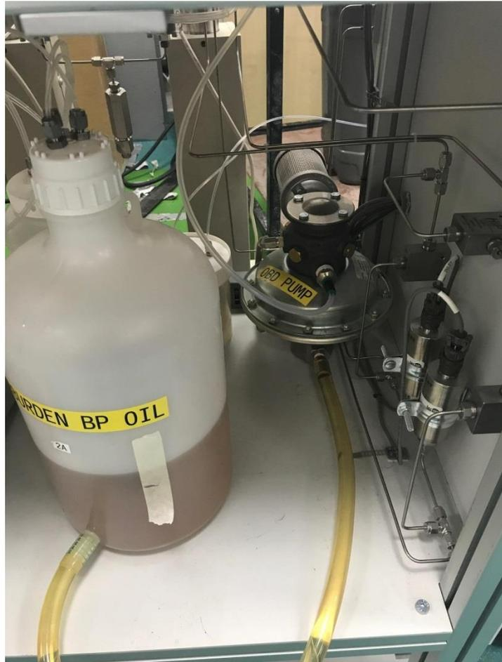
**Figure 4.20** Hydraulic pump Model S-216-JN-150 with hydraulic oil reservoir
