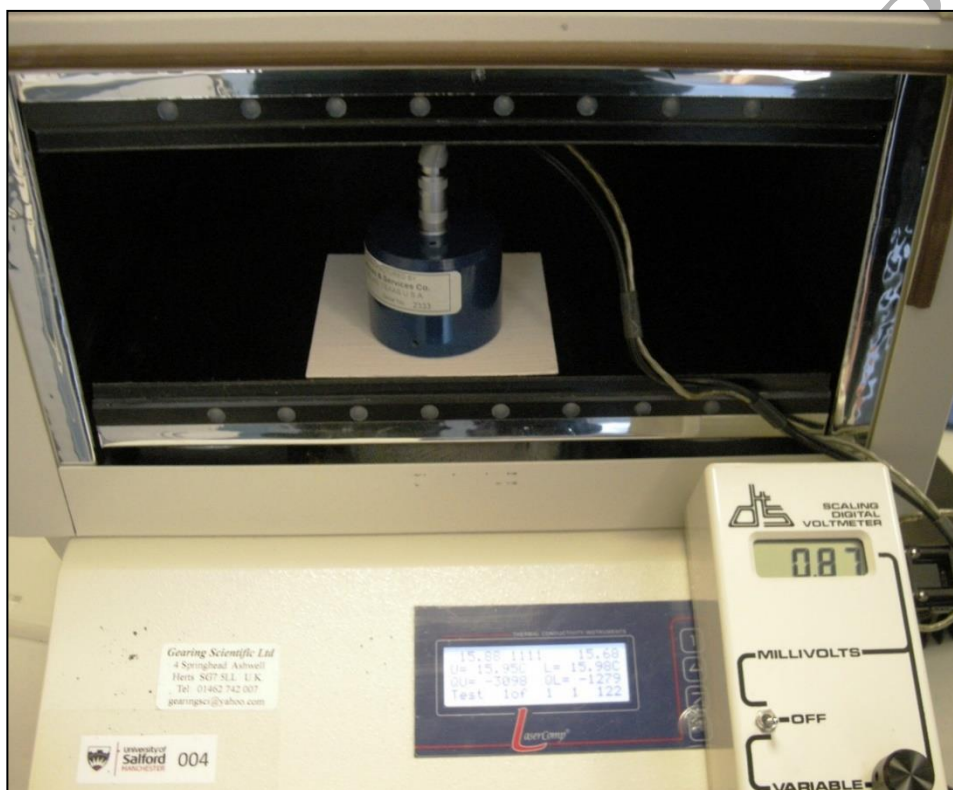
Figure 14 Emissometer mounted on a coated sample in constant temperature heat flow meter apparatus
