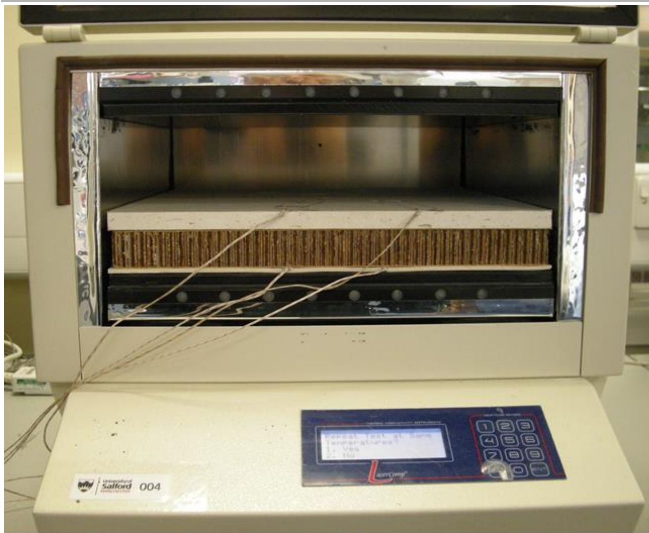
Figure 15 Composite sample being assembled in the heat flow meter apparatus, with thermocouples on both faces and contact sheet on hot plate
