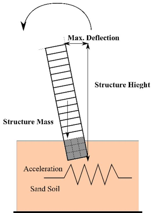
**Figure 6-14 Soil-foundation-structure interaction moment of structure on raft foundation**
