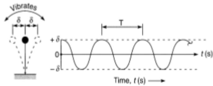
Figure 2-4 Undamped free vibrations of a single degree of freedom system (Taranath, 2009; Clough and Penzien, 2013)
