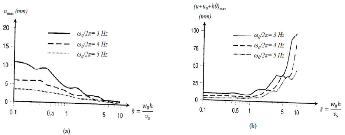
**Figure 2-12 Response of the equivalent soil-structure system: (a) maximum structure demand, (b) maximum total displacement of the structure relative to the free field ground motion (Wolf and Oberhuber, 1985)**
