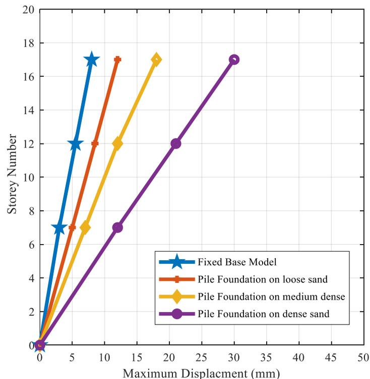
**Figure 6-8 Effects of soil properties on maximum displacement (raft-on-pile foundation)**
