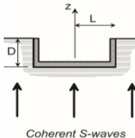
**Figure 2-9 Embedded raft foundation (Stewart, 1999)**
