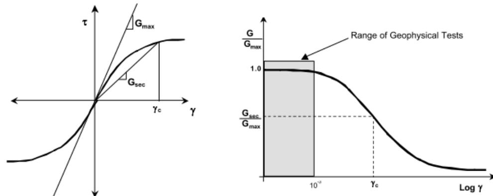
**Figure 2-8 Stress-strain curve with a variation of shear modulus and modulus reduction curve (Tabatabaiefar and Massumi, 2010)**
