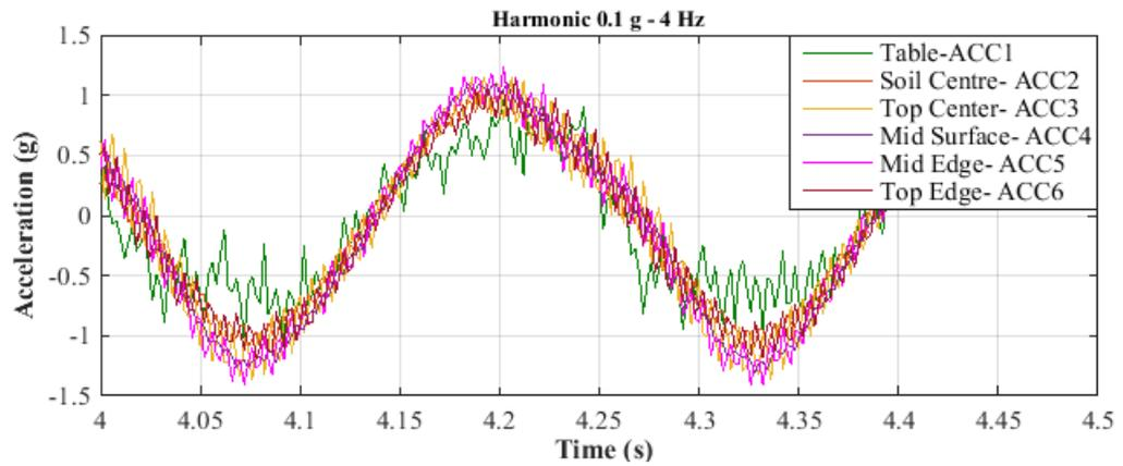
Figure 3-17 The effect of the container boundary of the soil response
