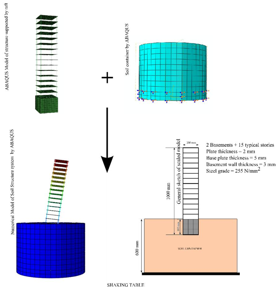
Soil Foundation Structure Interaction ( Raft Foundation)
