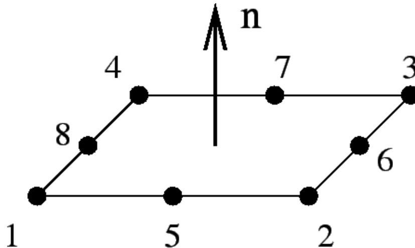
**Figure 4-6 ABAQUS shell element (ABAQUS Documentation, 2013)**
