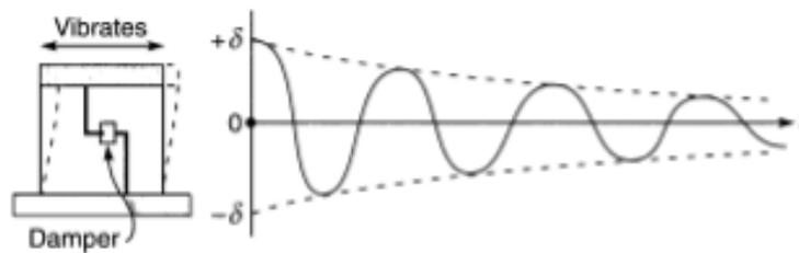
Figure 2-5 Damped free vibrations of a single degree of freedom system (Taranath, 2009; Clough and Penzien, 2013)
