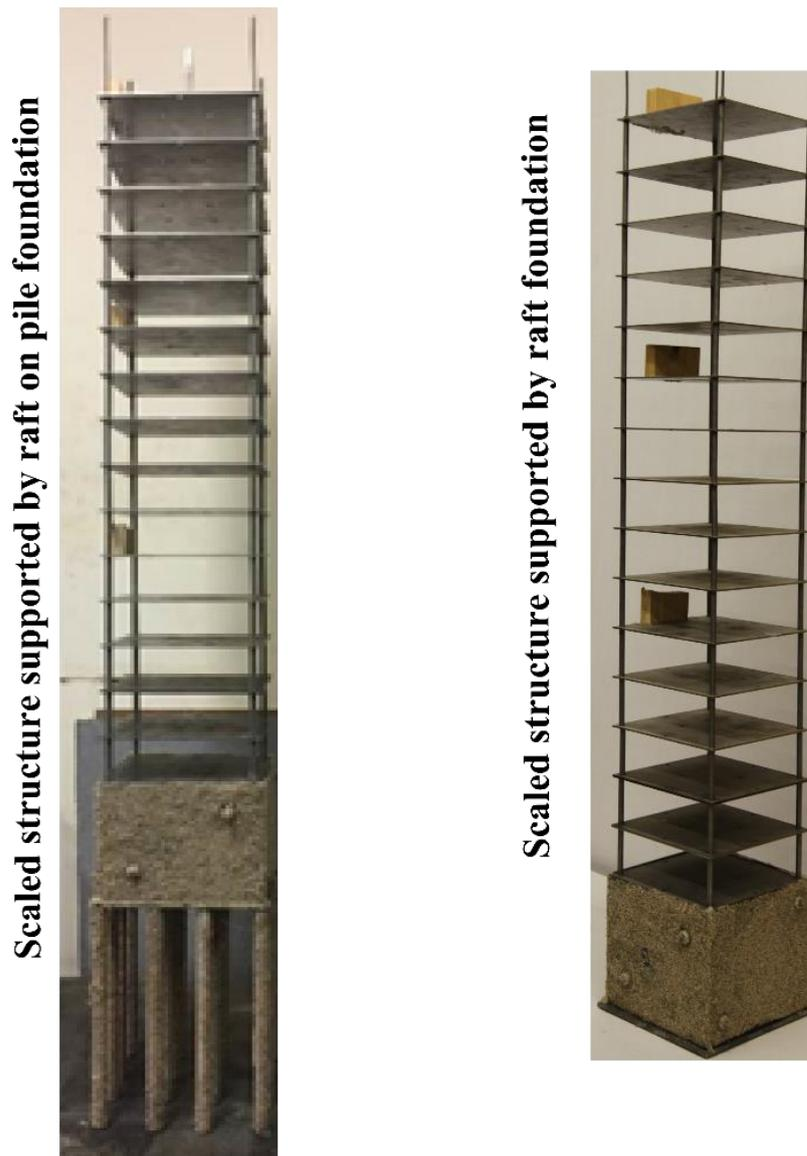
Figure 3-10 Constructed scaled model and foundation types
