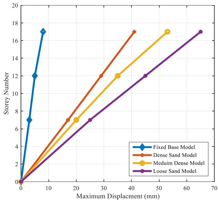
**Figure 6-5 Effect of soil properties on maximum displacement (raft foundation)**
