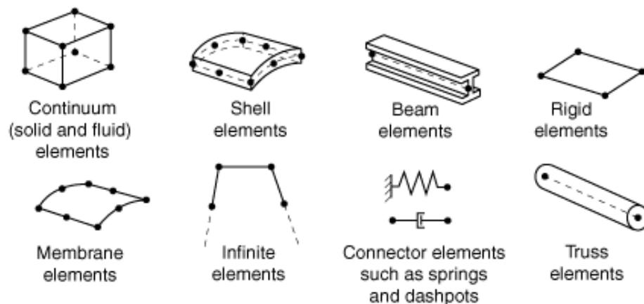
**Figure 4-3 ABAQUS elements (ABAQUS documentation, 2013)**
