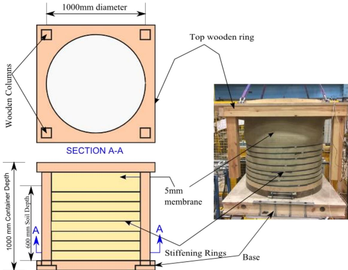
Figure 3-7 The soil container design
