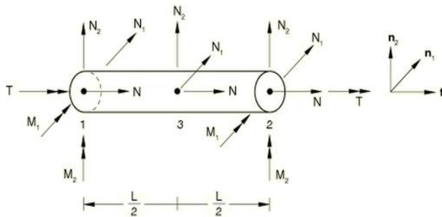
**Figure 4-5 ABAQUS beam element B31 (ABAQUS Documentation, 2013)**
