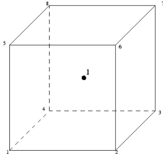
**Figure 4-4 hexahedral C3D8R elements with integration point scheme
