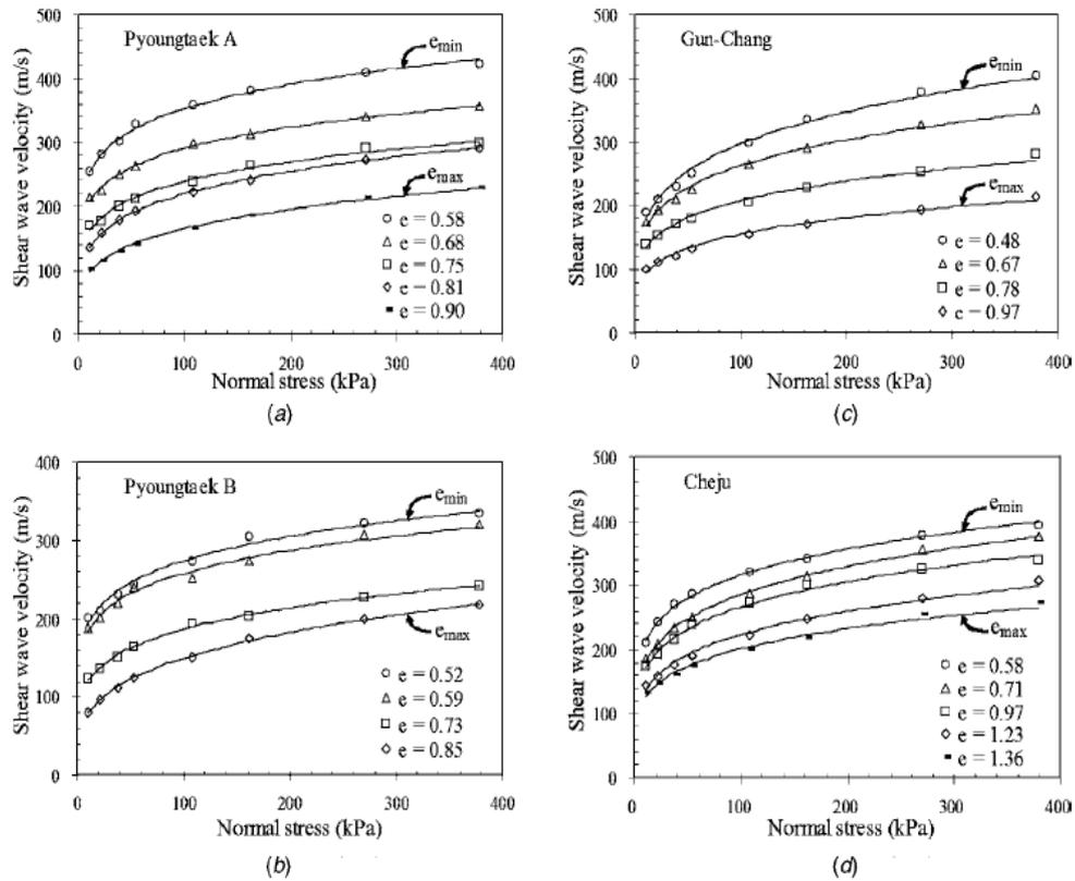
**Figure 2.19 Variations of void ratio versus shear waves velocities after Cha and Cho (2007)**
