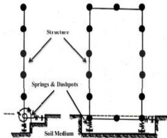
**Figure 2-14 Soil model in lumped parameter methods (Bowles Joseph, 1996)**
