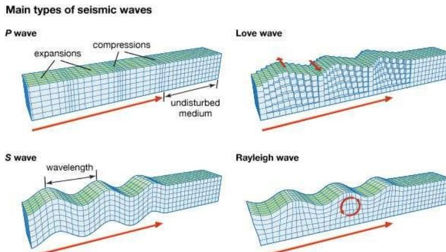
**Figure 2-16 Types of seismic waves (Chowdhury and Dasgupta, 2008)**
