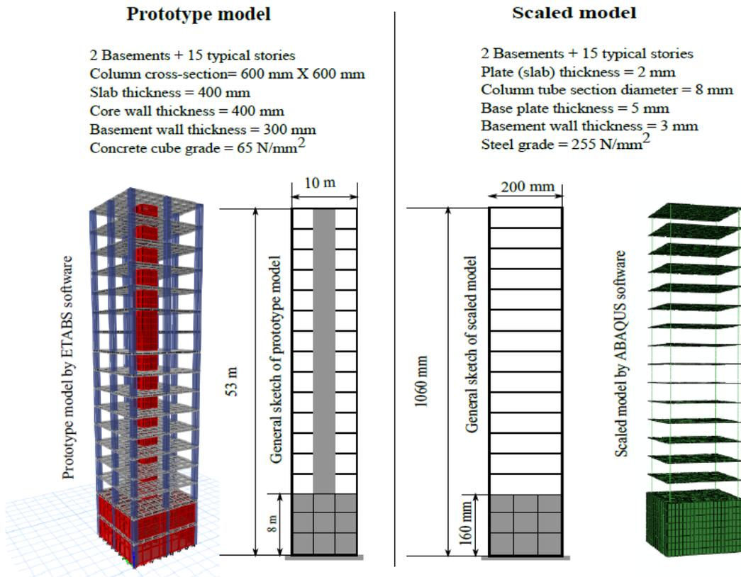
**Figure 5-1 Detail of the prototype and scaled model**
