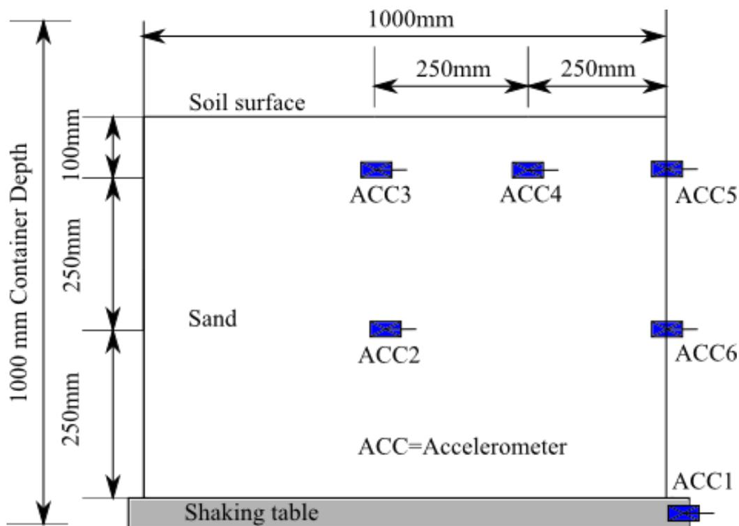
**Figure 3-16 Layout of accelerometers**
