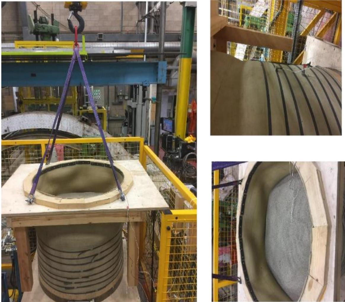
**Figure 3-15 Soil container fixed on shaking table at Salford University**
