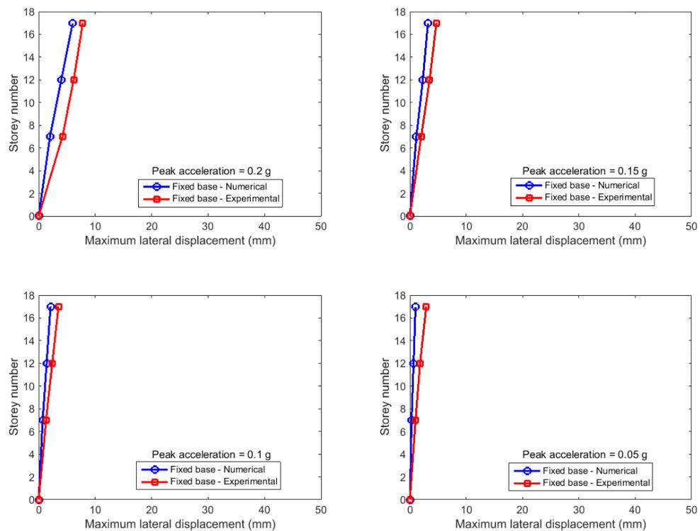
**Figure 5-3 Maximum lateral displacement of experimental and numerical outputs**
