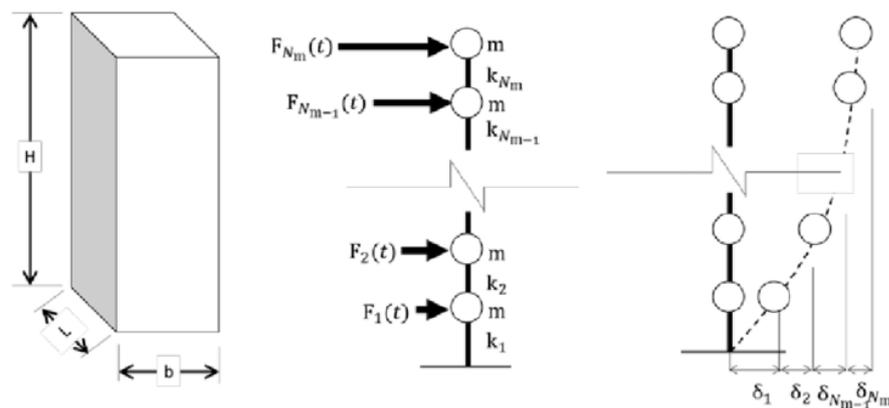
**Figure 3-3 Lumped mass simplification of multi-story buildings (Serrano et al., 2017)**
