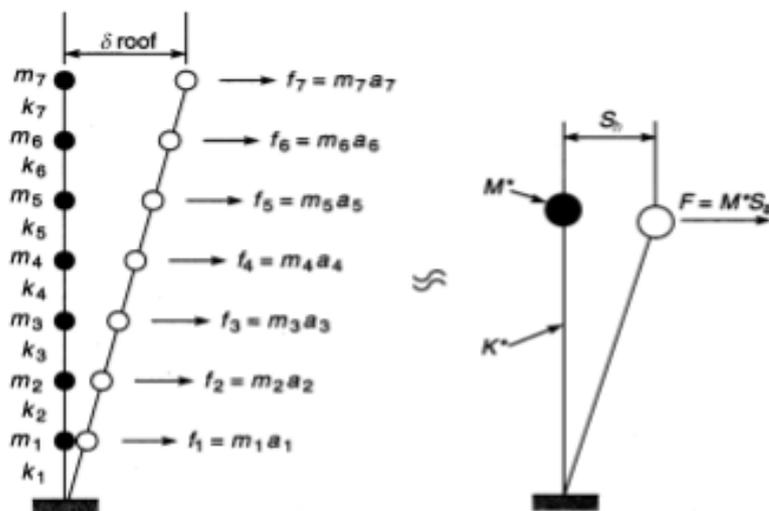
Figure 2-6 Representation of multi-mass system by a single mass system (Taranath, 2009; Clough and Penzien, 2013)
