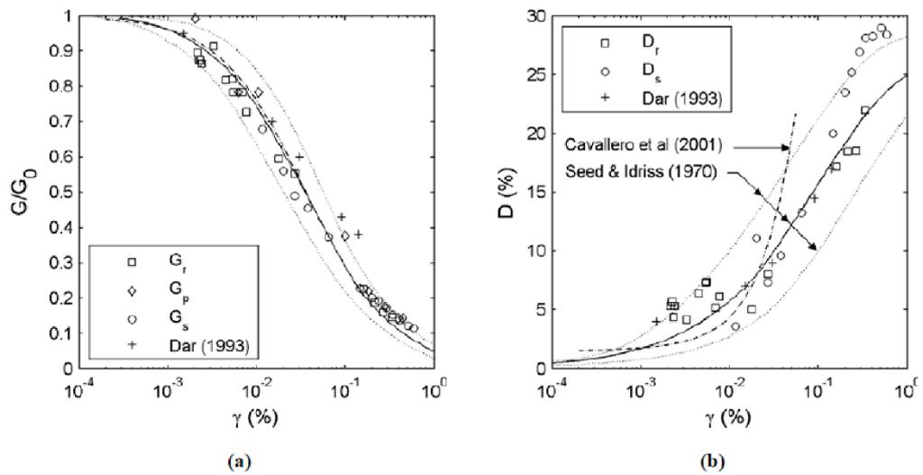
Figure 3-18 (a) The evolution of Shear modulus  $G$  with shear strain  $\gamma$  (b) The evolution of damping Ratio  $D$  with shear strain  $\gamma$  (Seed et al. 1986)
