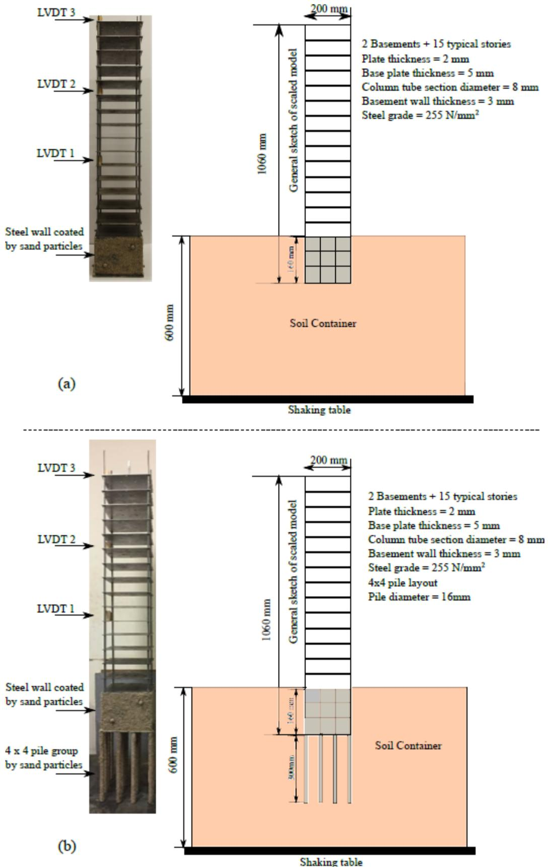
Figure 5-6 Structures supported by (a) raft foundation and (b) raft on pile foundation
