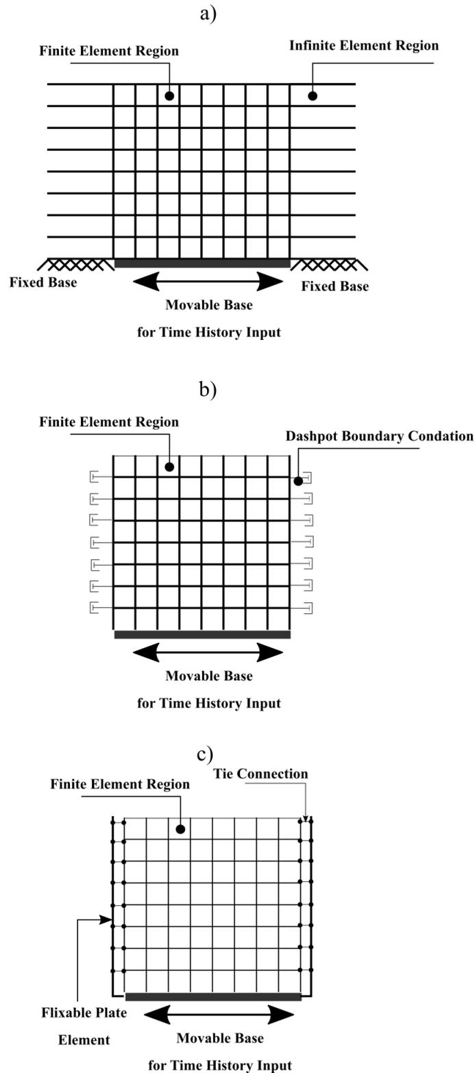
**Figure 4-7 Numerical simulation of the soil boundary condition a) infinite boundary condition, b) dashpot boundary condition c) flexible plate element boundary condition**
