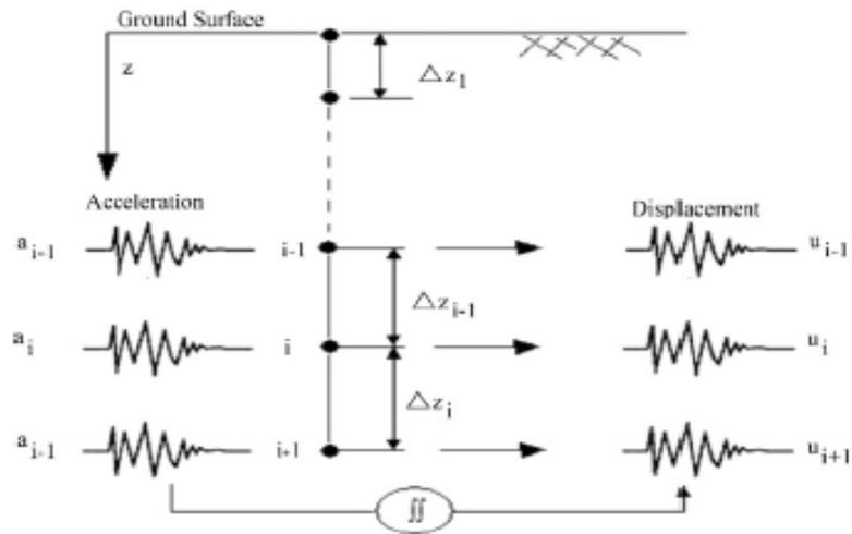
Figure 3-19 The soil response based on acceleration outputs
