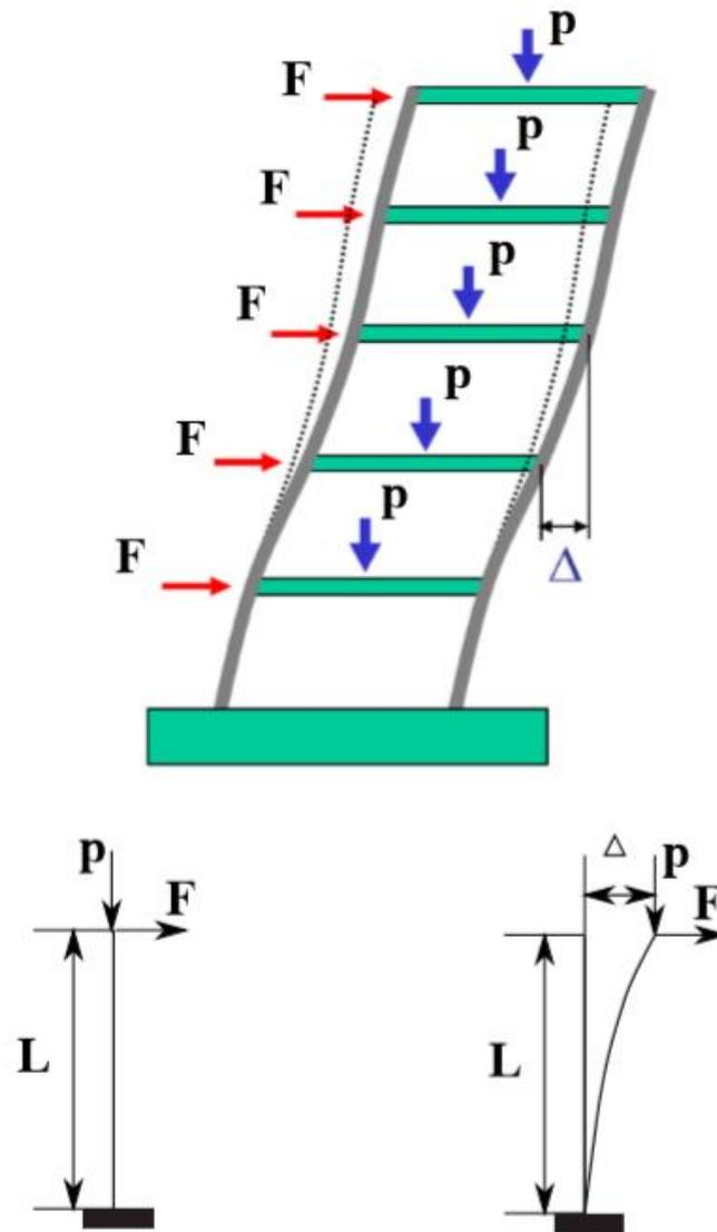
Figure 6-1 Configuration of P- $\Delta$  effect
