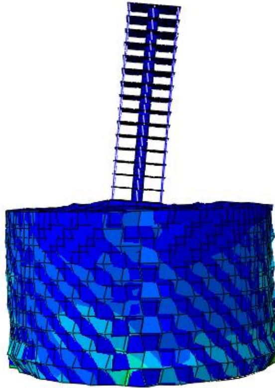
**Figure 6-13 Soil-structure (prototype model) by ABAQUS**
