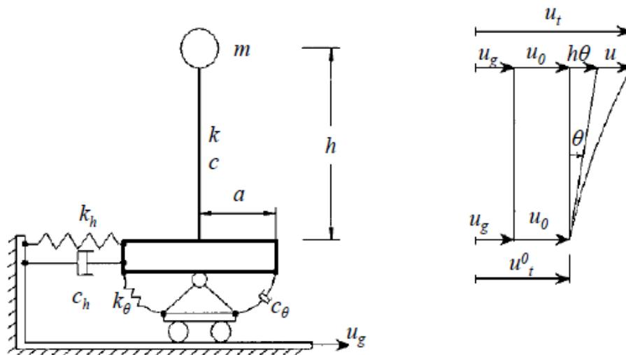
**Figure 2-10 Coupled dynamic model of structure and soil for horizontal and rocking motions proposed by Zhang and Wolf (1998)**
