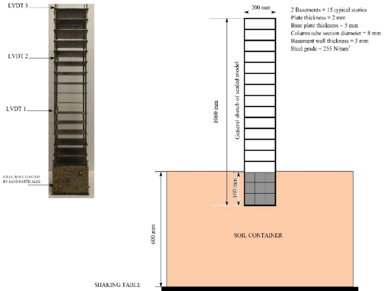
Figure 3-22 Soil foundation structure system details (raft foundation)
