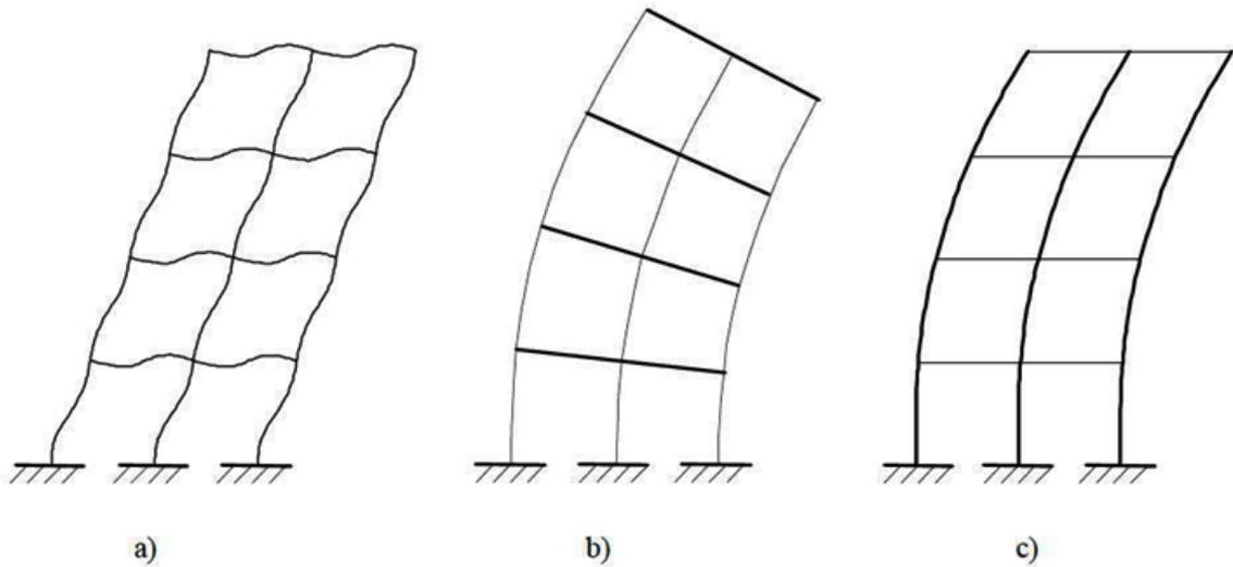
**Figure 4-1 Shear deformation of multi-storey buildings under seismic force (Han and Cathro, 1997)**
