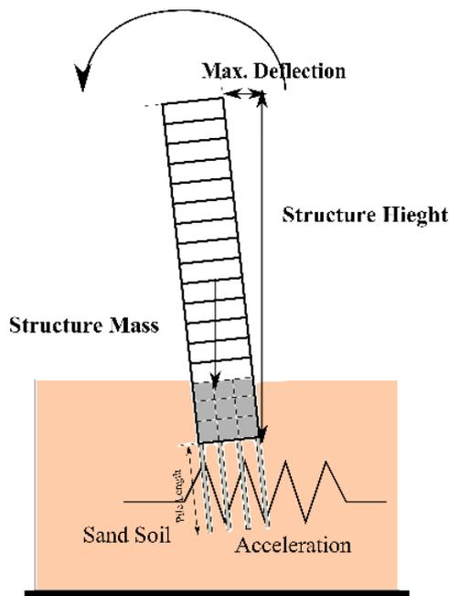
**Figure 6-15 Soil-foundation-structure interaction moment of structure supported by raft-on-pile foundation**
