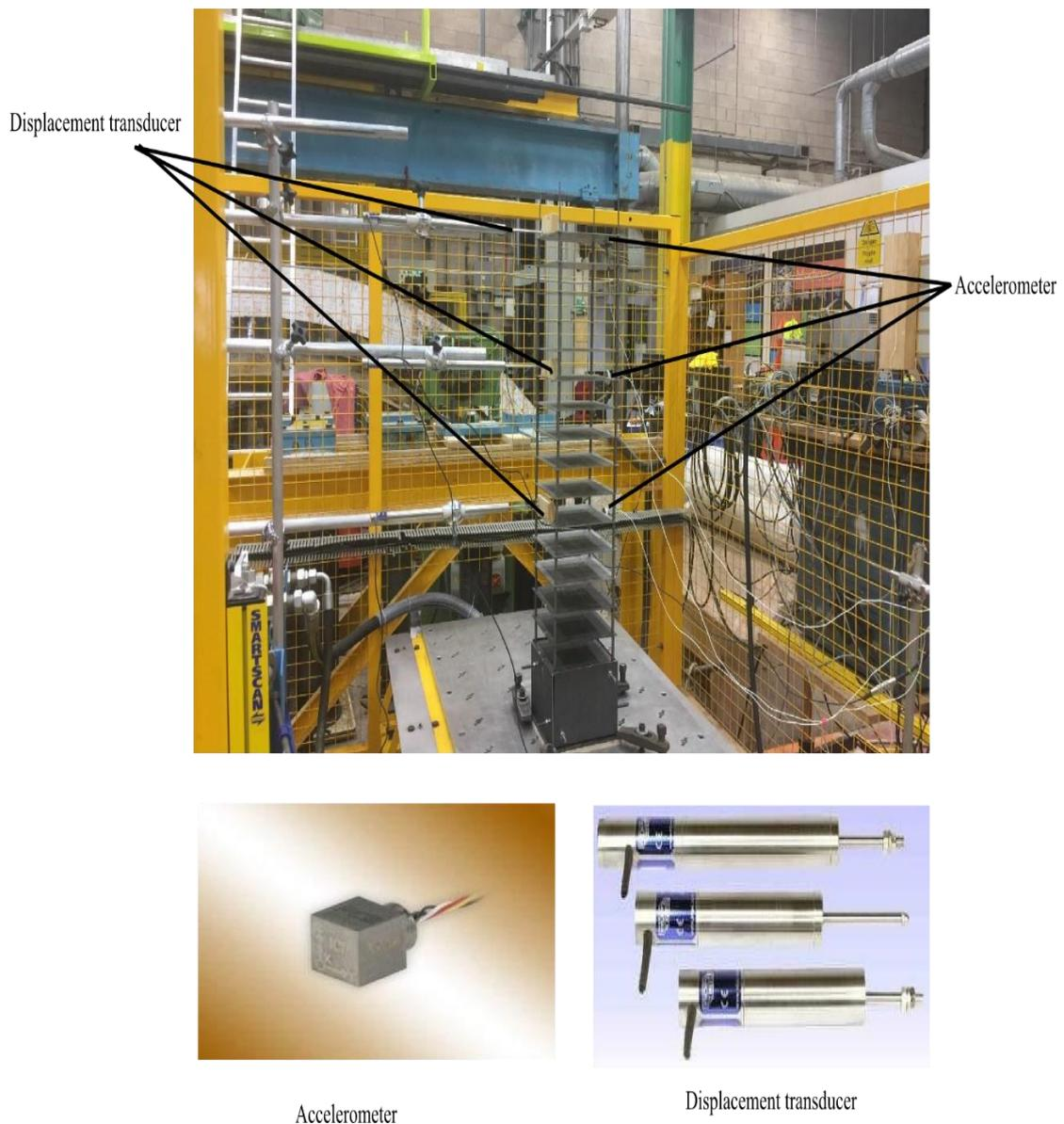
**Figure 3-13 Fixed base shaking table test**
