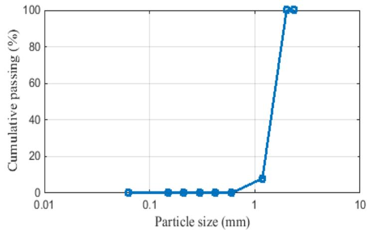
**Figure 3-9 Sieve analysis of selected sand**
