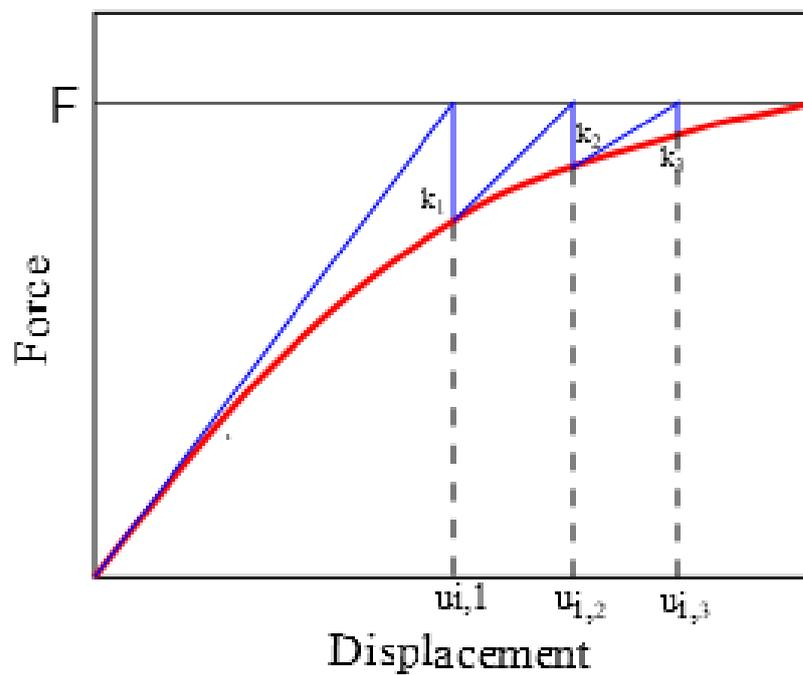
**Figure 4-2 Newton-Raphson iterations used in nonlinear analysis
