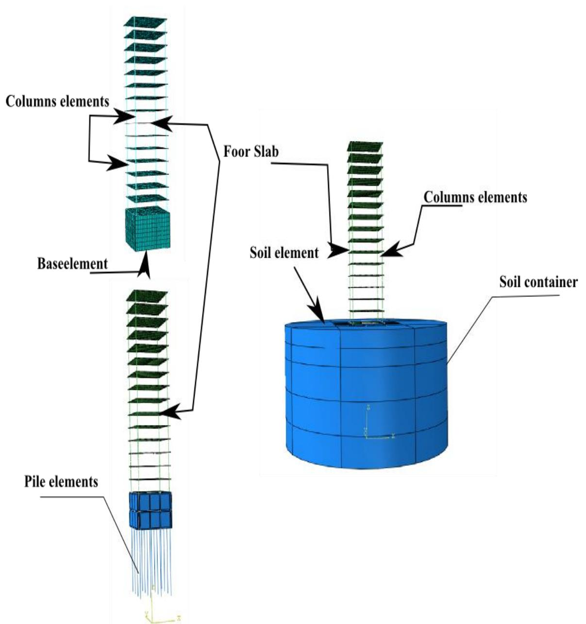
**Figure 4-8 Numerical elements modelled by ABAQUS**
