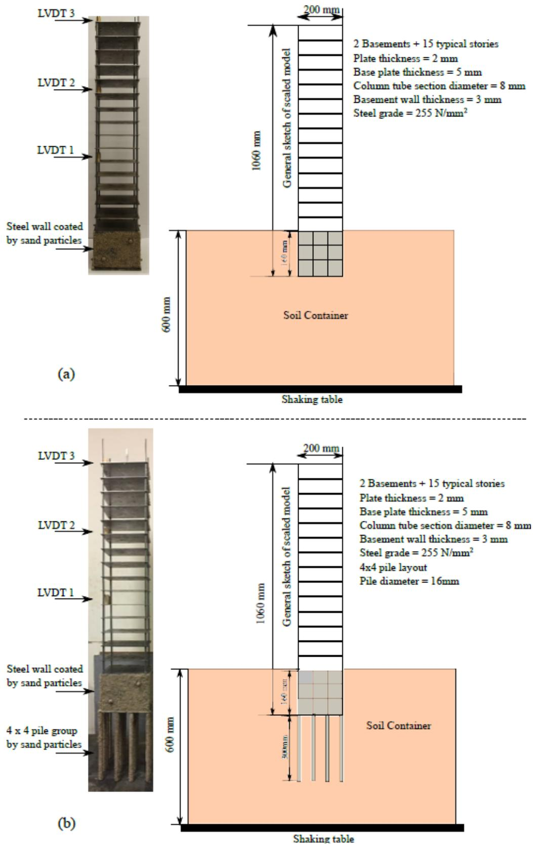
Figure 6-2 Structures supported by (a) raft foundation and (b) raft-on-pile foundation
