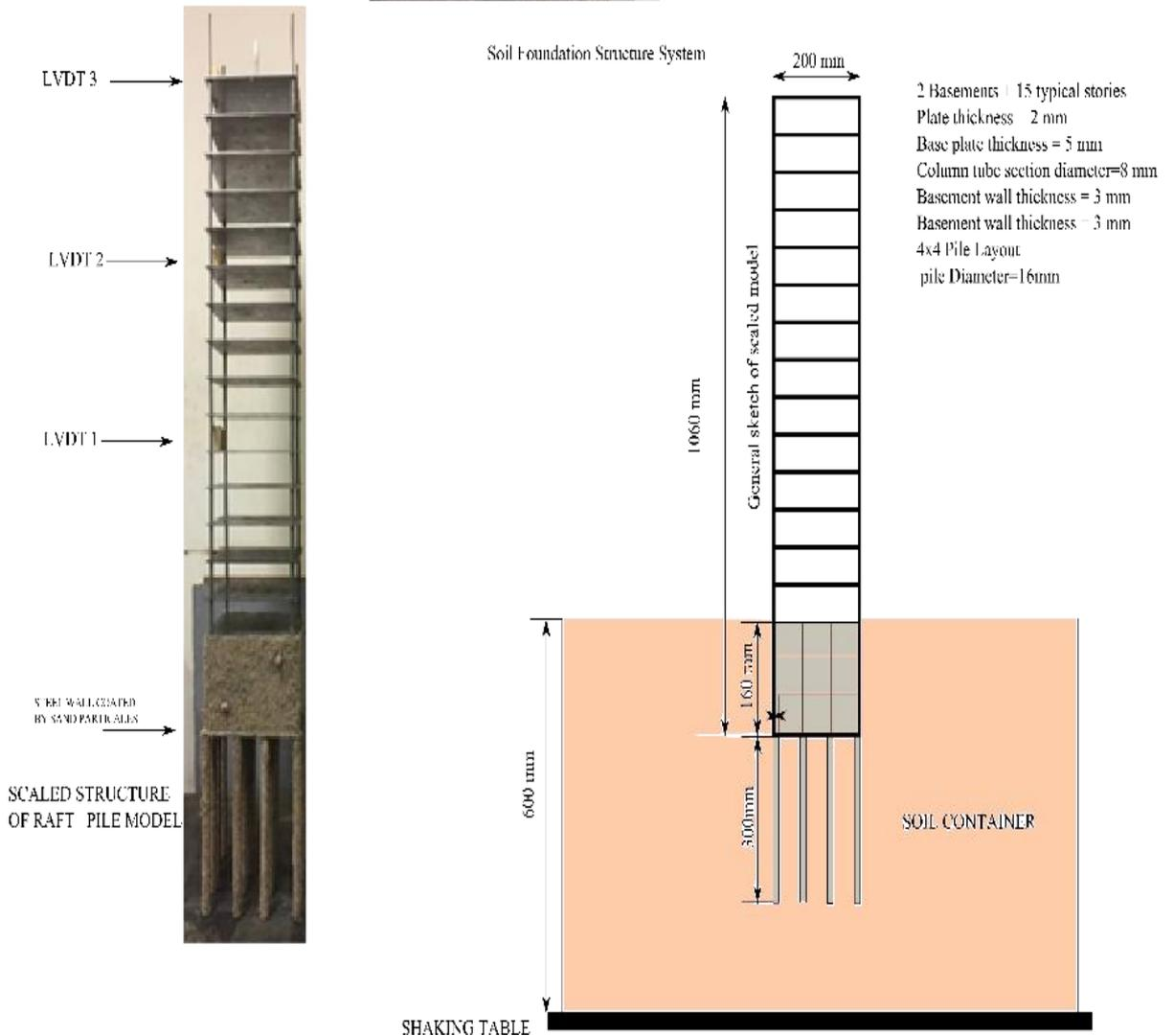
Figure 3-24 Soil foundation structure system details (raft on pile foundation)
