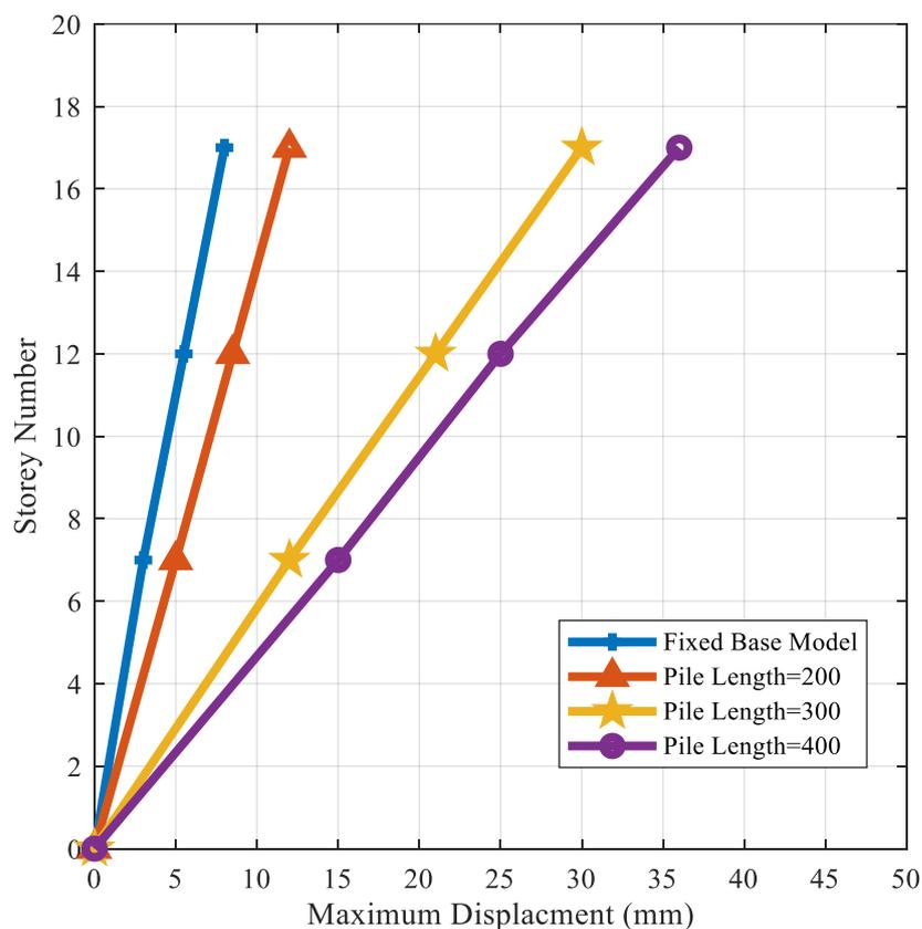
Figure 6-11 Effect of pile length on maximum displacements
