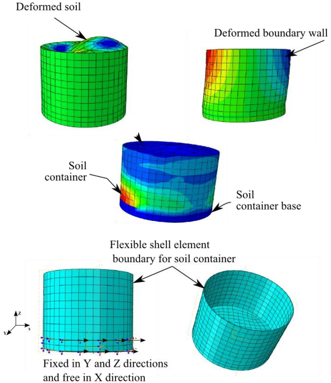
**Figure 4-10 Soil element boundary model by ABAQUS software
