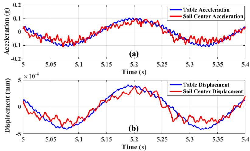
**Figure 3-20 Measurement of time-acceleration and time displacement at the table and soil mass level**
