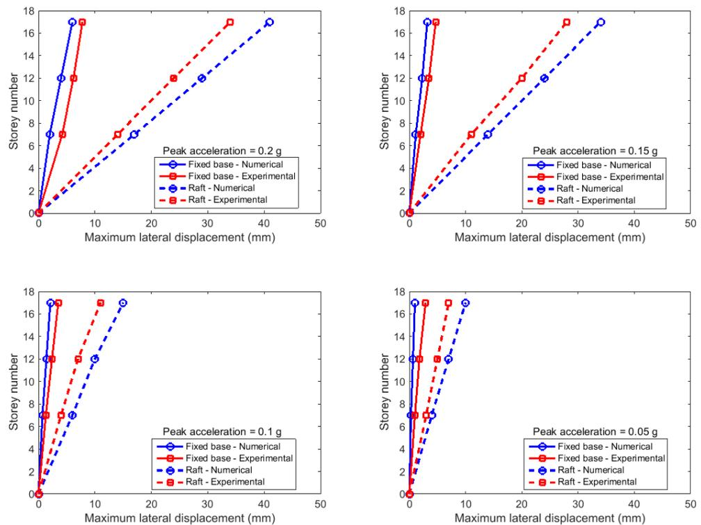
Figure 5-8 Structure on raft foundation output
