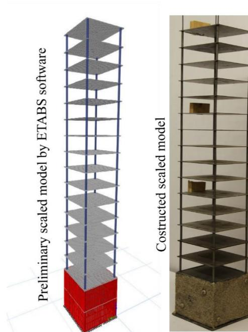
**Figure 3-6 Scaled model design**
