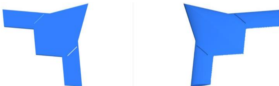
Figure 7.11: Flying wing configurations with optimised chordwise slot: Flat plate model (left); GOE444 aerofoil profile wing (right)
