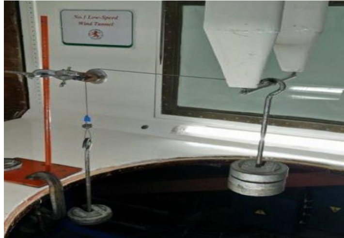
Figure 3.2: Weight applied linearly in order to measure lift and drag
