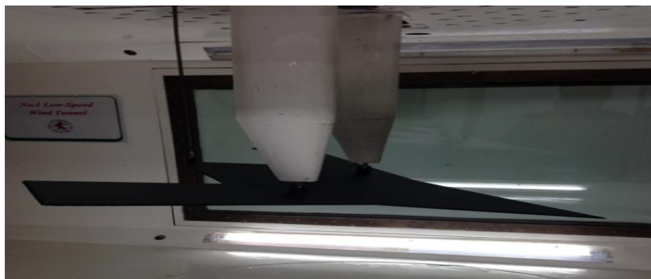
Figure 3.1: Flying wing configuration 2 mounted in low speed wind tunnel
