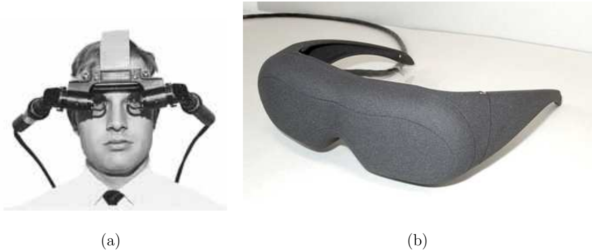
Figure 1.2: (a) 1966: Ivan Sutherland's CRT based HMD (b) Modern day: A typical HMD with stereo capabilities up to 800x600 resolution. Commercially available for approx $5000.
