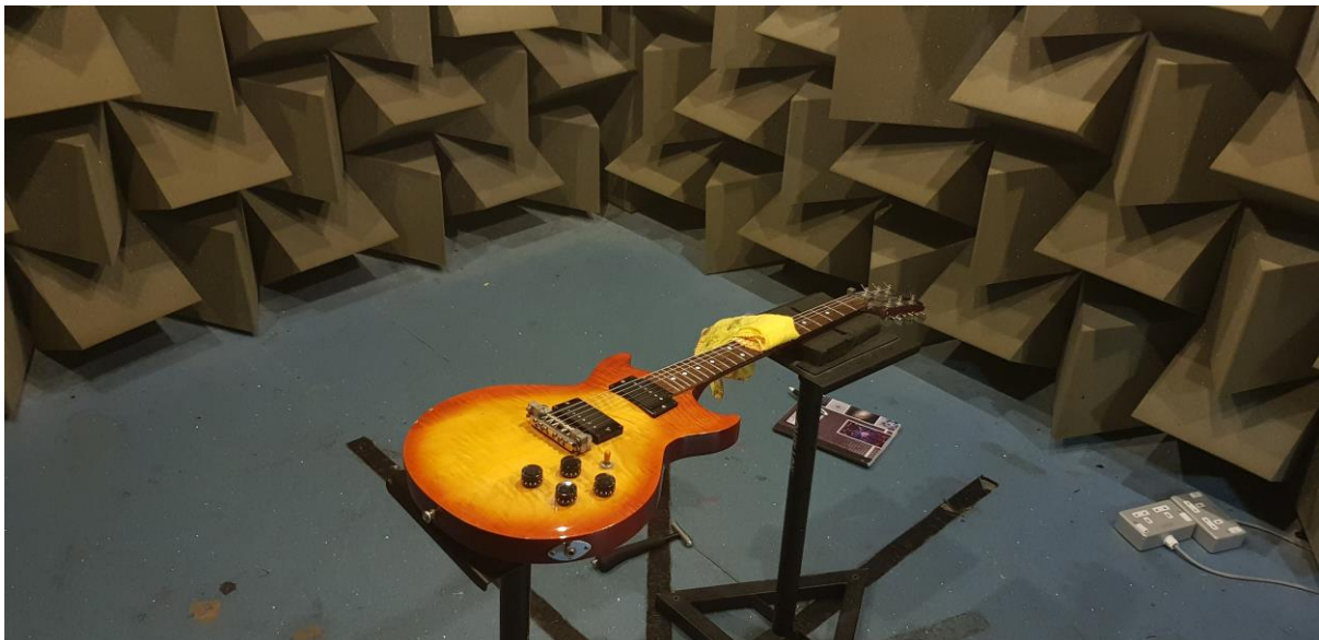
Figure 2 – Gordon Smith Electric guitar in the semi anechoic chamber. One of Two guitars tested.
