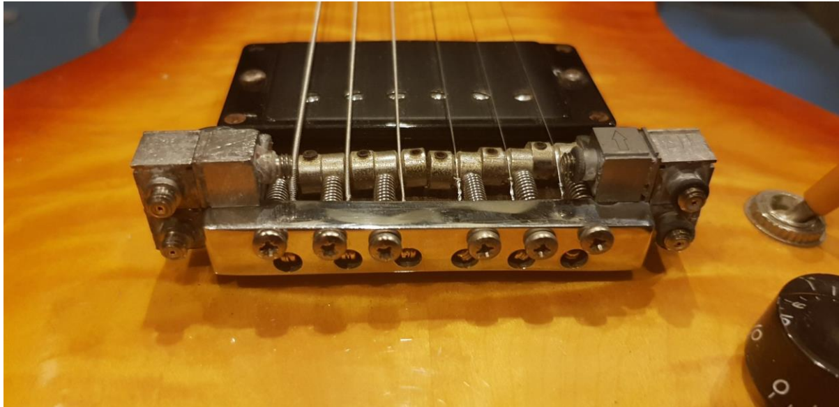
Figure 3 – Gordon Smith Electric guitar instrumented with six single axis accelerometers in order to capture three degrees of freedom of coupling of the guitar bridge screws to the guitar body.
