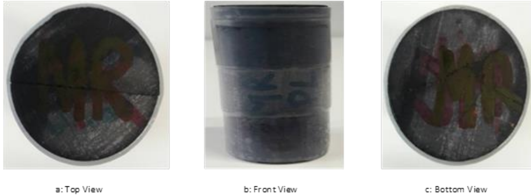
Figure 4-27: Show Marcellus Shale Sample (Fracture 1)
