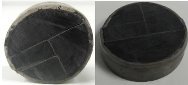
Figure B5: Line Complex Fractured Shale Sample (13.4 mm, L * 37.44 mm, D)
