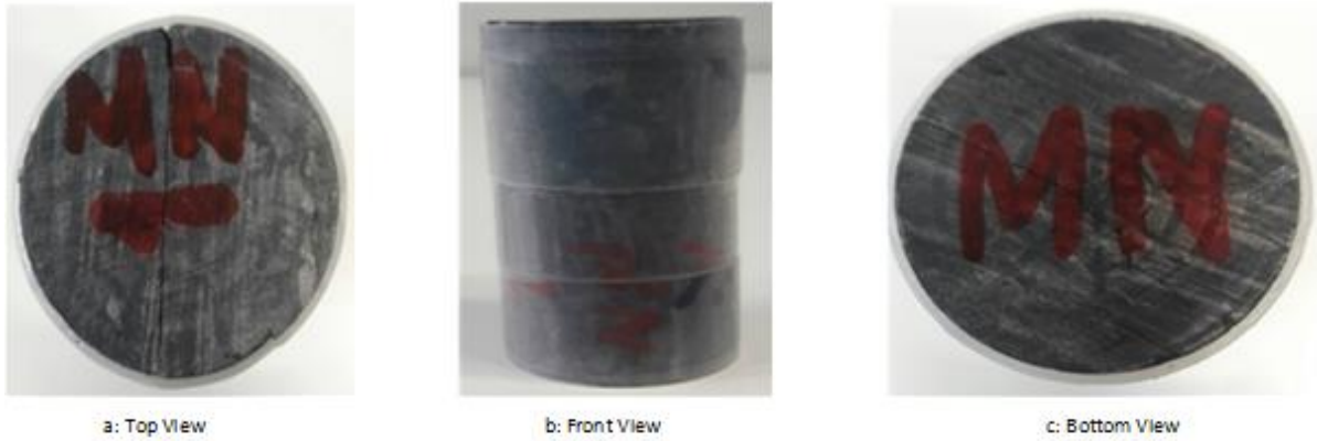
Figure 4-16: Mancos Shale Sample (Fracture 1)
