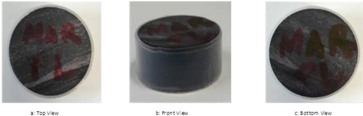
Figure 4-23: Show Marcellus Shale Sample (No Fracture)
