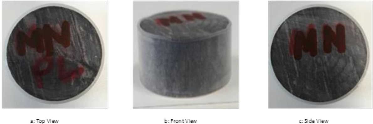
Figure 4-14: Show Mancos Shale Sample (No Fracture)
