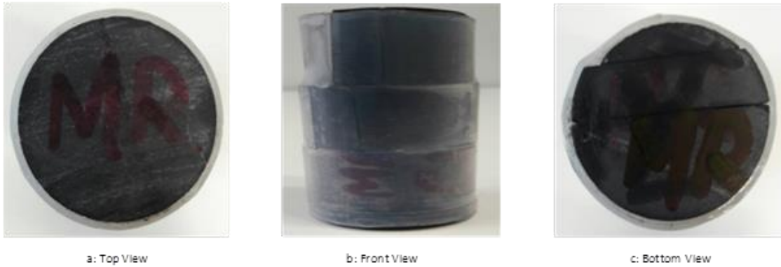
Figure 4-29: Show Marcellus Shale Sample (Fracture 2)
