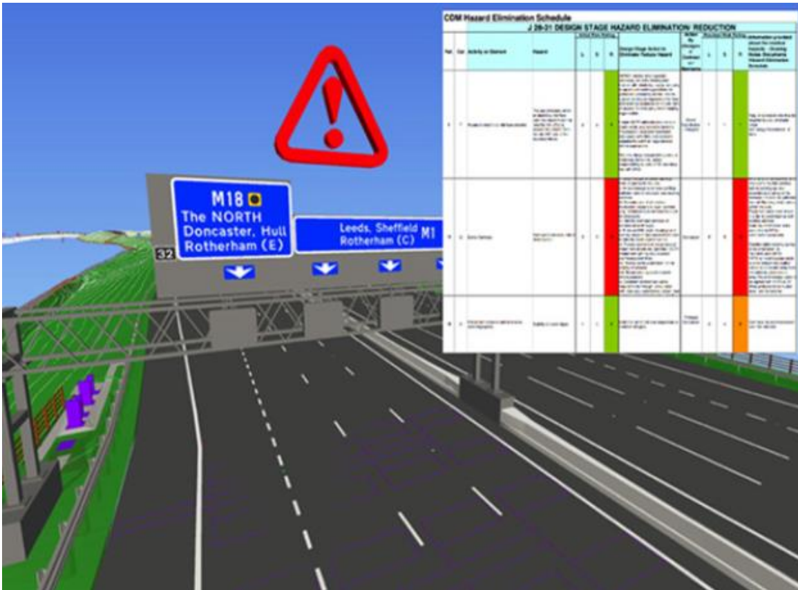
Figure 4.12: Screenshot of capturing as-built records including residual hazards within the BIM model to aid future maintenance operations
