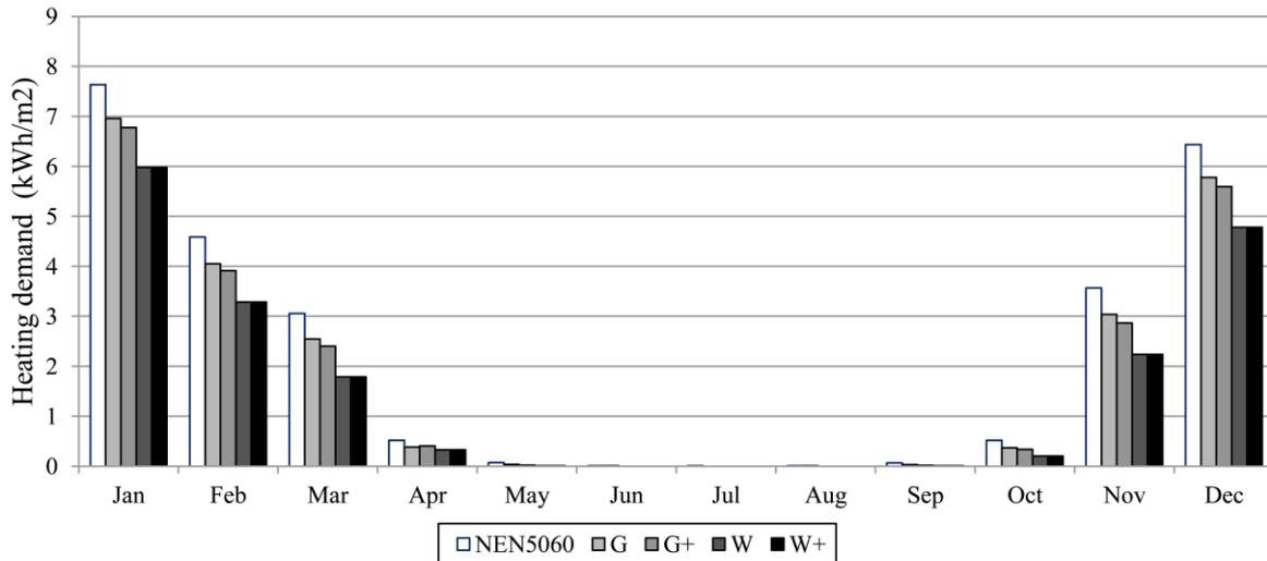
Figure 12: Heating energy demand of Building I based on [45] and the four KNMI'06 climate scenarios.
