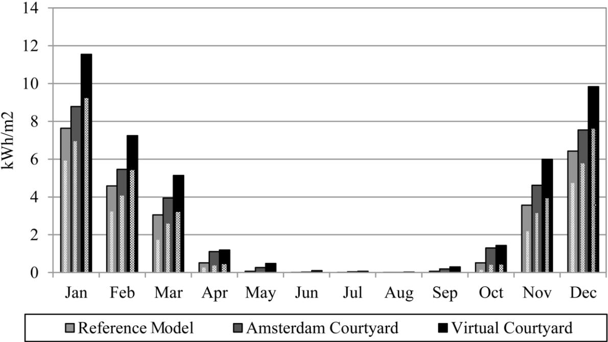
Figure 13: Heating energy demand of Building I, IIC and IIIc for the current climate of the Netherlands (dark bars) and the future W+ scenario (white bars inside dark ones).
