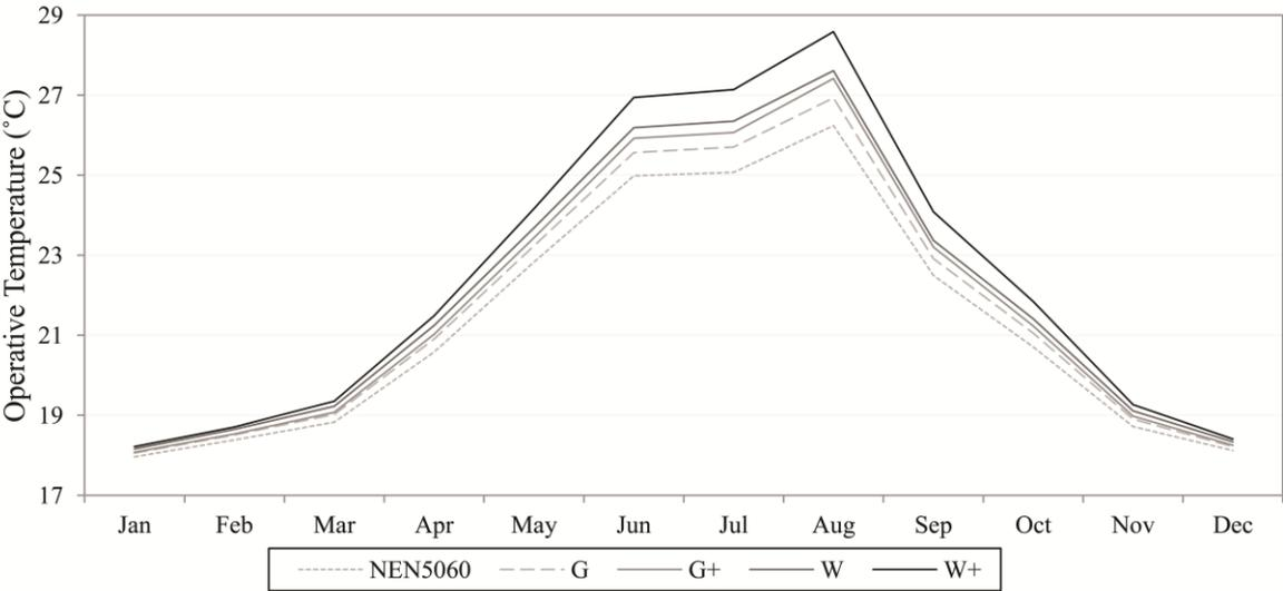
Figure 11: Monthly average Indoor operative temperature of Building I versus outside dry bulb temperature based on [45] and the four KNMI'06 climate scenarios.
