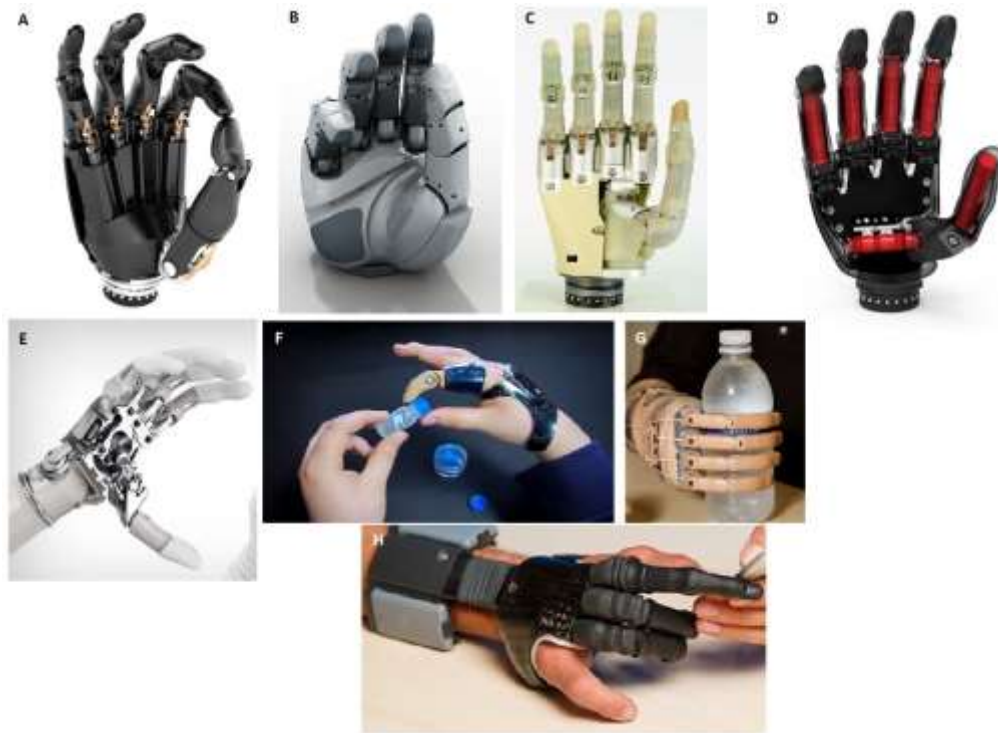
Figure 2.1. Commercial robotic hands for prosthetics and other uses
