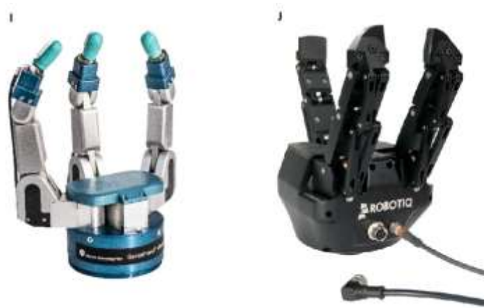
Figure 2.1. Commercial robotic hands for prosthetics and other uses
