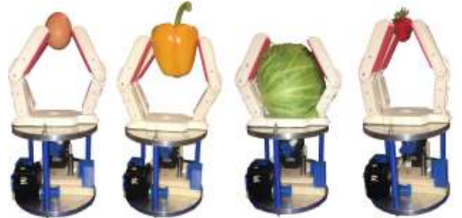
FIGURE 10. VSH 1 with three finger can grasp different objects with different sizes and flexibilities thanks to its variable stiffness mechanism.
