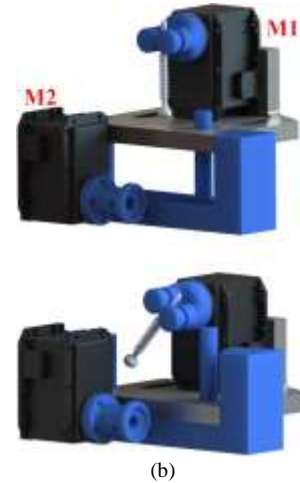
FIGURE 3. (a) A CAD model and (b) a schematic representation of our VSH 1 . Our design consists of two rotational electric actuators M 1 and M 2 . One of the servos, M 1 , provides rotational motion \theta , whilst the second is used to produce a linear displacement, \Delta B , along the wrist axis of the gripper.
