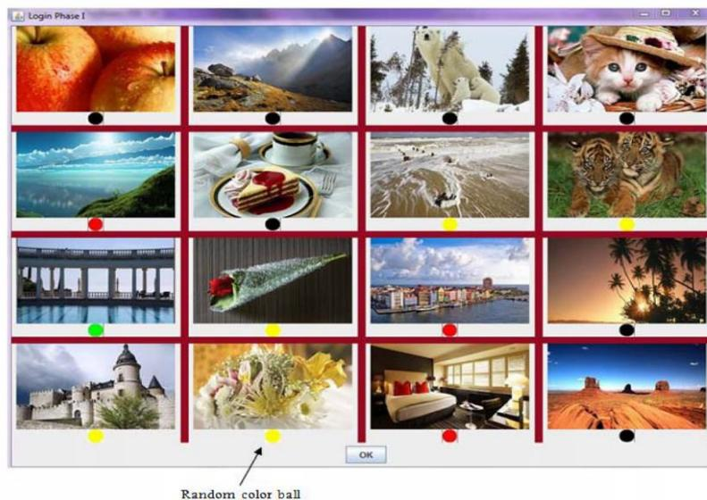
Fig. 2.15: The first authentication phase, 4x4 grid and associated colour balls
