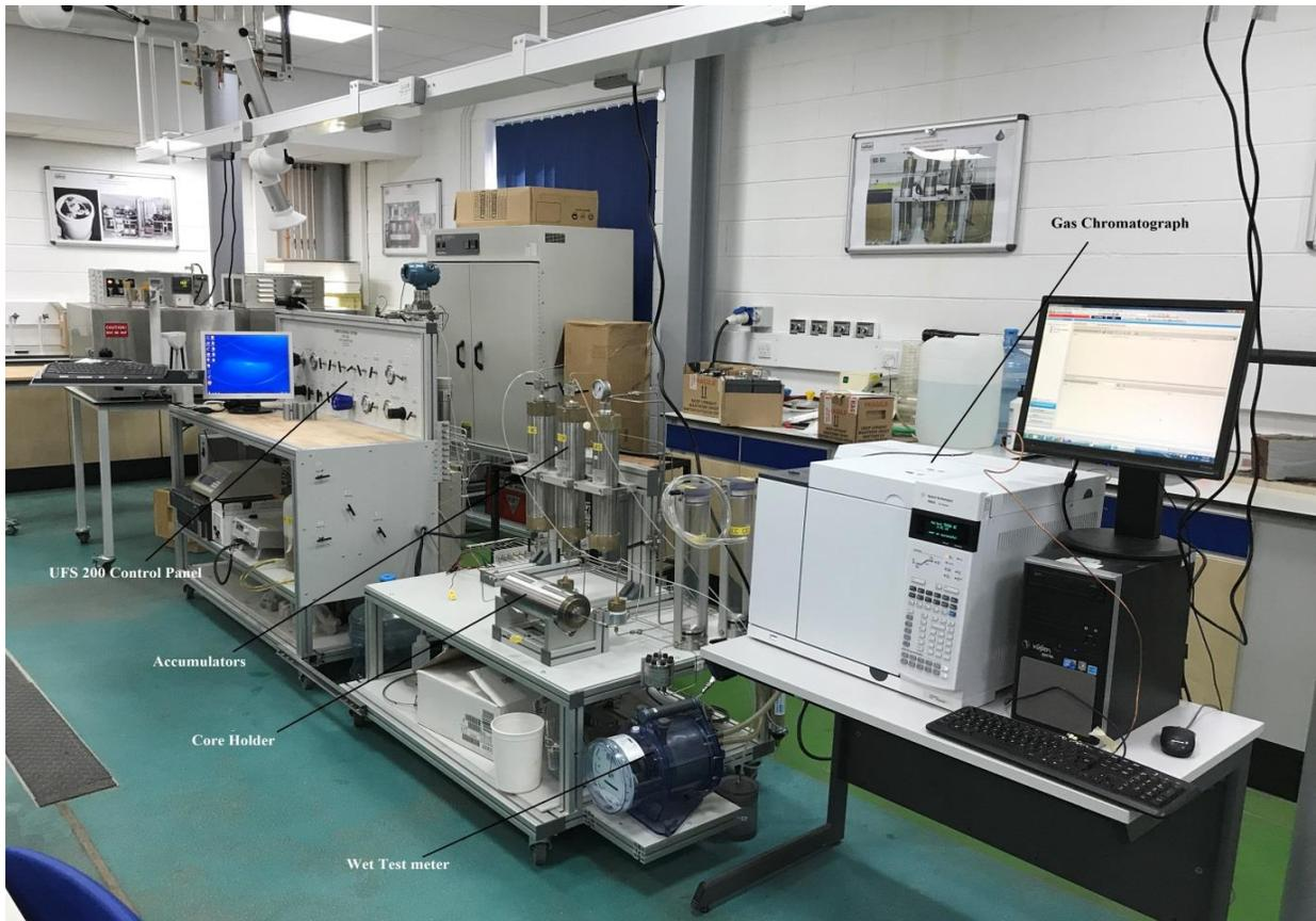
*Figure 3: A perspective depiction of the core flooding setup and the gas chromatograph*
