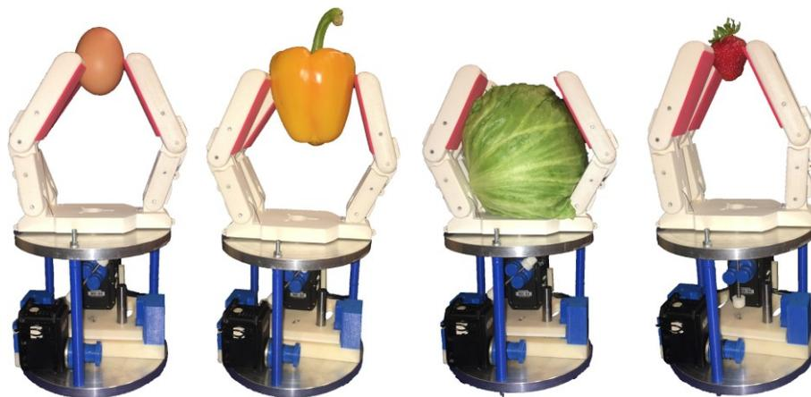
Figure 3.21: Different objects with different sizes and flexibilities lifted by VSG<sub>2</sub>.
