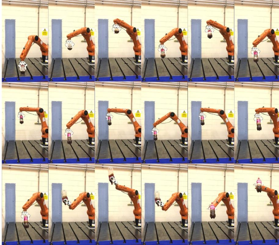
Figure 5.23: The robot grasps and lifts different objects (a Coca-Cola bottle) and starts to move along a pre-programmed trajectory in an accelerating and decelerating manner.
