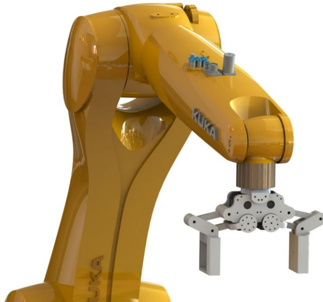
Figure 4.1: The two-finger gripper mounted on the KUKA robot.
