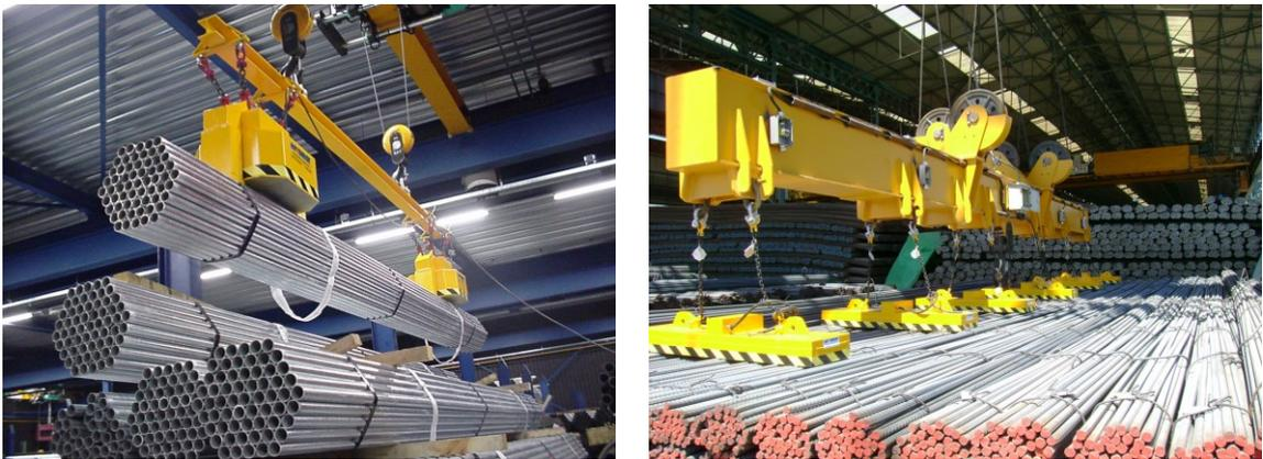
Figure 1.20: Electromagnet grippers provide a simple and low-cost solution for lifting ferrous materials (170).
