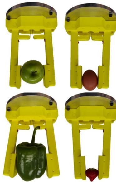
Figure 3.7: Different objects with different sizes and stiffnesses, as lifted by the VSG.
