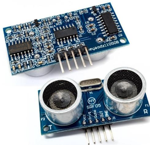
Figure 5.9: Front and back view of the ultrasonic sensor used in the 45 kg payload gripper.
