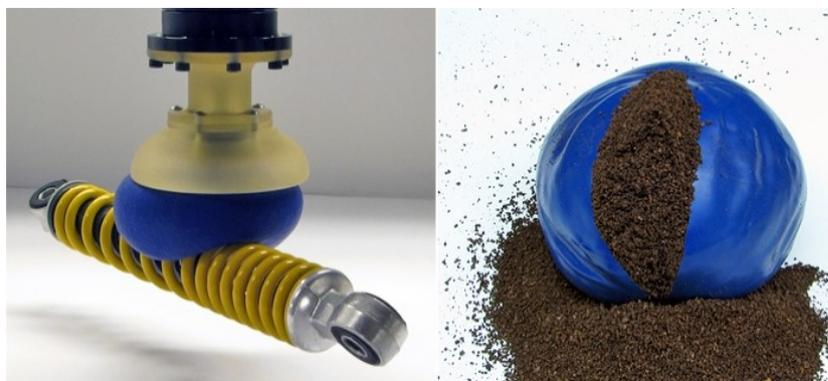
Figure 1.10: The granular jamming universal gripper proposed by Brown et al. (163).
