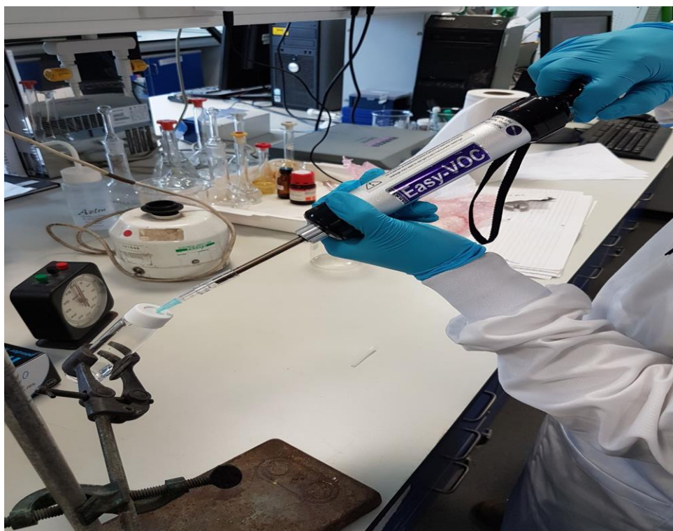
Figure 2.2: Sampling of headspace by using Easy-VOC
