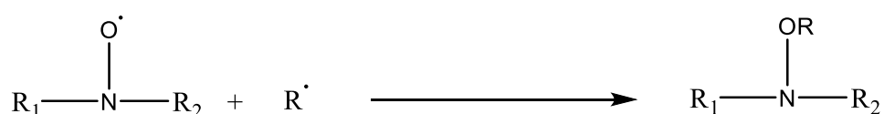
Scheme 1.13: Trapping of radical by nitroxide and formation of the stable radical adduct
