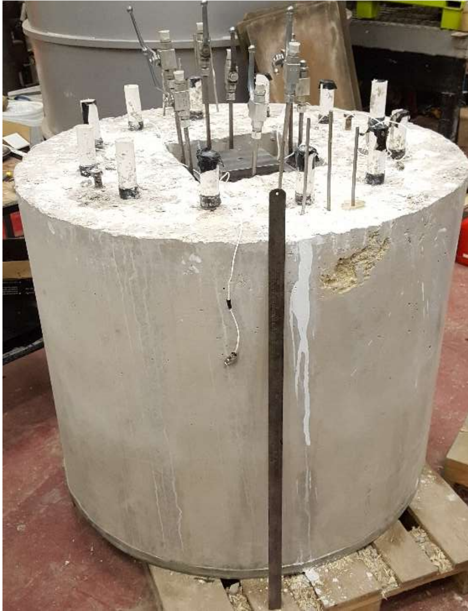
FIGURE 4-1: Concrete reservoir pressure simulator.
