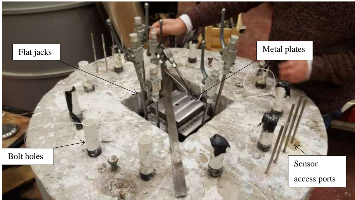
FIGURE 4-22: Sample placed for acoustic confidence testing, this time with the top metal plate attached.
