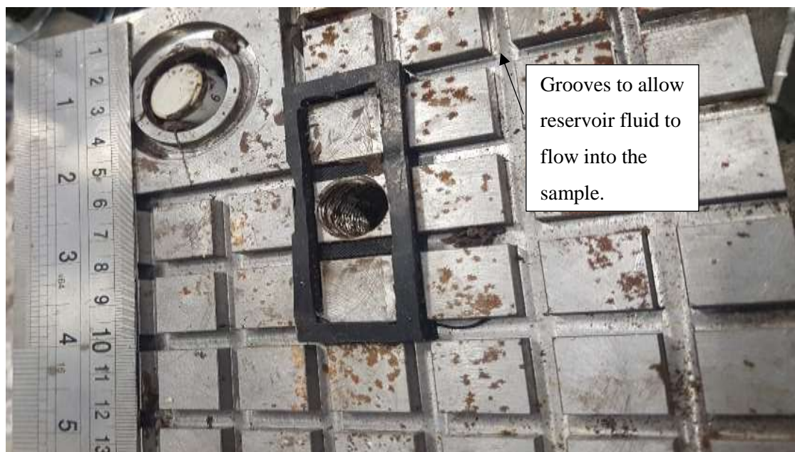
FIGURE 4-30: Plastic packer and rubber seal placed on the metal plate.
