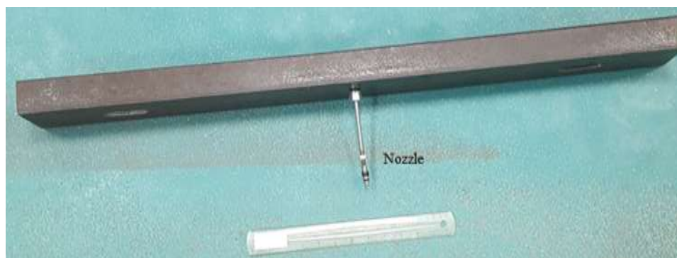
FIGURE 4-27: Fluid injection system set up.
