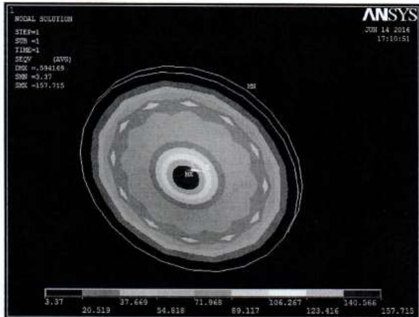
Figure 3: FE Model of End Plates with 12 No HSFG bolts
