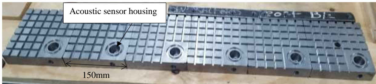
FIGURE 4-3: Metal plates and bulkheads as originally built.
