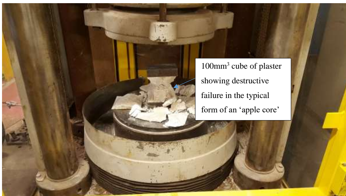
FIGURE 4-18: Apple core failure of the high strength plaster.
