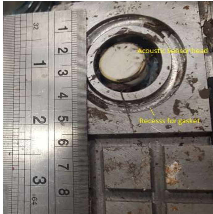
FIGURE 4-23: Acoustic sensor fitted in to the metal plate.
