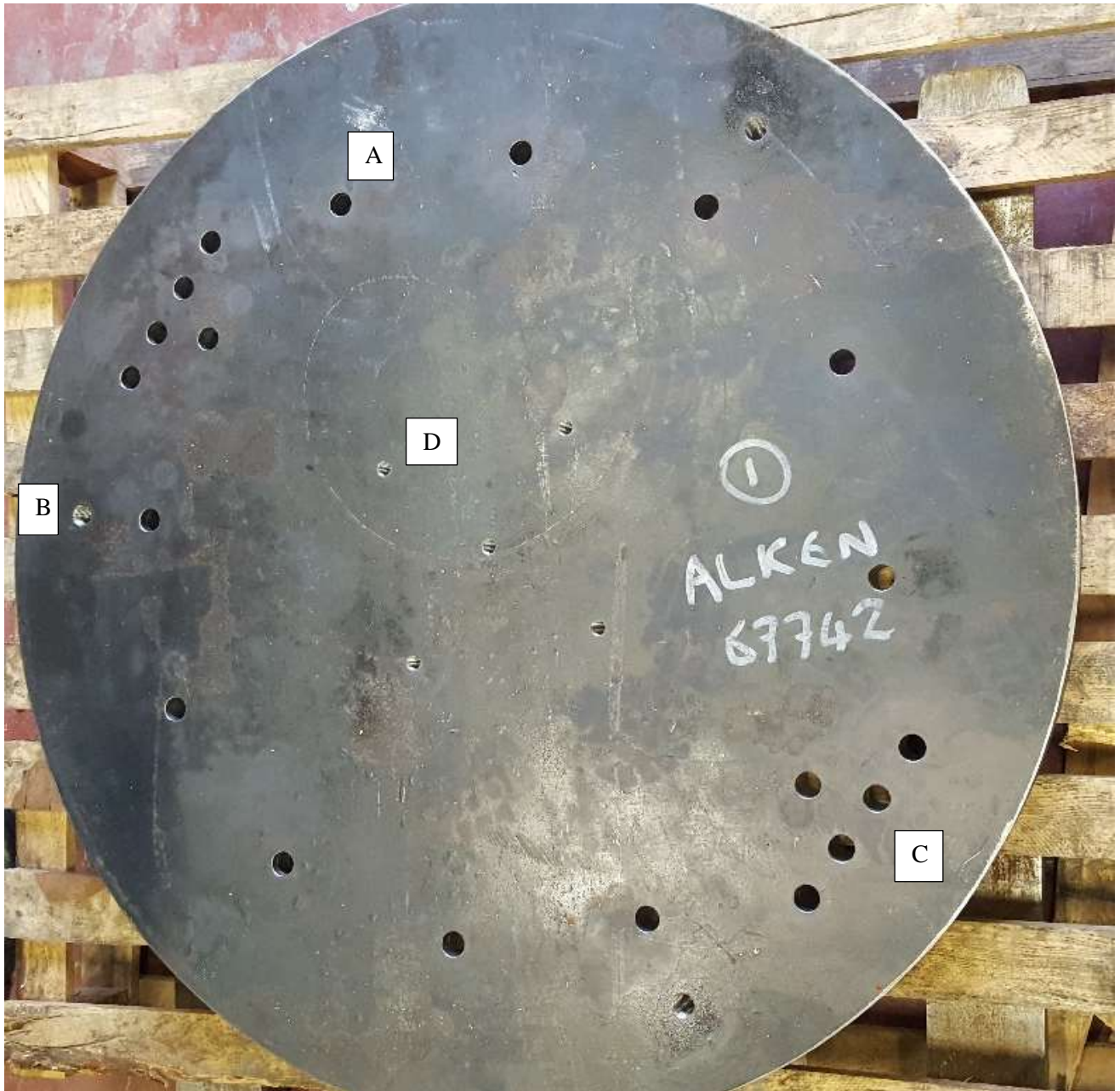
FIGURE 4-2: Top plate. A) M20 bolt holes. B) 20mm lifting eyes. C) Acoustic sensor entry port. D) Service points.
