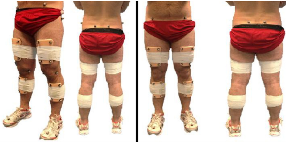
Figure 4.5 Static Trial Marker (Left) Tracking Markers (Right)
