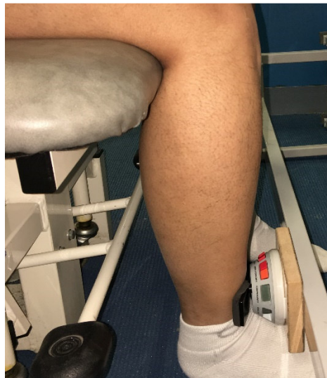
Figure 4.16 Isometric strength assessment of knee extensors with HHD
