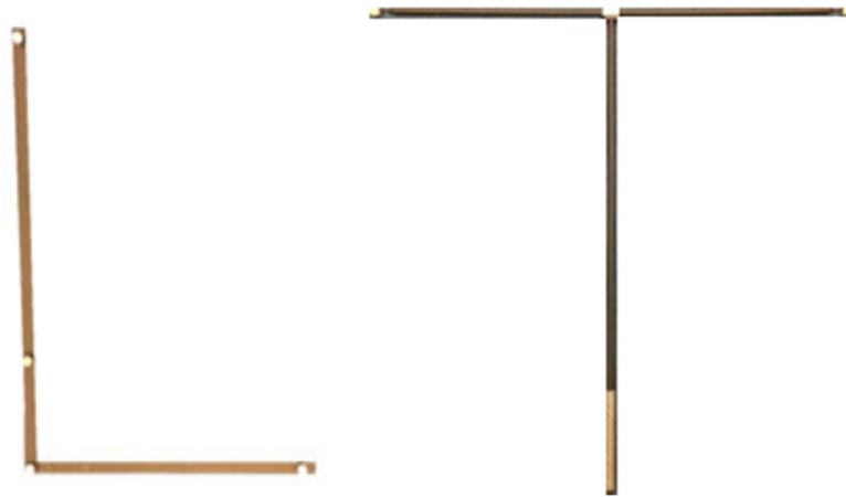
Figure 4.4 Calibration L-shaped frame (Left) and T-shaped handheld wand (right)
