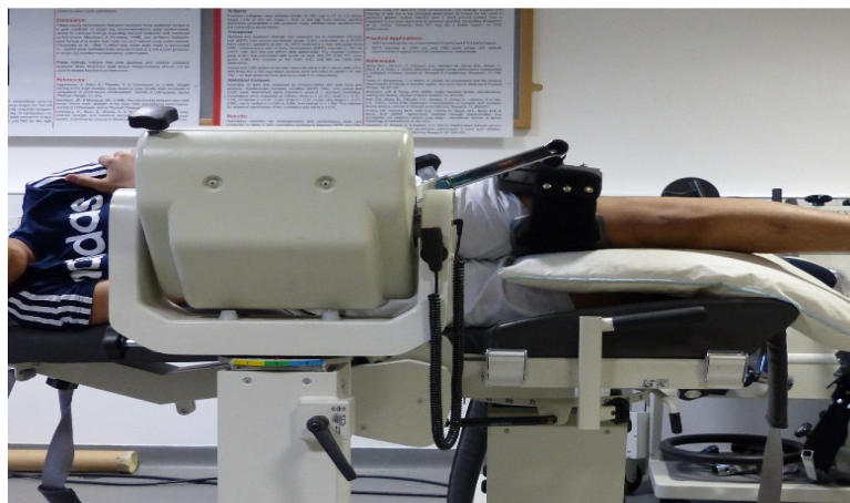
Figure 4.19 Isometric strength assessment of hip abductors with Biodex
