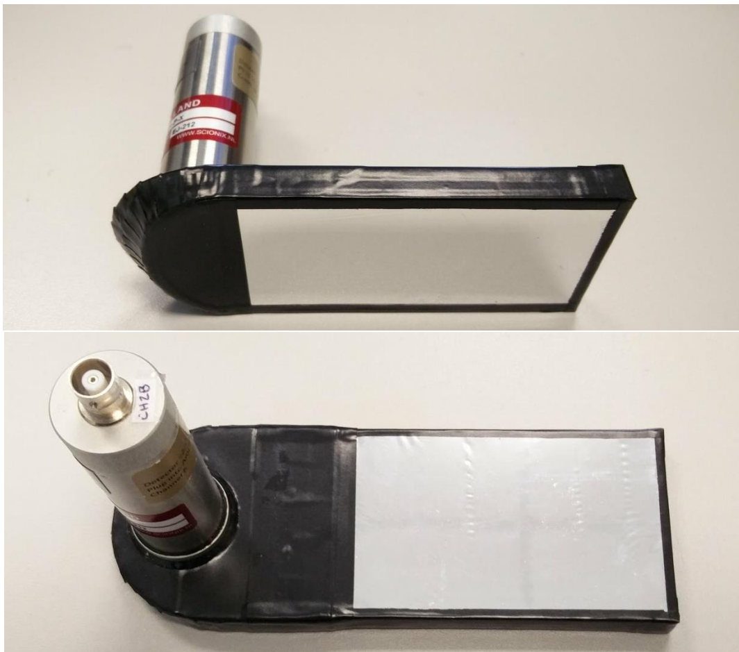
Figure 6.16: The two beta scintillators. Top: the upper beta scintillator with the detection surface visible as the silver rectangle on the lower surface. Bottom: the lower beta scintillator with the detection surface visible as the silver rectangle on the upper surface.
