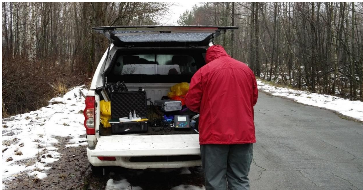
Figure 7.13: Roadside test site. The detector was positioned inside the transport vehicle with access provided through the tailgate.
