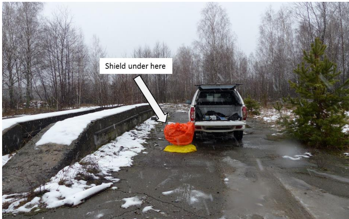
Figure 7.12: Vehicle inspection ramp test site. The detector was positioned under a folding table next to the tailgate of the transport vehicle. An emergency tent was used to cover the table.
