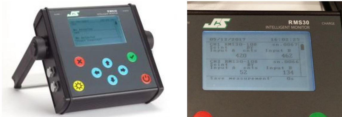
Figure 6.17: The RMS30 unit from JCS. Left, visible are the two scintillator inputs to the left side of the unit. Power and computer connections are available (not shown) on the right side. Right, display on the RMS30 showing all four inputs active. The top two rows display the counts for the gamma scintillators and the bottom row for the beta scintillators.
