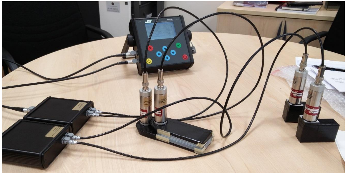
Figure 6.32: Partial assembly of the detection system. The four scintillators connected to the RMS30 via the interface boxes.
