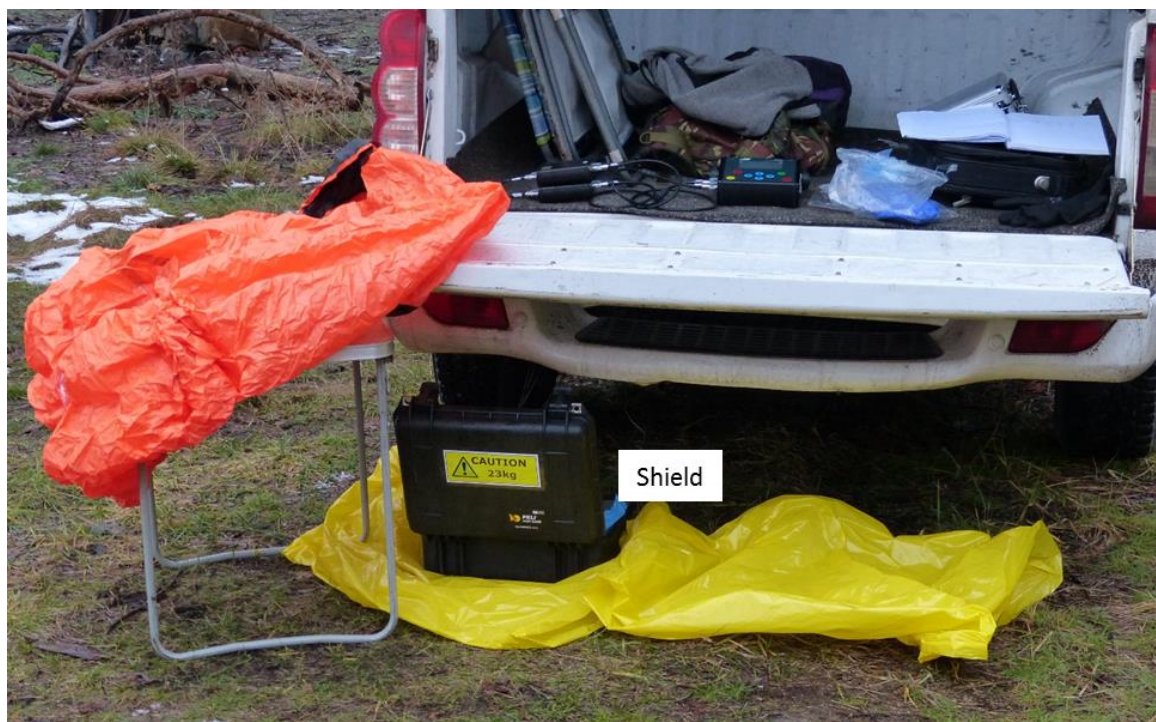
Figure 7.11: Car park test site. The detector shield was located under the tailgate of the transport vehicle due to adverse weather.
