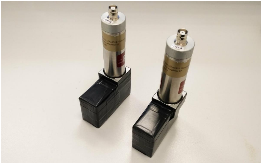
Figure 6.15: The two CsI gamma scintillators. The detection material is wrapped within the black tape.
