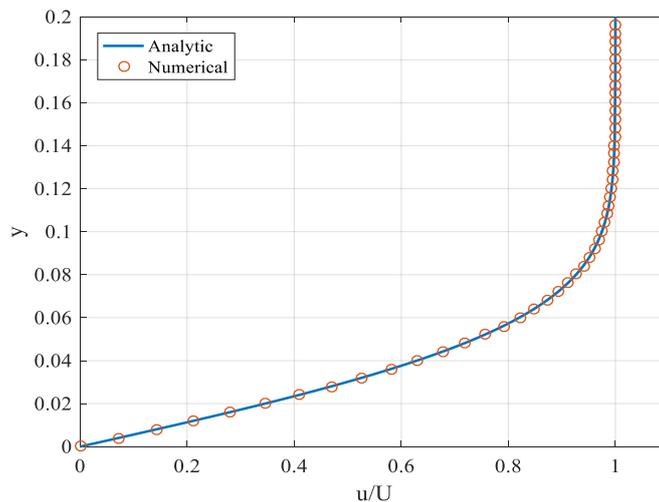
**Figure 8.7** The  $x$ -momentum velocity  $u/U$  with  $y$ -axis of analytic and numerical solution of the Oseen-Blasius equation at  $x = 1$ .
