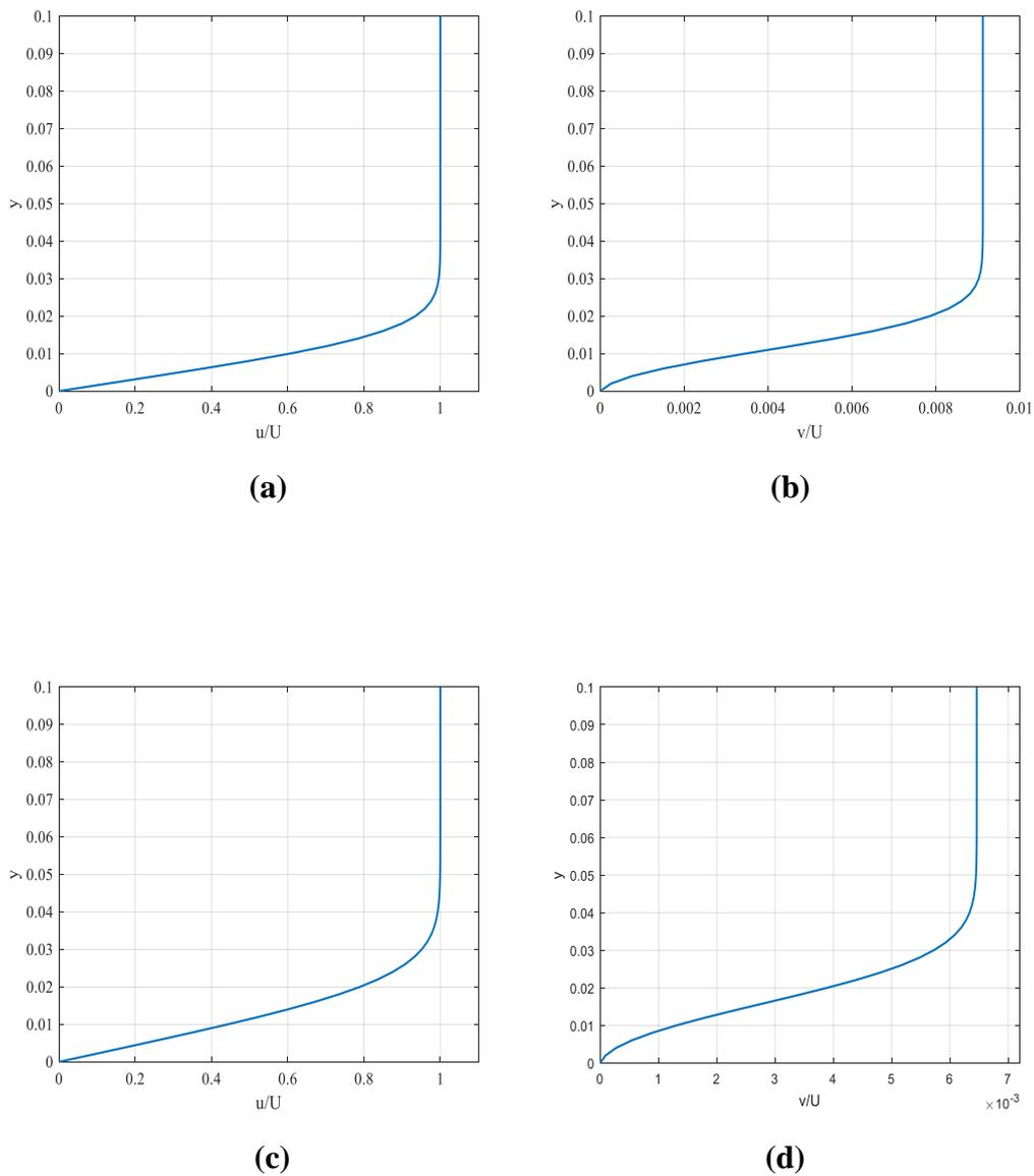
**Figure 6.16** Numerical solution of Blasius equation at  $Re = 10^4$ .
