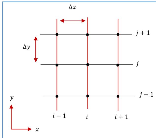
**Figure 6.1** Graphic view of grid where  $i$  runs along  $x$ -axis and  $j$  runs along  $y$ -axis
