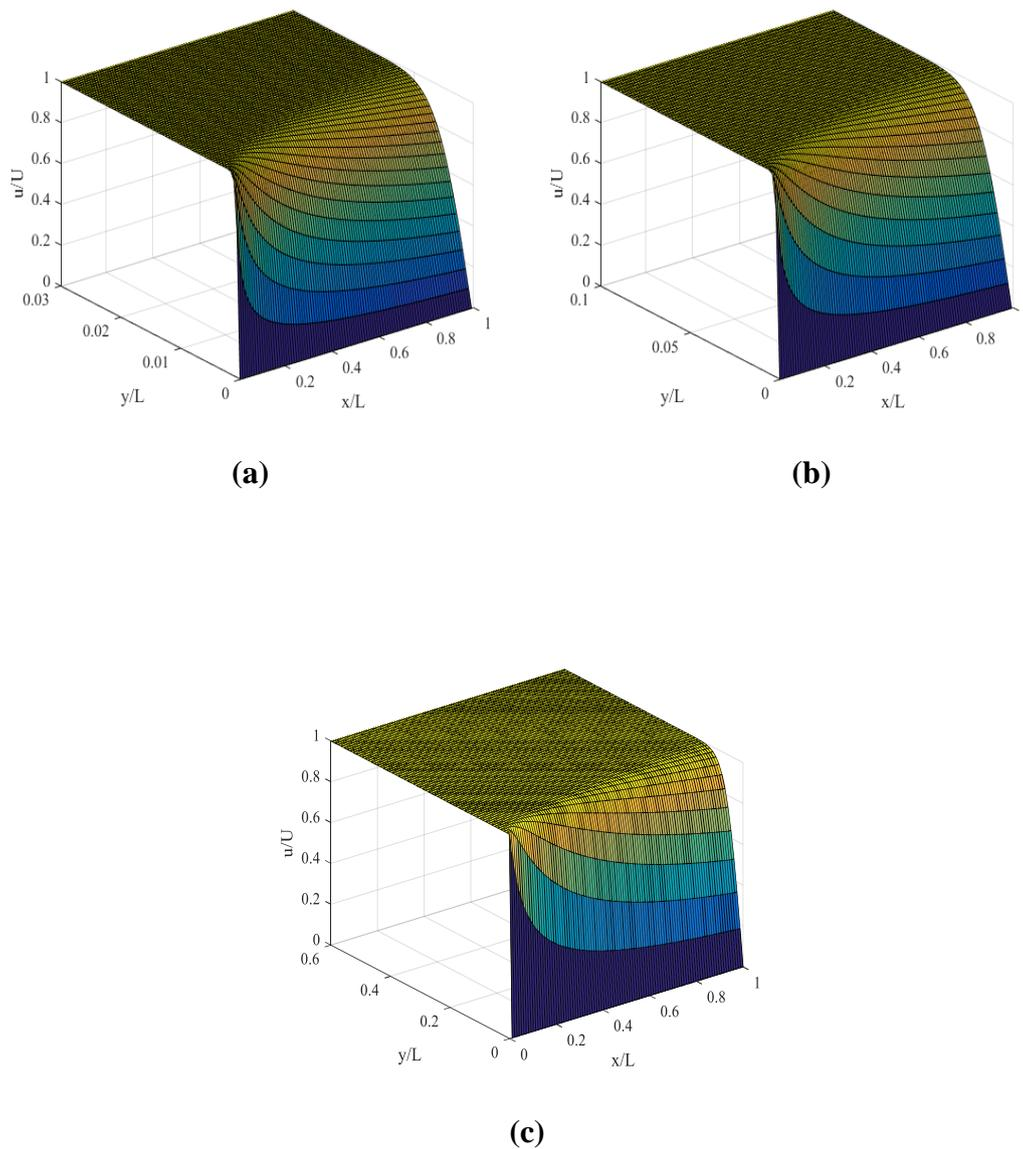
**Figure 6.12** Velocity  $u$  Surface with  $yx$ -plane of the Oseen Boundary Layer equation.
