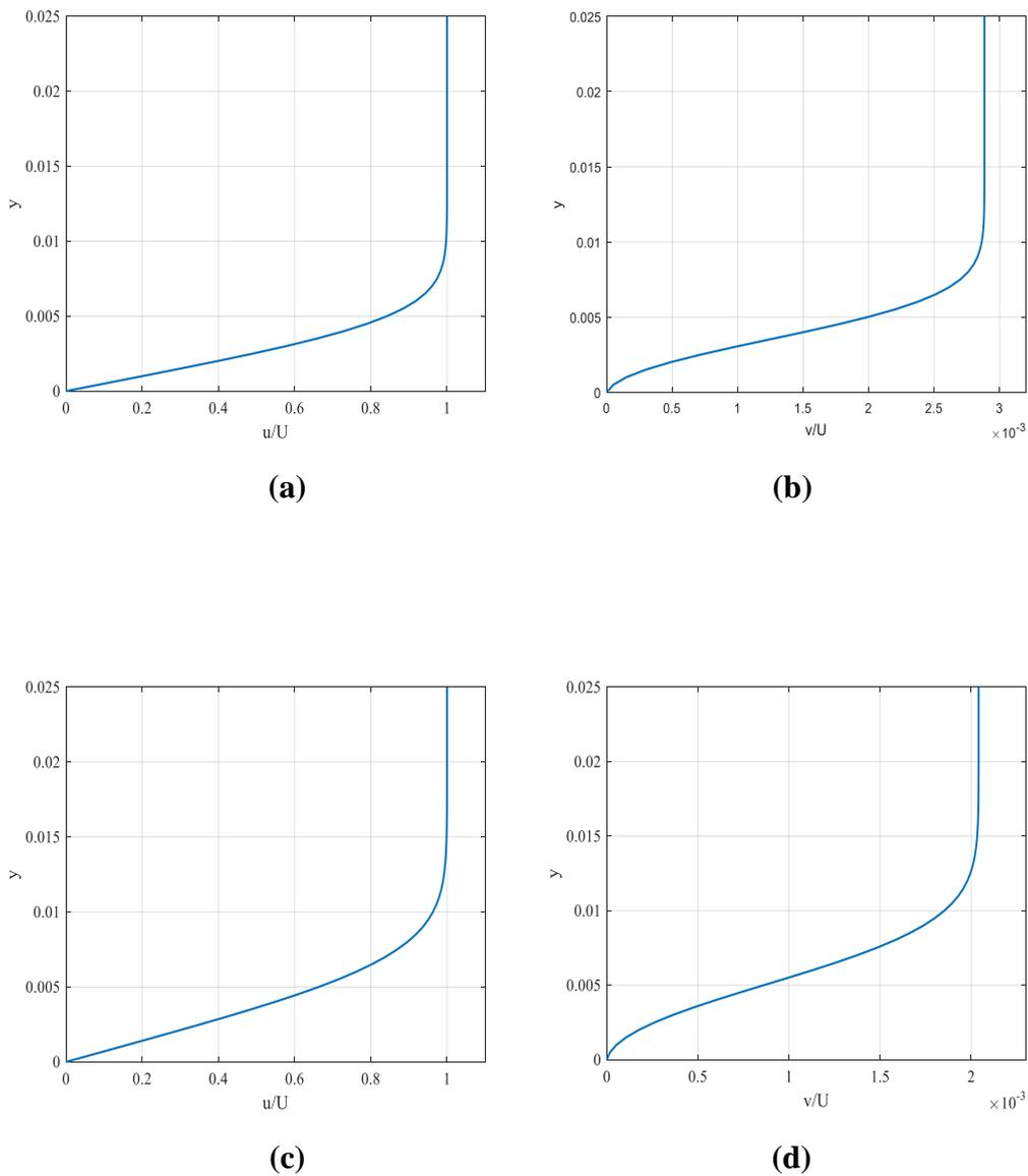
**Figure 6.15** Numerical solution of Blasius equation at  $Re = 10^5$ .
