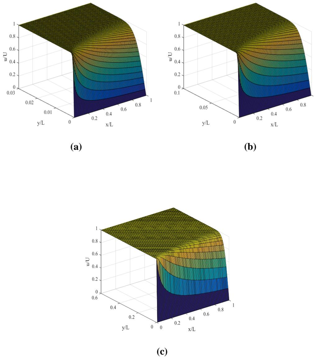
**Figure 6.24** Velocity  $u$  Surface with  $yx$ -plane of Oseen-Blasius equation.
