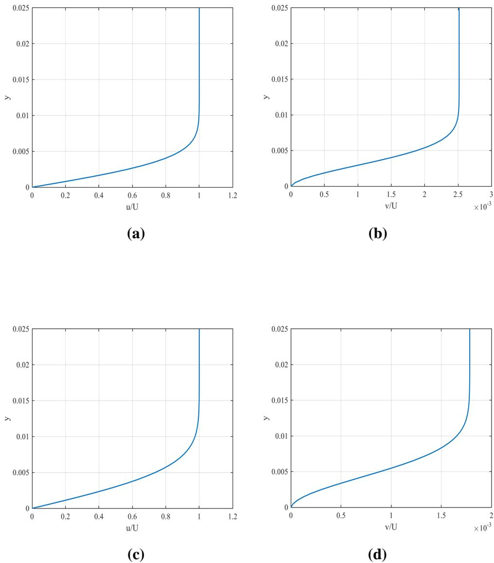
**Figure 6.21** Numerical solution of Oseen-Blasius equation at  $Re = 10^5$ .
