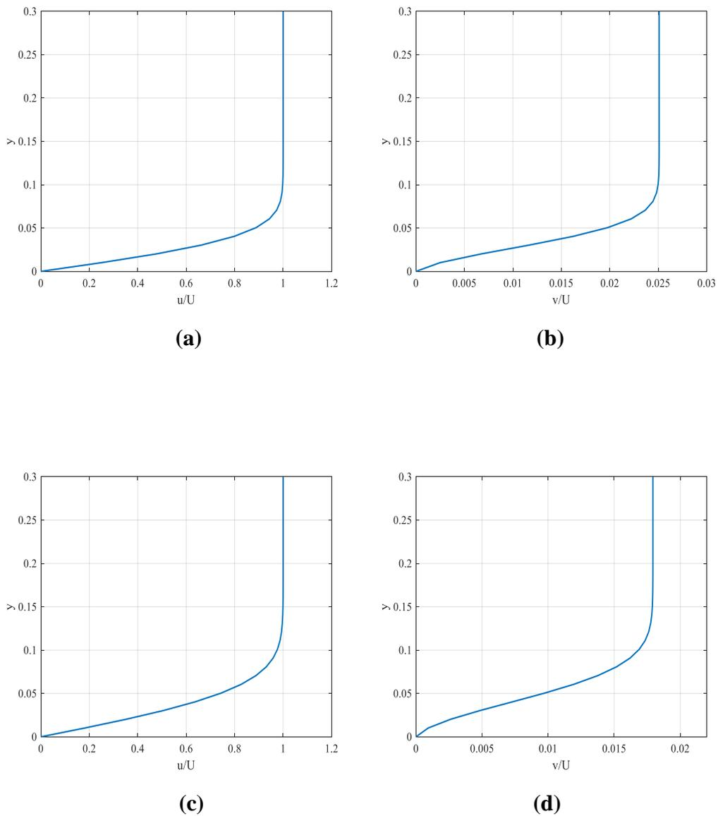
**Figure 6.23** Numerical solution of Oseen-Blasius equation at  $Re = 10^3$ .
