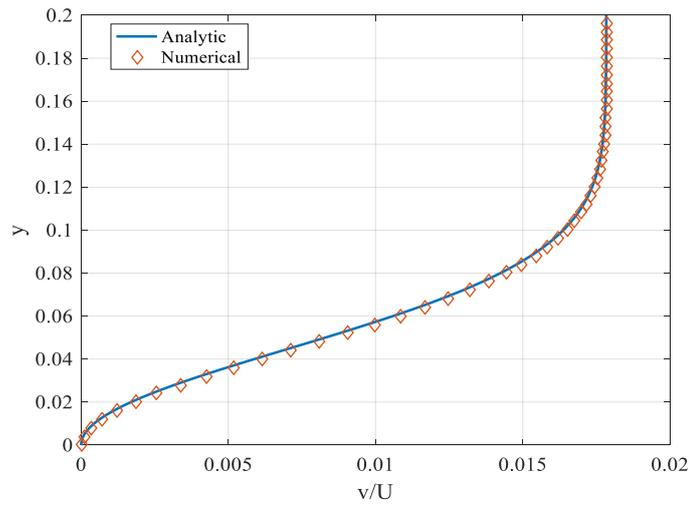
**Figure 8.8** The  $x$ -momentum velocity  $v/U$  with  $y$ -axis of analytic and numerical solution of the Oseen-Blasius equation at  $x = 1$ .
