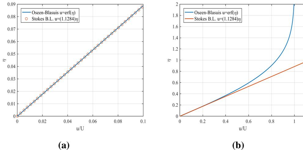
**Figure 8.14** Comparison between Stokes Boundary Layer equations and Oseen-Blasius of Velocity  $u$  at  $x=1$  and  $Re = 10^3$  and  $A = \frac{2}{\sqrt{\pi}} = 1.1284$
