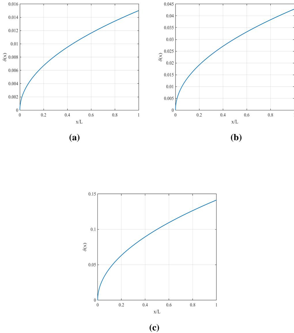
**Figure 6.19** Boundary Layer Thickness  $\delta$  with  $x$ -axis of Blasius equation.
