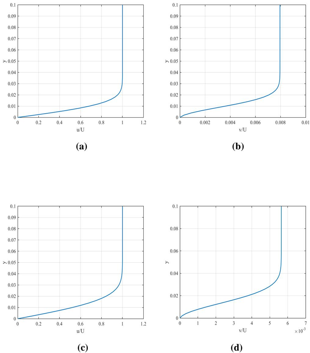
**Figure 6.22** Numerical solution of Oseen-Blasius equation at  $Re = 10^4$ .
