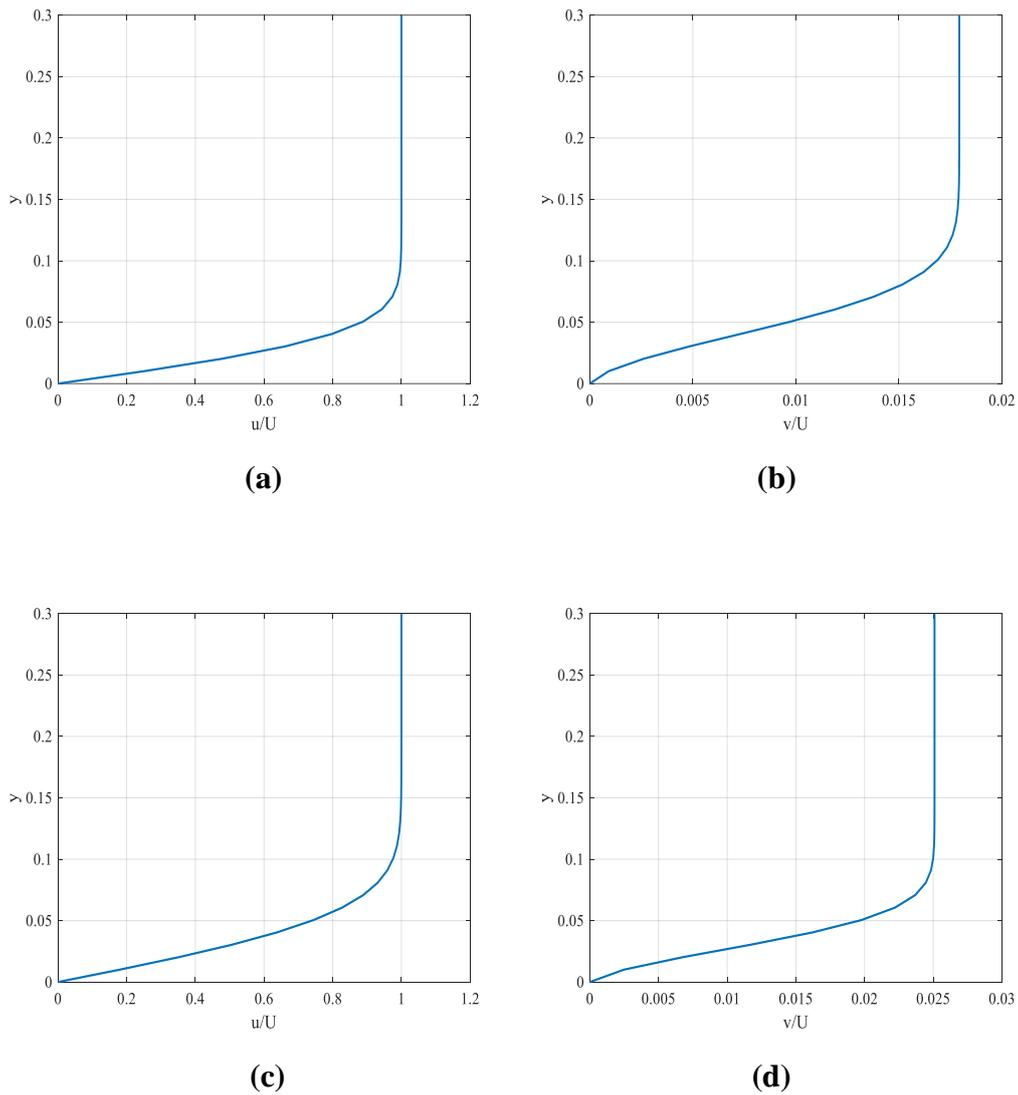
**Figure 6.11** Numerical solution of the Oseen Boundary Layer equation at  $Re = 10^3$ .
