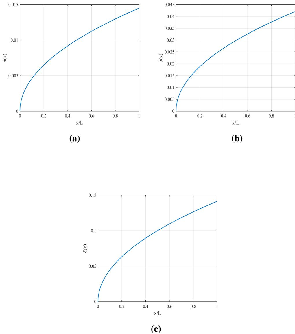
**Figure 6.13** Boundary Layer Thickness  $\delta$  of the Oseen Boundary Layer equation.
