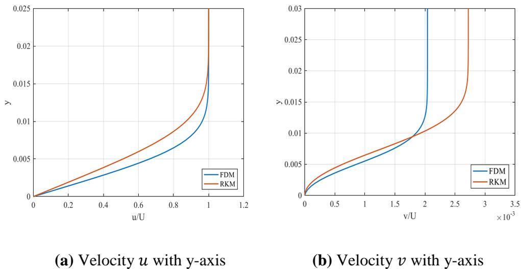
**Figure 8.10** Velocity of Blasius equation at  $x=1$  at  $Re=10^5$  by RKM and FDM.
