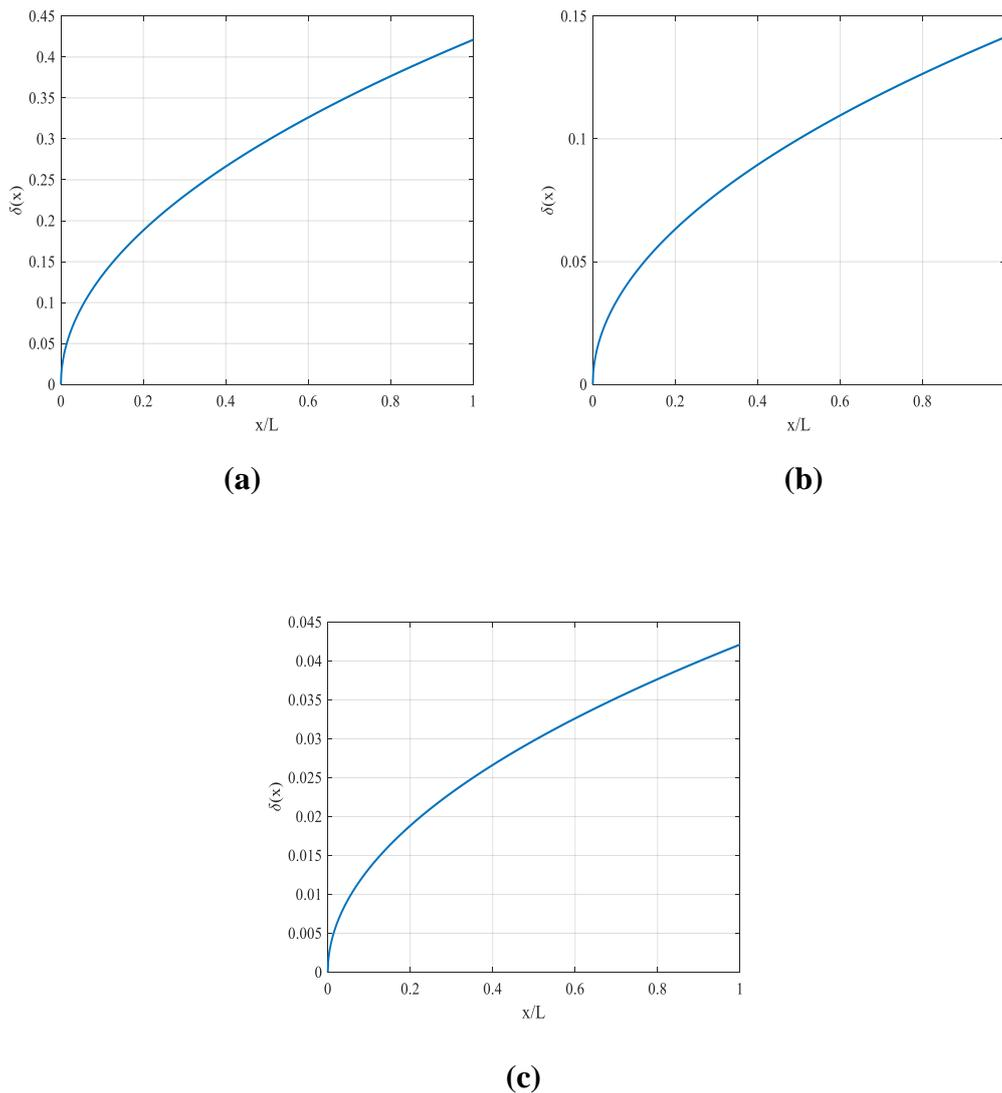
**Figure 6.7** Boundary Layer Thickness  $\delta$  with  $x$ -axis of the Boundary Layer equation.
