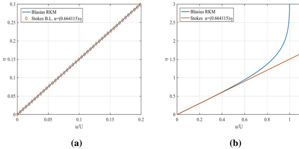
**Figure 8.15** Comparison Velocity  $u$  between Stokes near-field with  $A=0.664115$  solution and Blasius solution by Runge-Kutta method at  $x=1$  and  $Re = 10^3$ .
