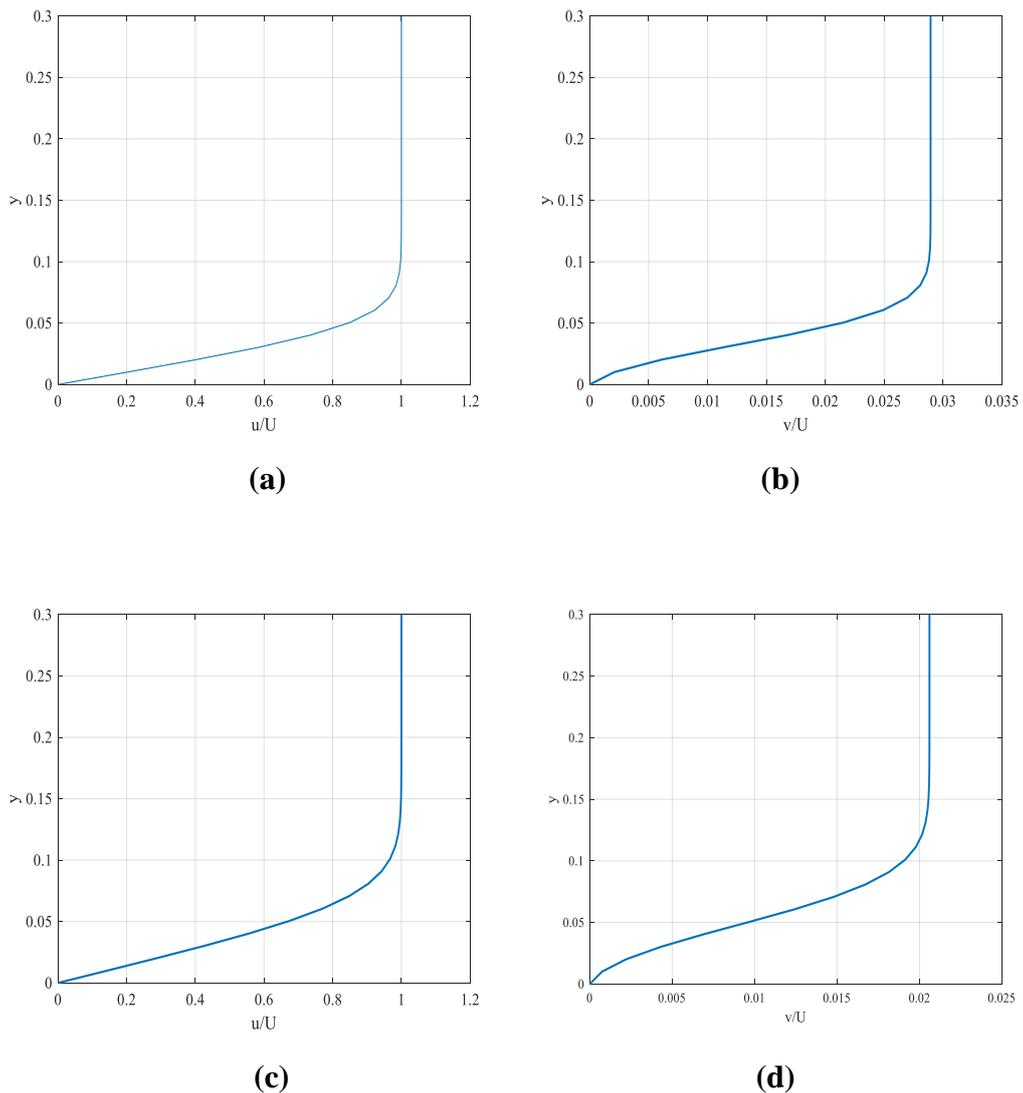
**Figure 6.5** Numerical solution of the Boundary Layer equation at  $Re = 10^3$ .
