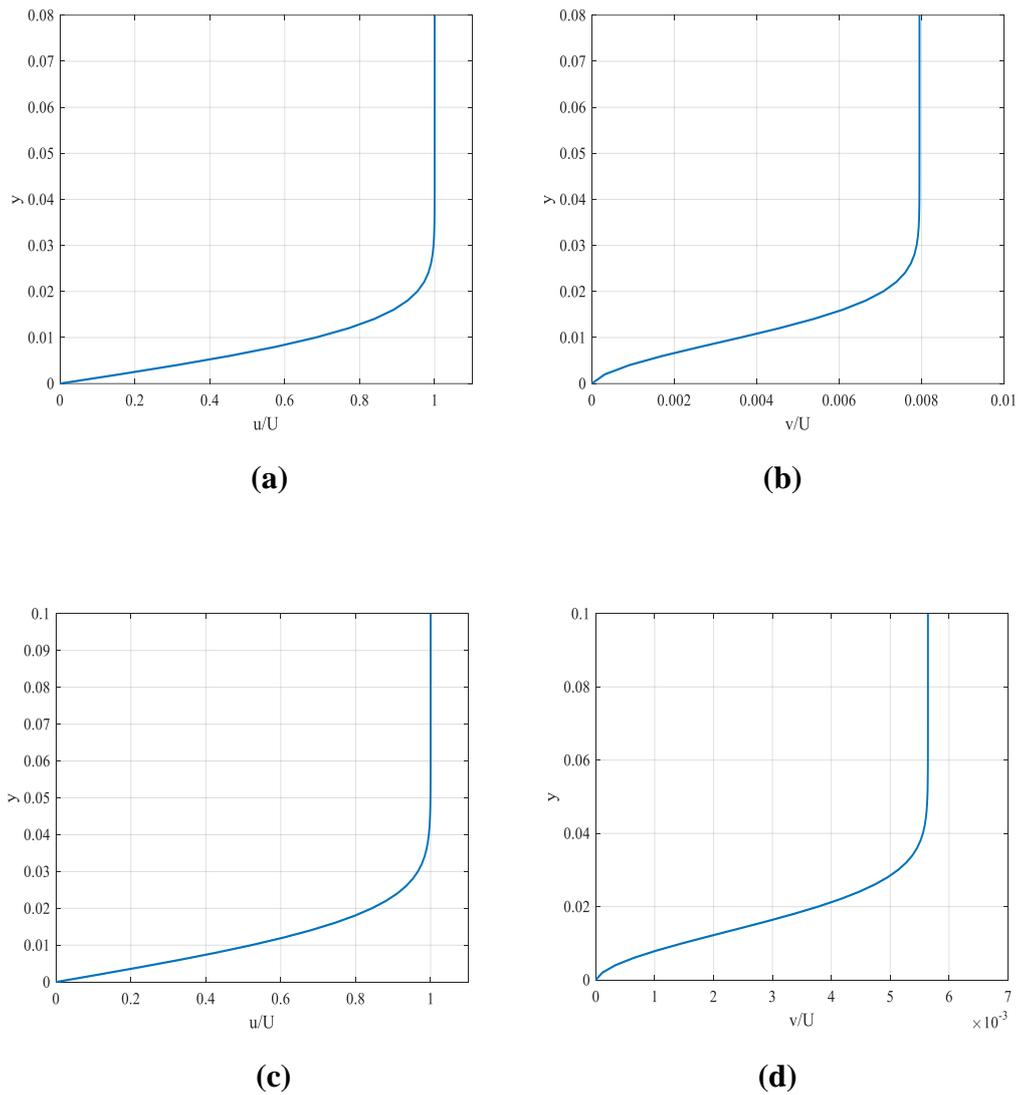
**Figure 6.10** Numerical solution of the Oseen Boundary Layer equation at  $Re = 10^4$ .
