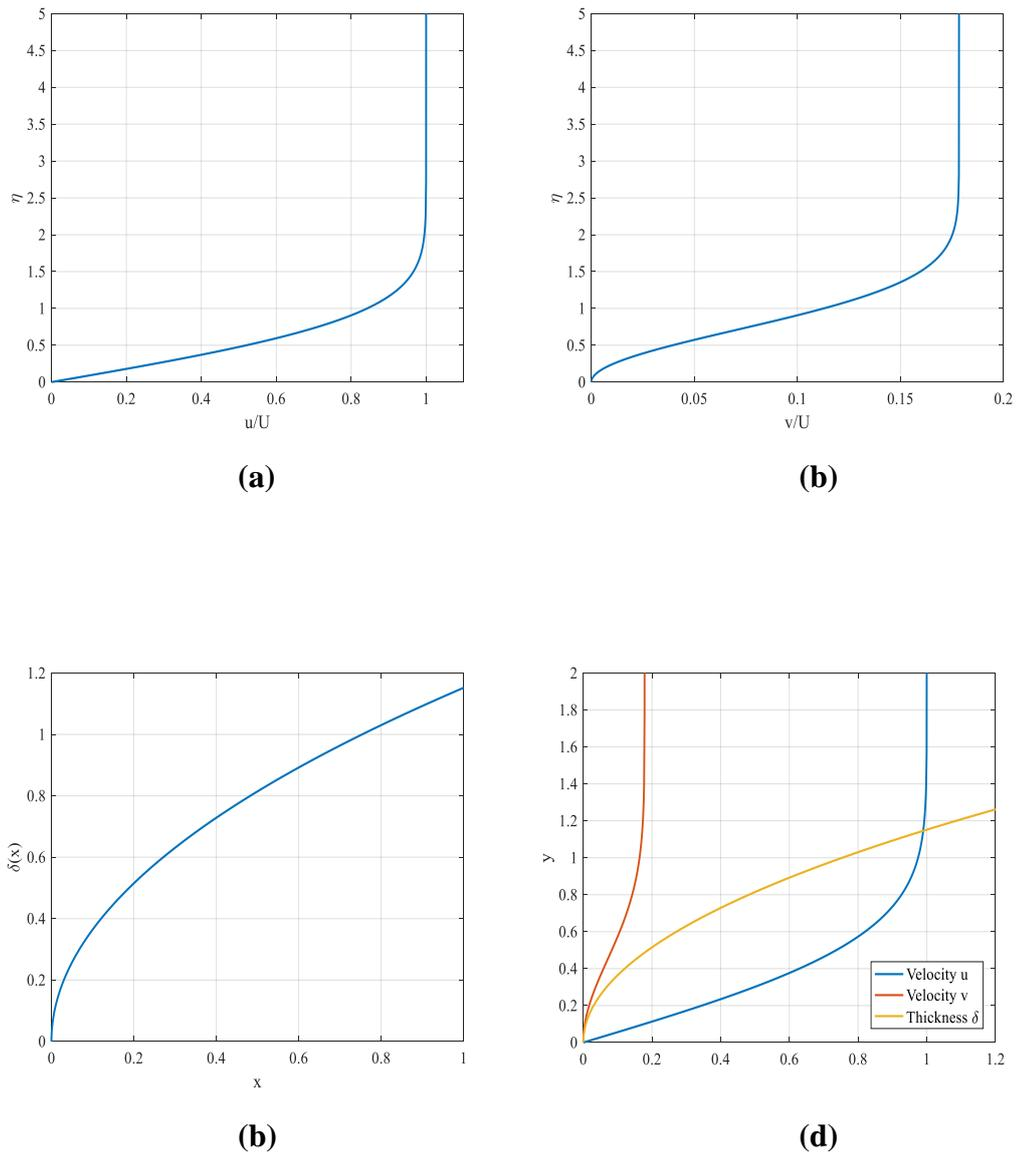
**Figure 7.4** The analytic solution of Oseen-Blasius equation
