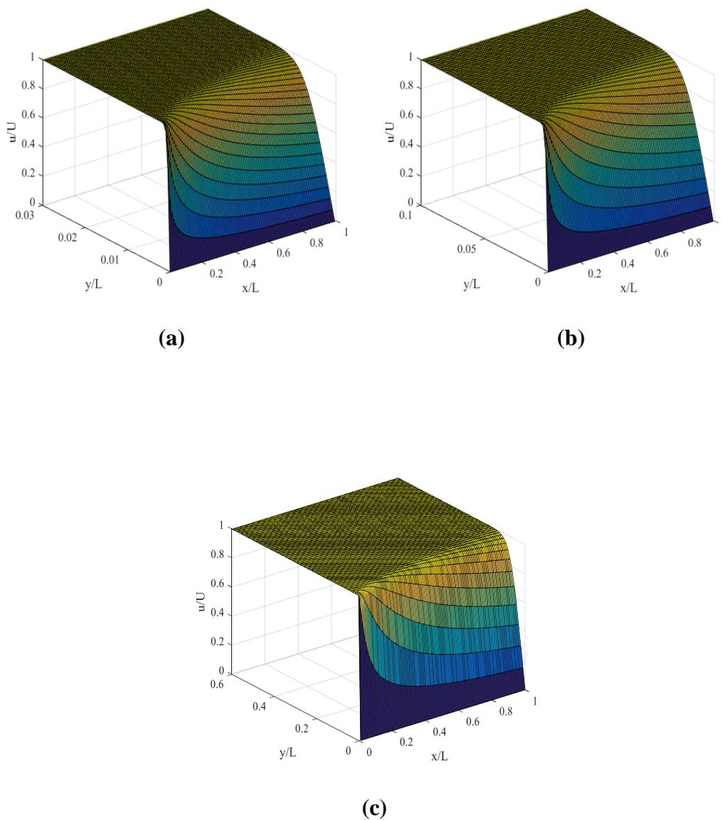
**Figure 6.18** Velocity  $u/U$  Surface with  $yx$ -plane Blasius equation.
