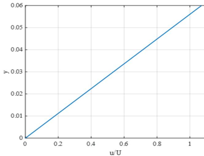
**Figure 7.5** The solution of velocity  $u$  of Stokes boundary layer equation where  $x = 1$  and  $Re = 10^3$ .
