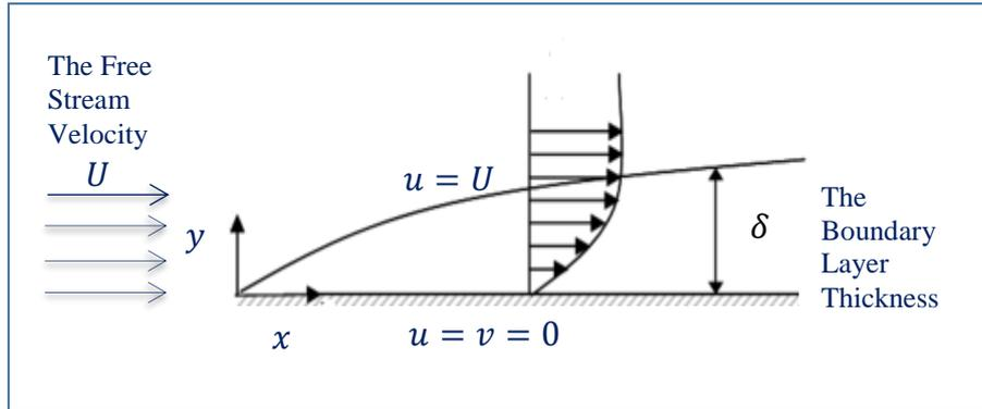
**Figure 3.1** Velocity Boundary layer development on Flat Plate
