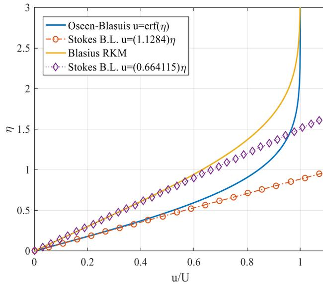
**Figure 8.16** The profile velocity  $u$  solution of Oseen-Blasius, Blasius solution by Runge-Kutta method, Stokes with  $A=2/\sqrt{\pi}$  and  $A=0.664115$ .
