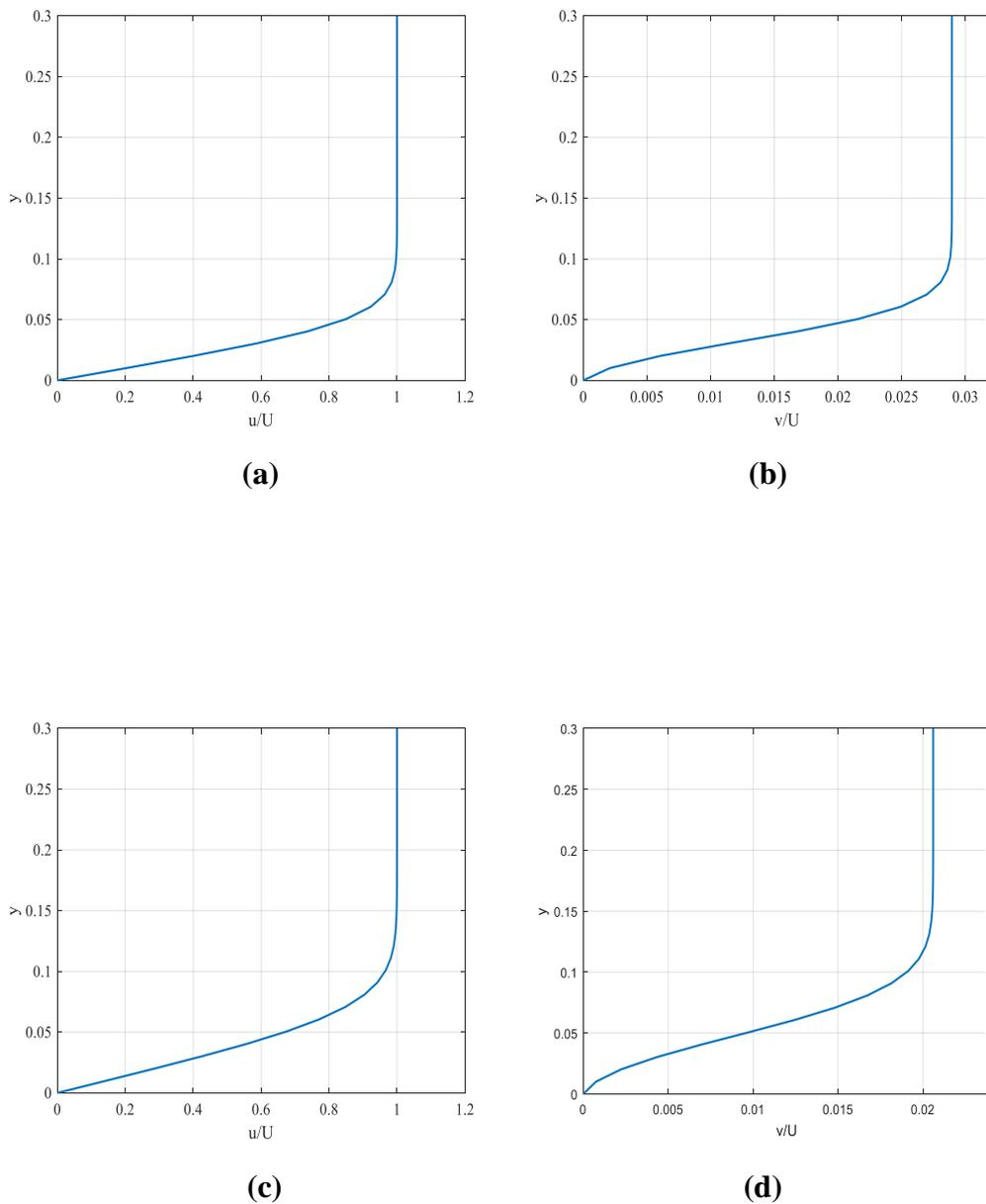
**Figure 6.17** Numerical solution of Blasius equation at  $Re = 10^3$ .
