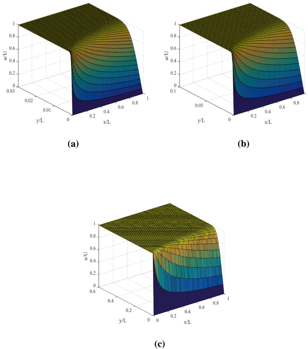
**Figure 6.6** Velocity  $u$  Surface with  $yx$ -plane of the Boundary Layer equation.
