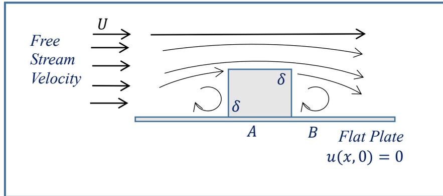
It could use the Finite Difference Method and the same Boundary conditions in Chapter 6 except on the flat plate it could be divided into 5 parts:
