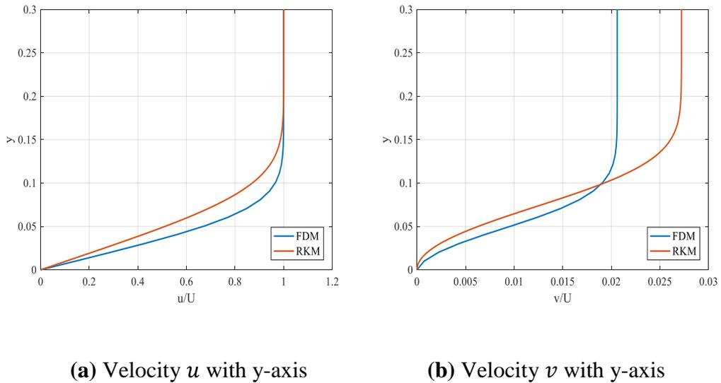
**Figure 8.12** Velocity of Blasius Equation at  $x=1$  at  $Re=10^3$  by RKM and FDM.
