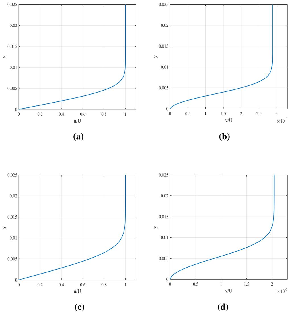
**Figure 6.3** Numerical solution of the Boundary Layer equation at  $Re = 10^5$ .
