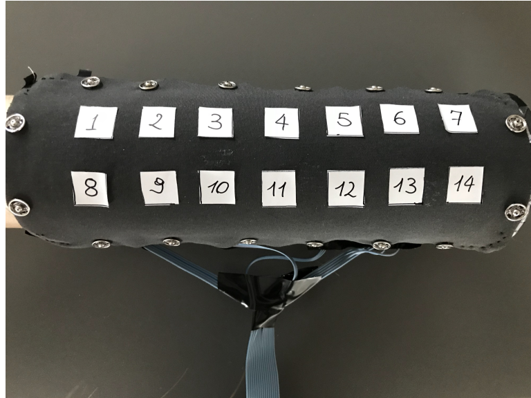
Figure 5.11: Electrical tomography flexible fabric sensor implemented over a curved surface with bending radius of 3 cm, and presenting C = 14 touch input classes
