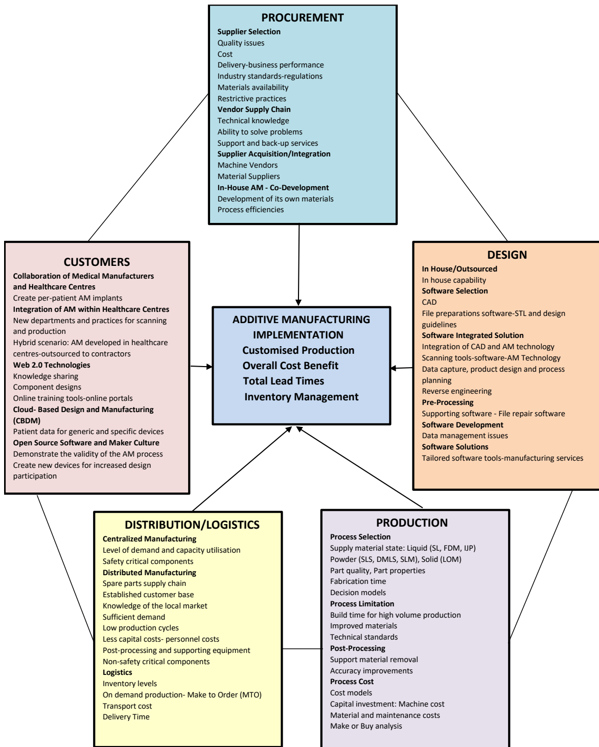
Figure 3.7: Additive Manufacturing Implementation Framework
