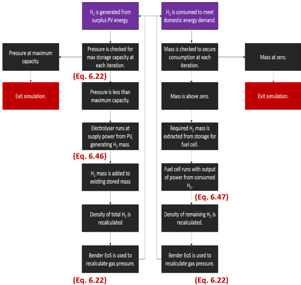
Figure 6.21 – Operational flow of hydrogen storage logic as a result of surplus or deficit in photovoltaic energy supply.
