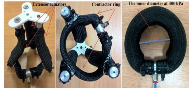
Figure 17. The structure of the extension-circular gripper.
