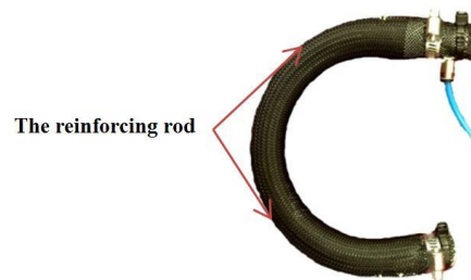
Figure 6. A 30 cm self-bending contraction PMA
