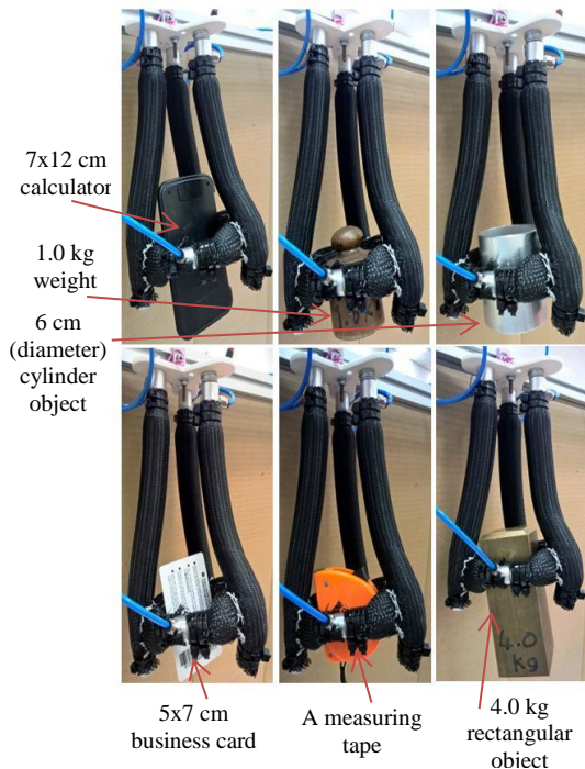
Figure 20. Multiple objects grasped by the extension-circular gripper.
