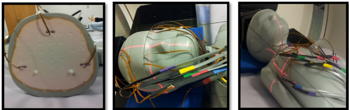
Figure 5-15: Paediatric phantom MOSFET loading and scan set up.
