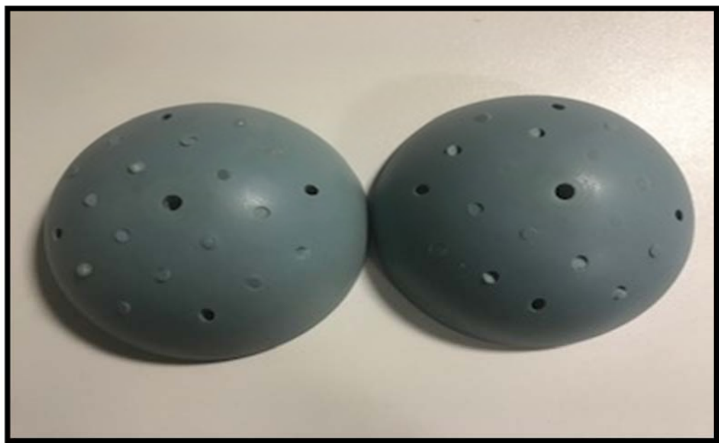
Figure 5-7: Female single breasts attachment (350cc) 701-BR-350 (CIRS, 2013). The unplugged holes were used for MOSFET accommodation.
