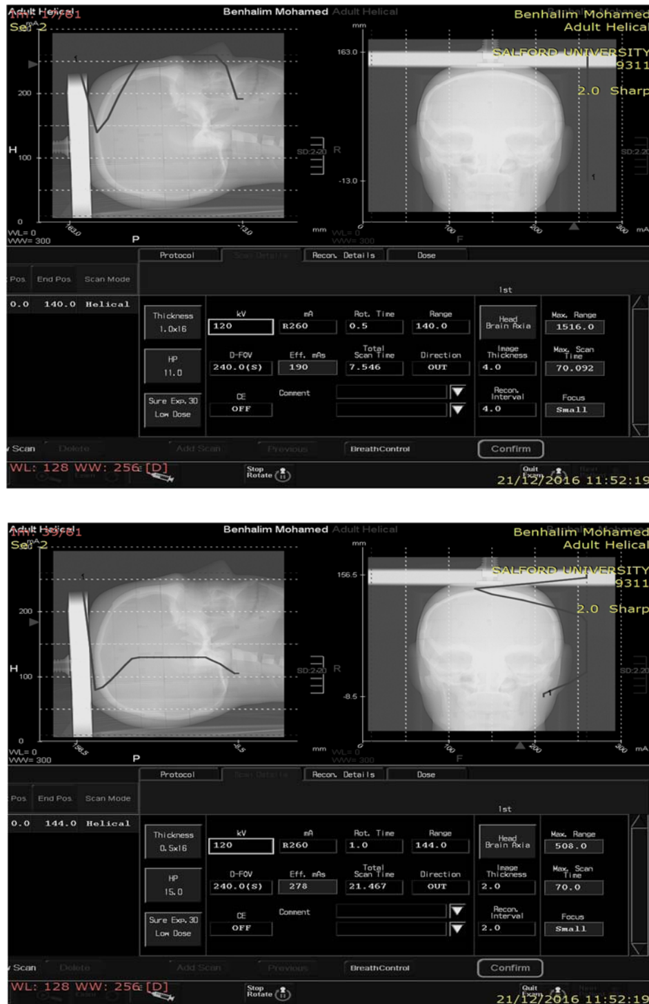
Figure 6-1: Angular and longitudinal mA modulation.
