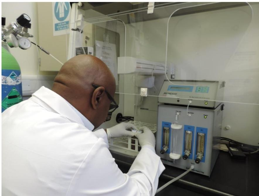
Figure 5. 2: Sample analysis using Cold Vapor Atomic Fluorescence Spectrometry
