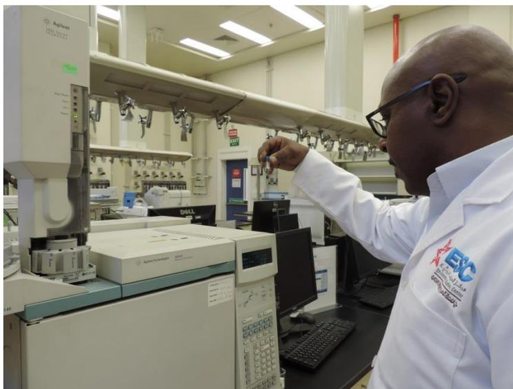
Figure 3. 1: Sample analysis using gas chromatography coupled to an electron capture detector.
