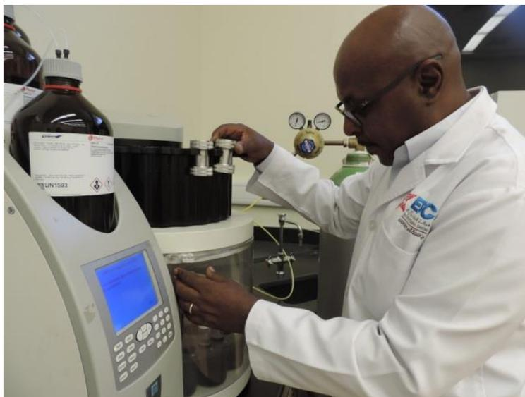
Figure 4. 6: Sample extraction using Dionex Accelerated solvent extractor.
