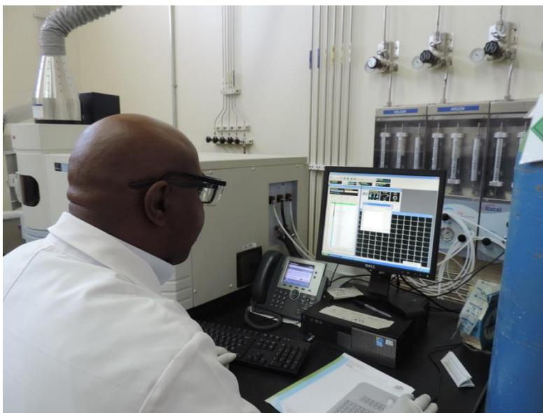
Figure 3. 2: Heavy metal analysis using inductively coupled plasma coupled to optical emission spectrometry.
