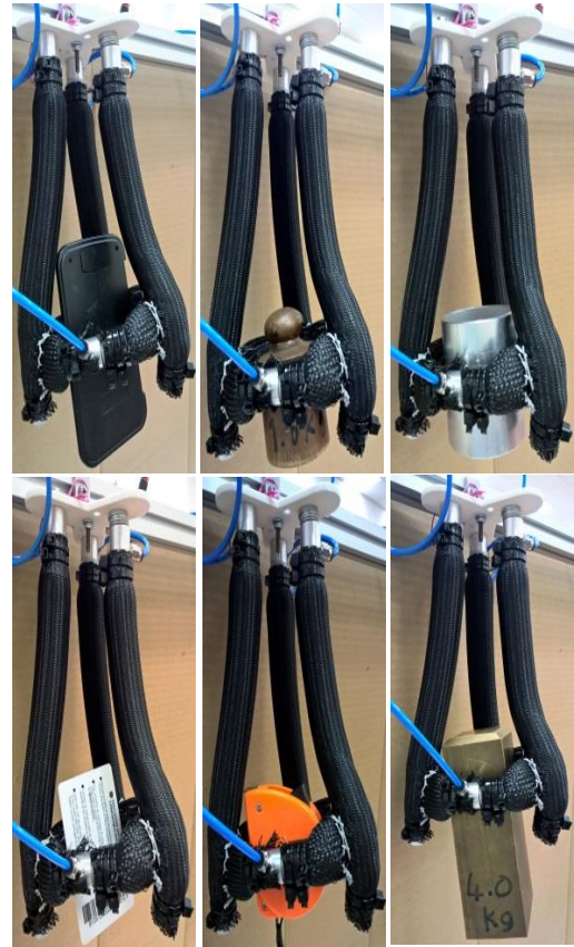
Figure 8. Multiple objects grasped by the extension-ring gripper.
