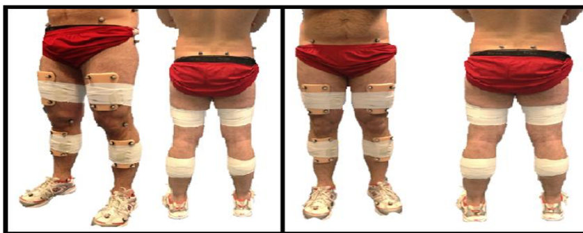
Figure 3.8 Static (left) and tracking (right) marker placement
