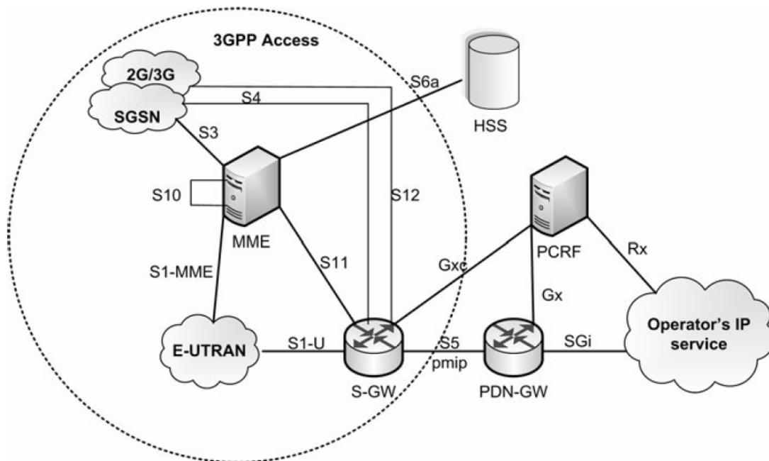
**Figure 2-2: LTE-A Reference Model [13]**
