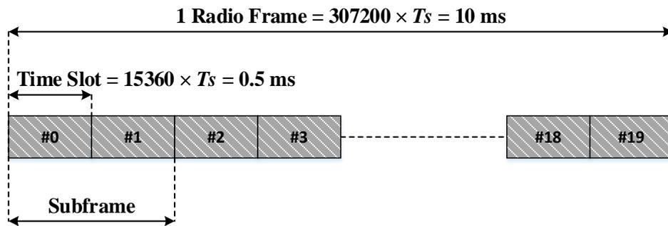
**Figure 2-3: Radio Frame Structure (type1)**
