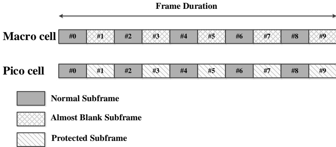
**Figure 3-3: Example of (ABS) for range expansion in heterogeneous network**
