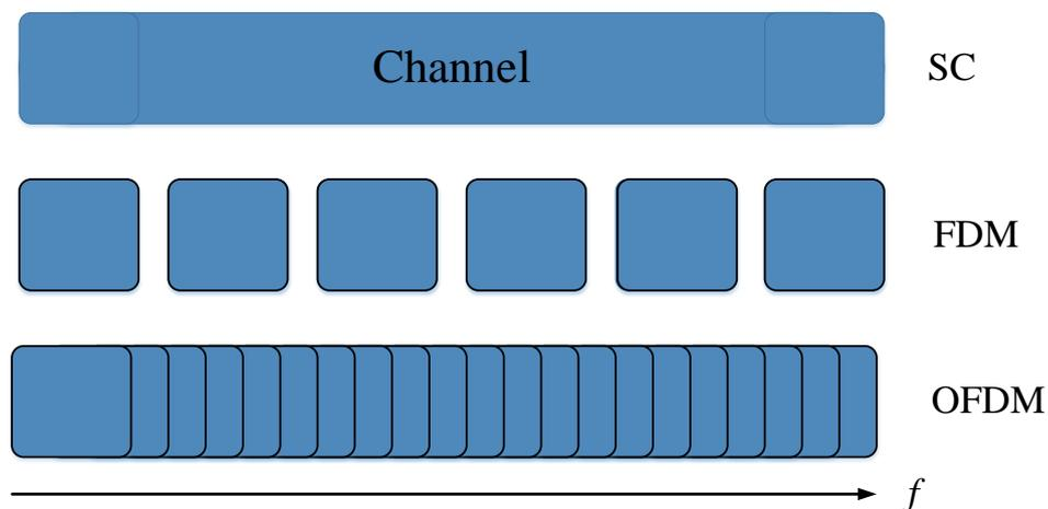
**Figure 2-1: A graphical illustration of OFDM scheme**
