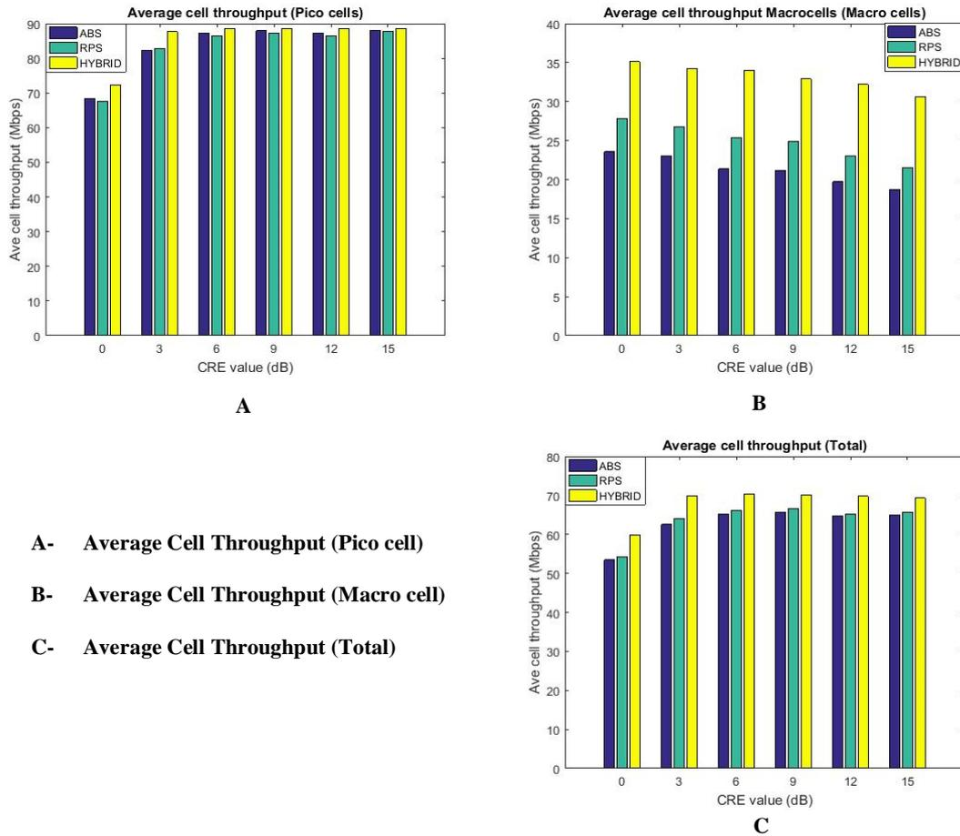
**Figure 5-20: Average Cell Throughput (Comparison with other Schemes)**
