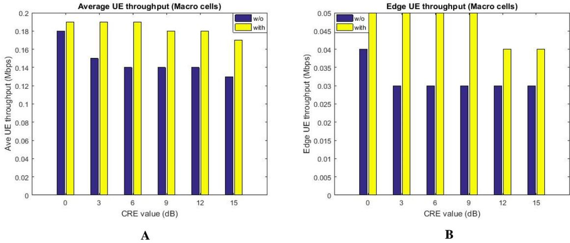
**Figure 5-10: Macro UE Throughput (Algorithm Evaluation)**
