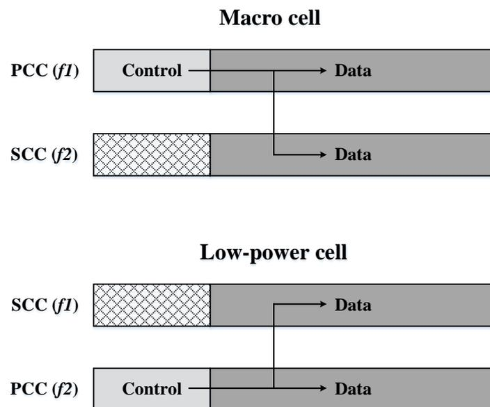
Figure 3-2: Frame configuration for CA-based ICIC scheme
