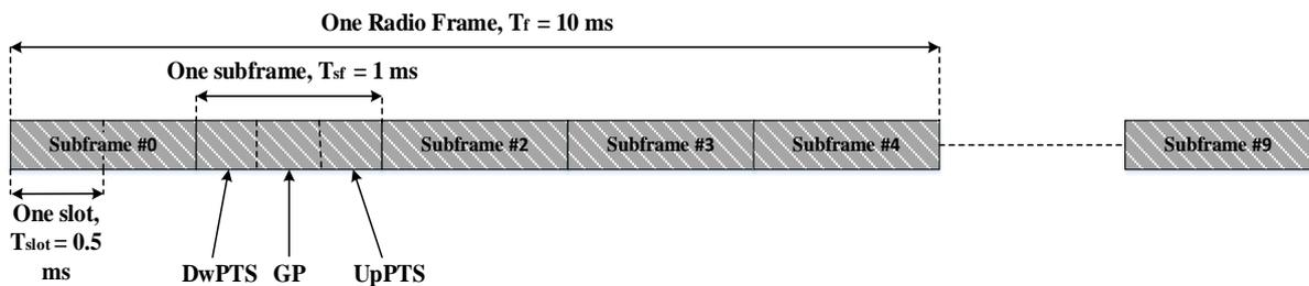
**Figure 2-4: Radio Frame Structure (type 2)**
