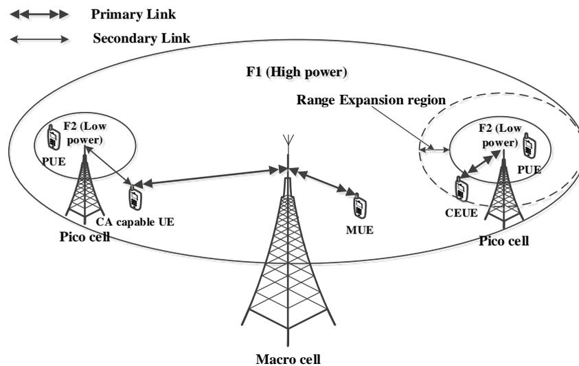
**Figure 2-6: Heterogeneous deployment in LTE-Advanced network**
