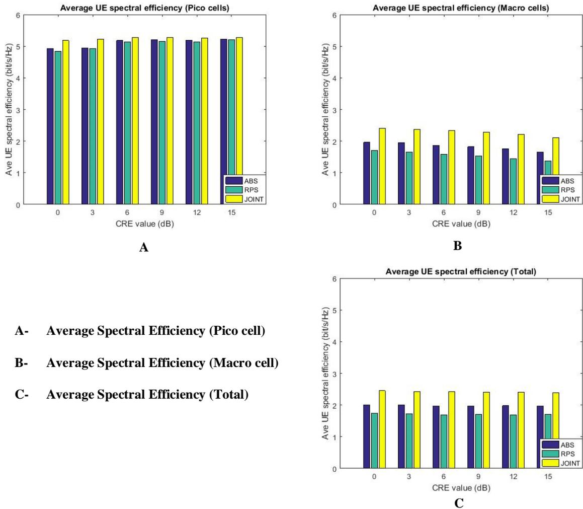
**Figure 5-22: Average Spectral Efficiency (Comparison with other Schemes)**
