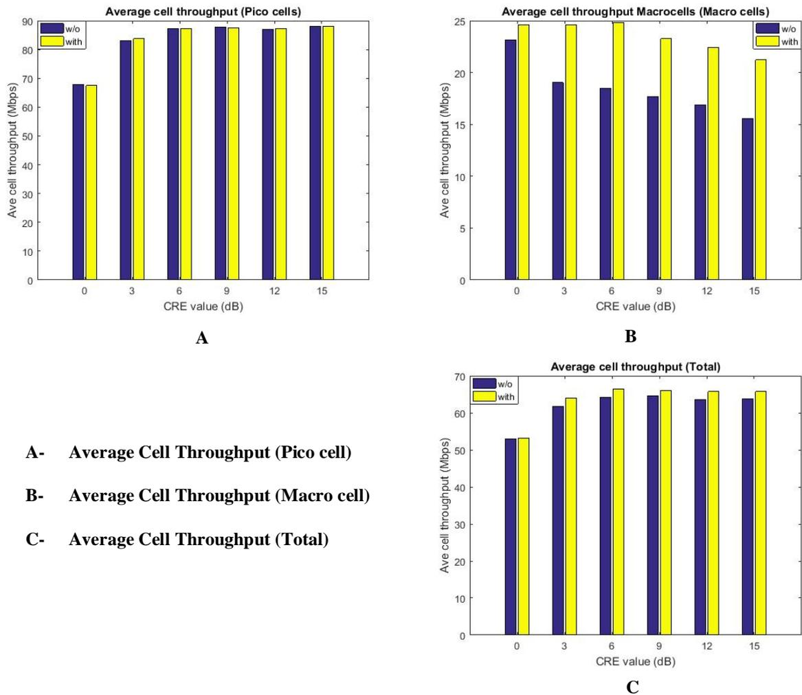
**Figure 5-12: Average Cell Throughput (Algorithm Evaluation)**
