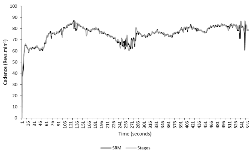
Figure 5. Mean cadence averaged at 1 second intervals for SRM and Stages Powermeters.
