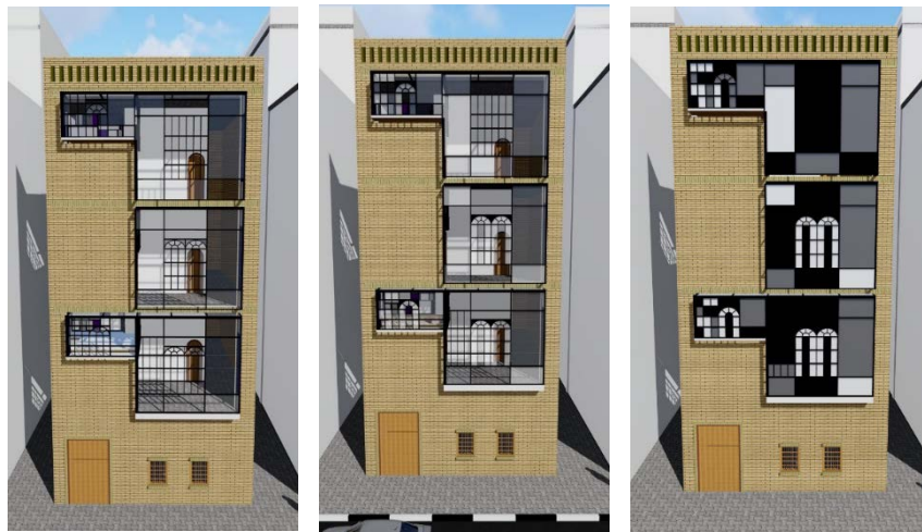
Figure 5.3 demonstrates the dsitribution of smart window/wall/balcony elements in a multi-storey building which expresses the changing state from transparent to semi-transparent to opaque.
