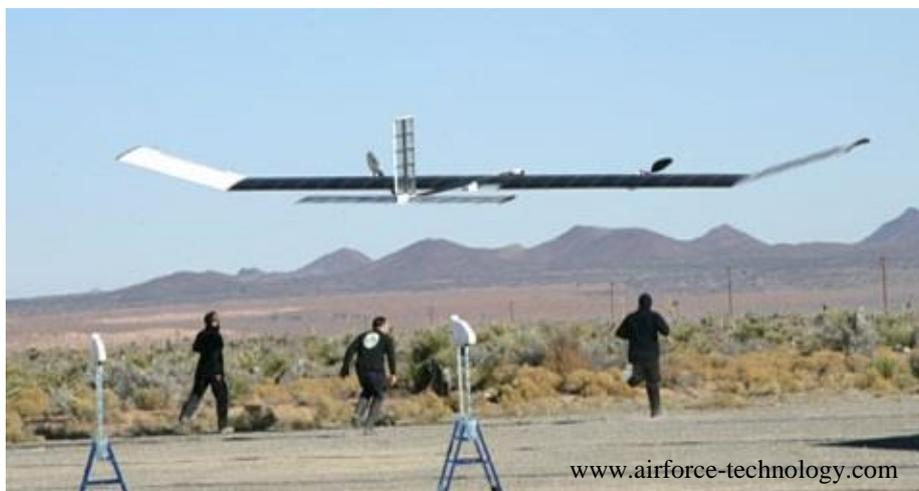
Figure 2-4 Qinetiq Zephyr UAV
