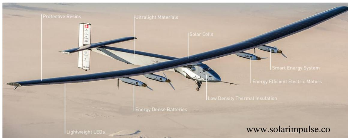
Figure 1-2 Solar Impulse-2 aircraft
