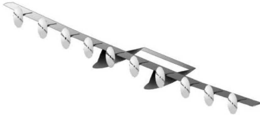
Figure 2-8 Rectangular braced-wing configuration in (Baldock & Mokhtarzadeh, 2006)
