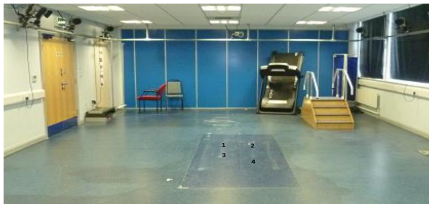
Figure 3-7: The gait laboratory with 16 infra-red cameras (Qualisys Oqus motion analysis system) and four force platforms.
