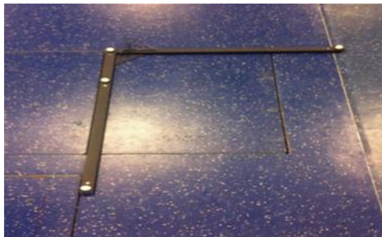
Figure 3-8: L-shaped metal frame with four markers.
