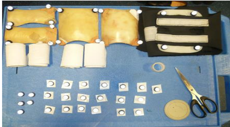
Figure 3-11: Retro-reflective markers, cluster pads, bandages, and hypoallergenic double sided adhesive tape.
