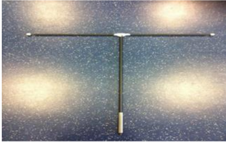
Figure 3.9: T-shaped wand with two markers.
