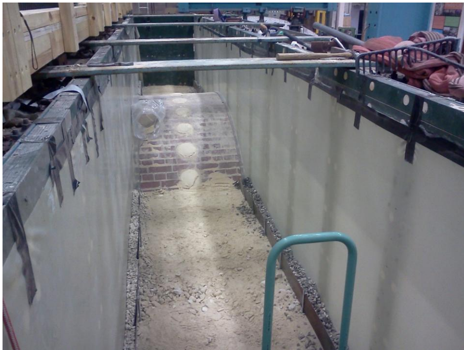
Figure 2.17 – Fill placement in progress, course fill coloured with ash placed in front of windows, pressure cells covered with sand, greased latex lining on Perspex slab walls
