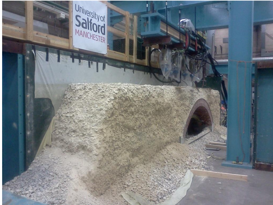
Figure 2.24 – South west perspective of main fill and arch after EP1 after removal of south chamber wall
