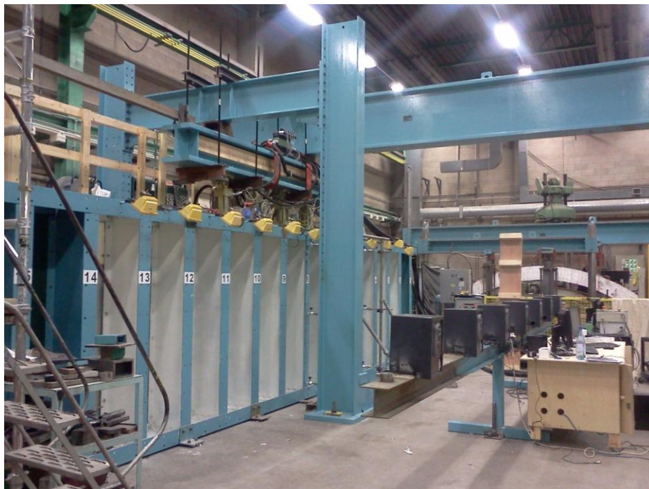
Figure 2.23 – General perspective of apparatus (left), rig supporting camera array (centre), control and data acquisition terminals (right)
