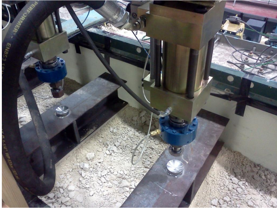
Figure 2.20 – Loading arrangement showing bearing points between actuator heads and steel sleepers, timber interfacing steels to fill surface.
