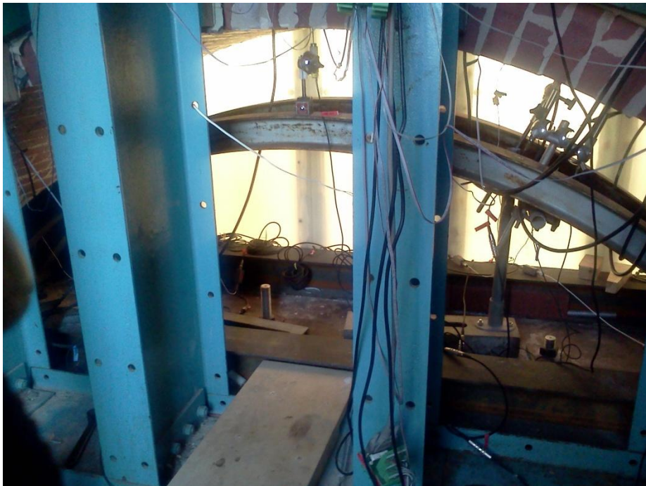
Figure 2.21 – Arrangement of LVDT displacement gauges on arch intrados
