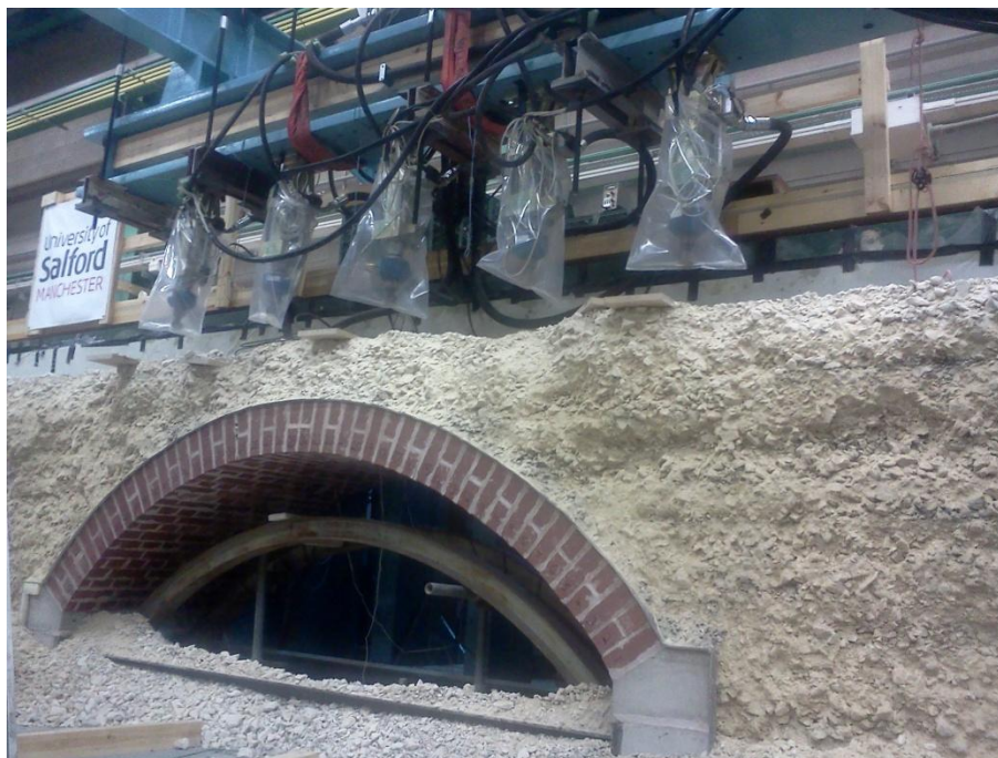
Figure 2.25 - South east perspective of main fill and arch after EP1 after removal of south chamber wall
