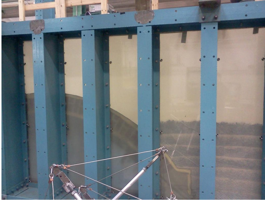
Figure 2.18 – View of compacted layers of fill through chamber windows during placement
