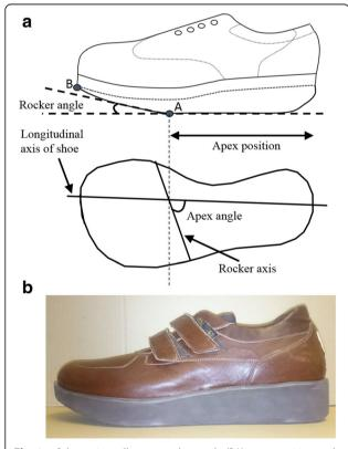
**Fig. 1 a** Schematic to illustrate rocker angle (RA), apex position and apex angle. Apex position was varied by moving point A proximally or distally and a corresponding adjustment made to the position of point B to ensure a consistent rocker angle. **b** Example rocker shoe with  $RA = 20^{\circ}$
