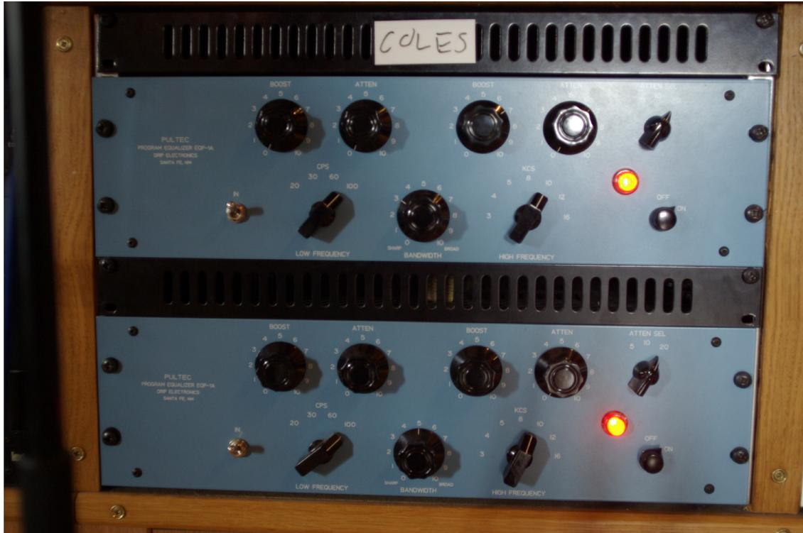
*Figure 49: Pultec equalisers used to brighten the Coles ribbon microphones*
