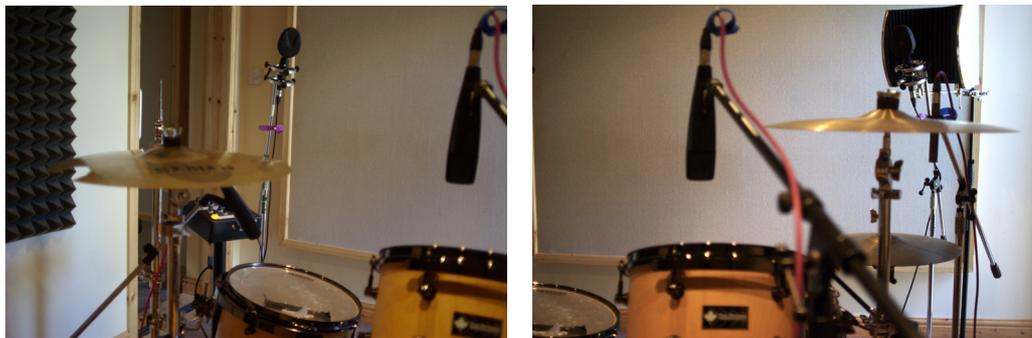
*Figure 48: Overheads - Coles ribbon microphones positioned behind the player*
