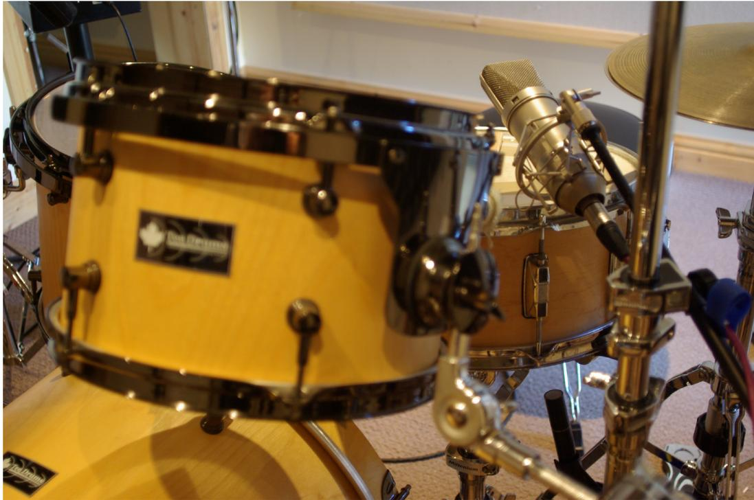
*Figure 51: Neumann U87a on the top of the snare drum with a Beyer 201 underneath*
