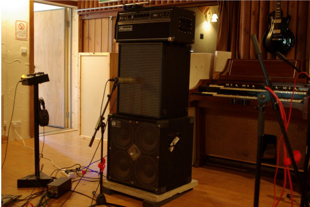
Figure 54: Foam blocks and a concrete slab were used to decouple the cabinet from the floor, reducing vibrations
