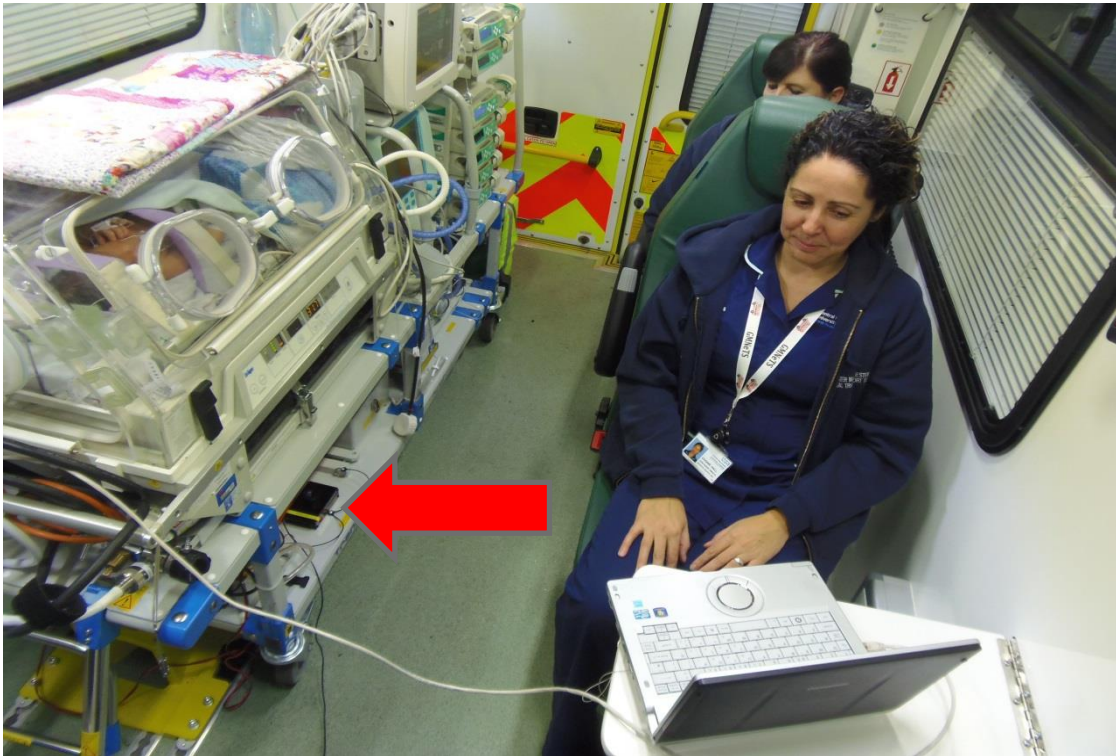
Figure 7: Position of transport incubator in ambulance and location of DL1 data logging device.
