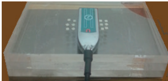
Figure (7) Demonstrates the TLD calibration process against the Unfors solid state dosimeter on three Perspex slabs.
