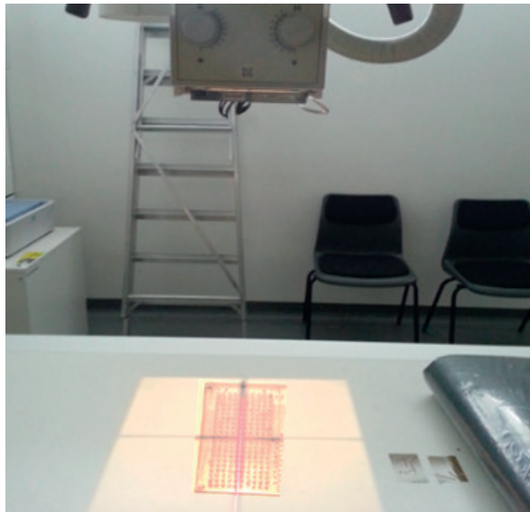
Figure (6) Illustrates the TLD positioning during exposure. The TLDs are positioned as close as possible to the central ray to minimise the impact of the anode-heel effect.
