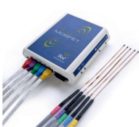
Figure (11) MOSFET reader and five dosimetries (34).
