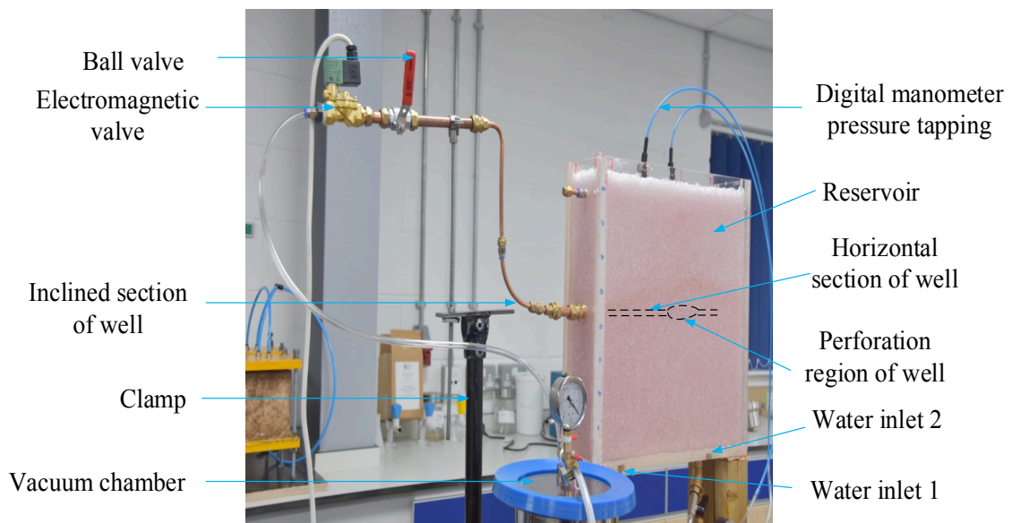
Fig. 1 Water and gas cresting rig (after Akangbou et al. 2017)
