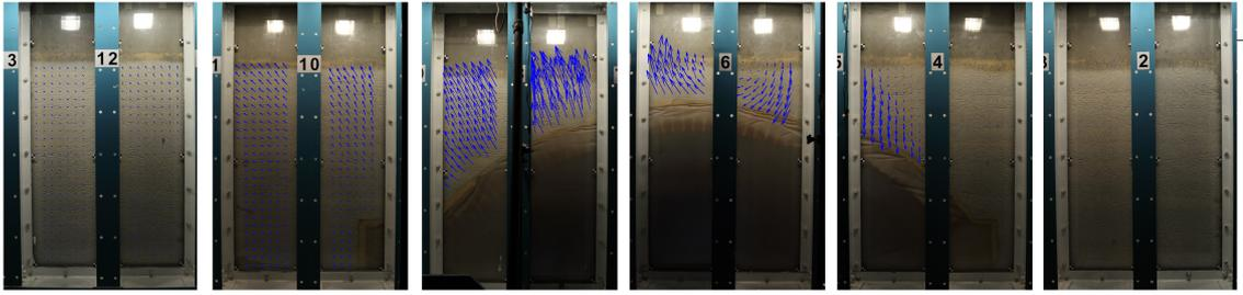
FIG. 12: Deformation of soil - four hinge failure mechanism (EP1)
