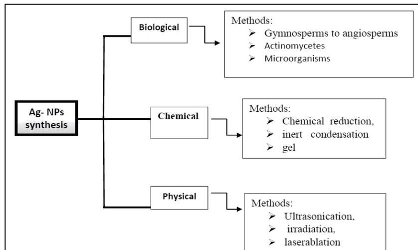
**Figure 4:** Different routes to synthesis of nanoparticles
