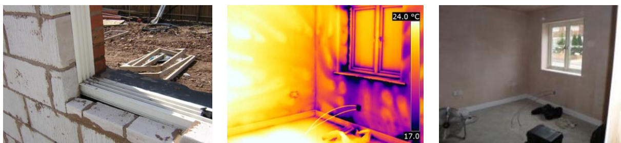
Figure 3. Air leakage due to ineffective seals at wall openings (source Smith et al 2005; Farmer et al 2014)
