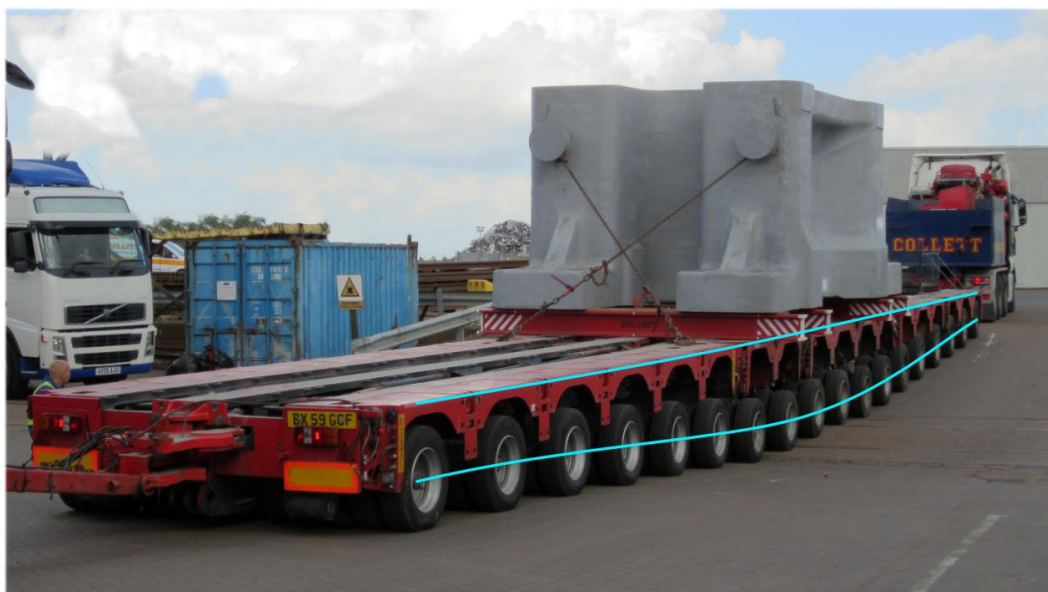
Figure 1. Modular Trailer axle compensation. Source: Collett & Sons Ltd.
