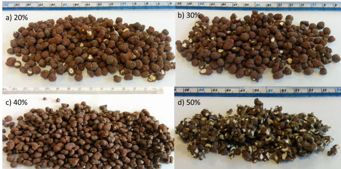
Figure 2. Granules with a sintered clay coating and APCr core containing: a) 20%, b) 30%, c) 40% and d) 50% sodium silicate.
