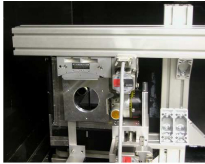
Fig. 1. Shearing-grating setup at CONRAD instrument. The round-shaped phase grating can be seen in the center.
