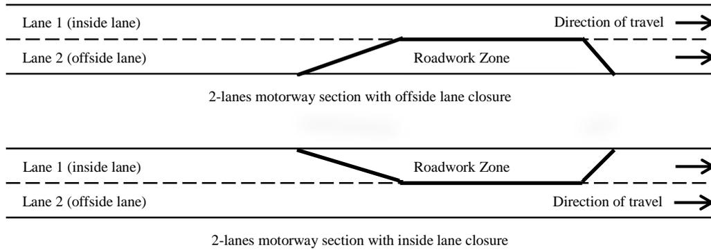
**Figure 8.2: Schematic layouts of the tested 2-lanes motorway roadwork sections**
