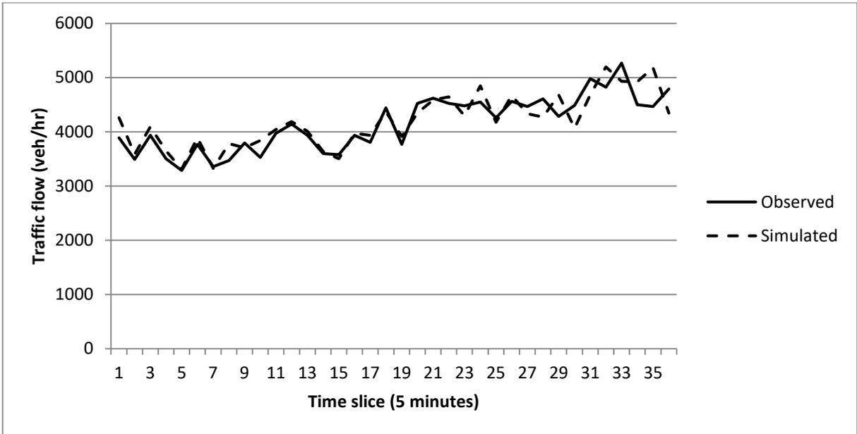
Figure 7.26: Validation - simulated versus observed traffic flow data (M42)
