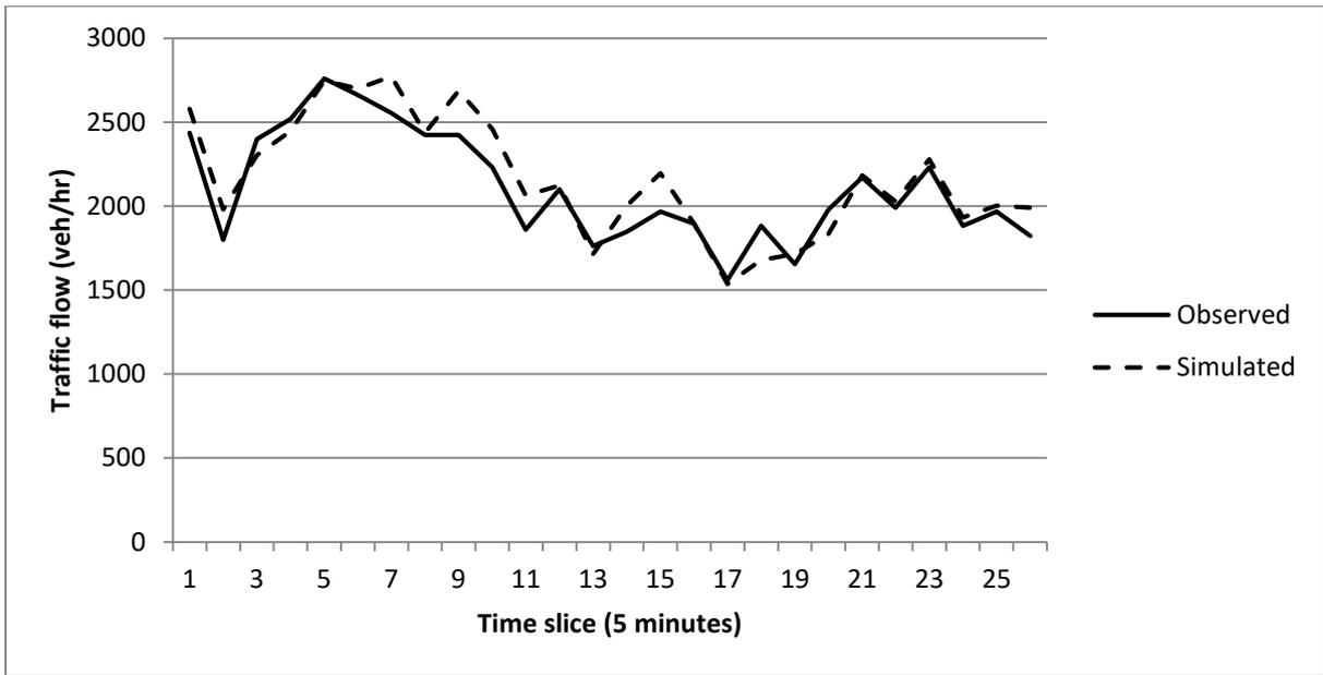
Figure 7.29: Validation - simulated versus observed traffic flow data (M602)
