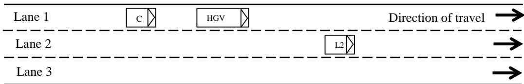
**Figure 6.21: Illustration of the surrounding vehicles for the avoider (vehicle C)**
