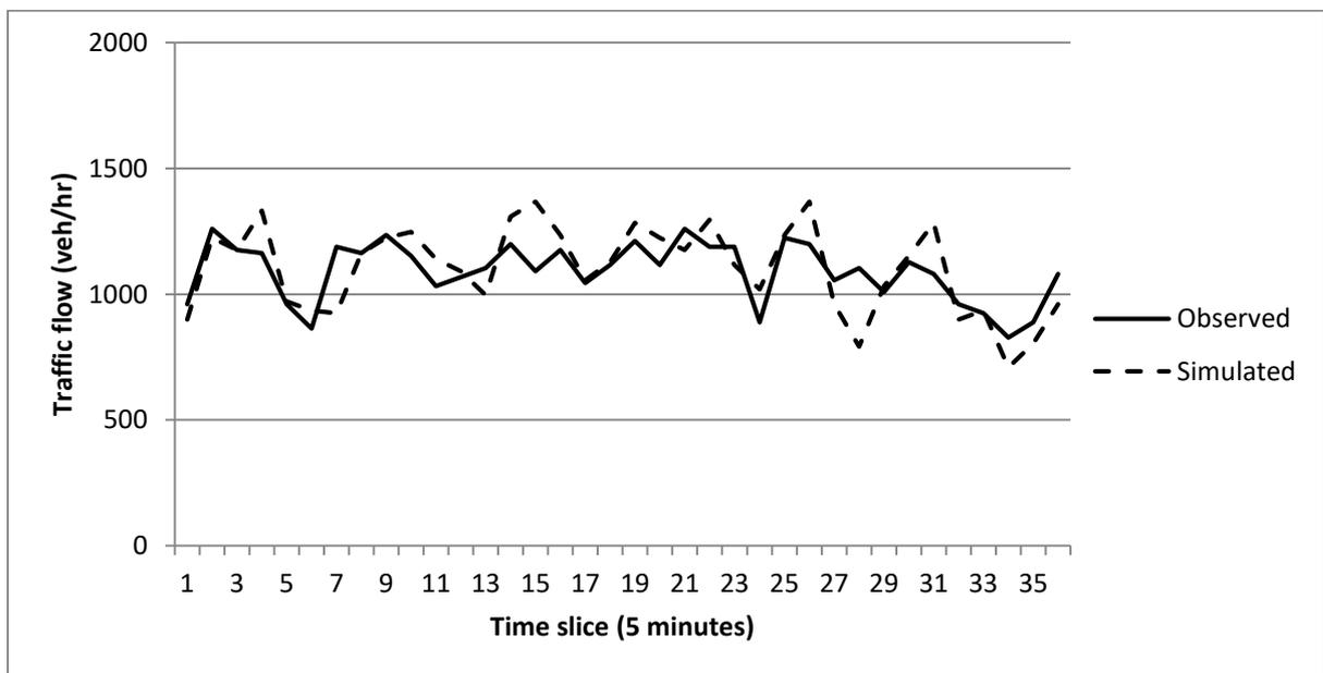
**Figure 7.33: Validation - simulated versus observed traffic flow data (M67, lane closure)**
