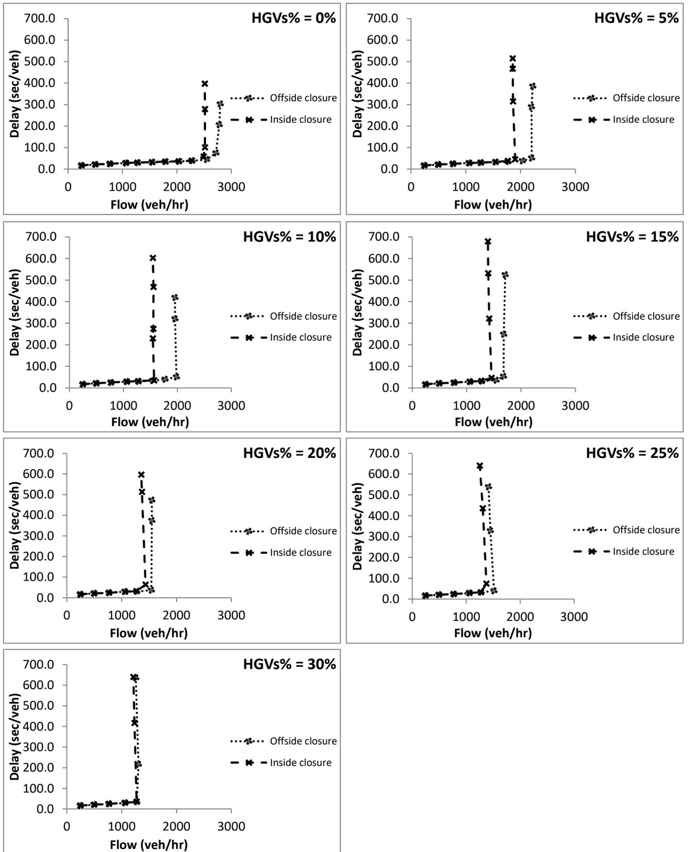
Figure 8.4: Effect of flow rates, HGVs% and TTMSs on average delay for 2-lanes motorway roadwork sections
