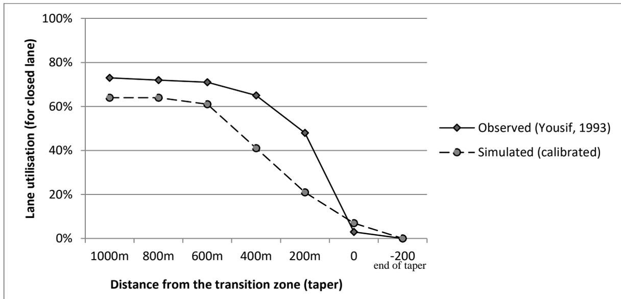
**Figure 7.14: Calibration - simulated (calibrated, N-CD%=95% & D2LC=600m) versus observed lane utilisation data (A4232)**
