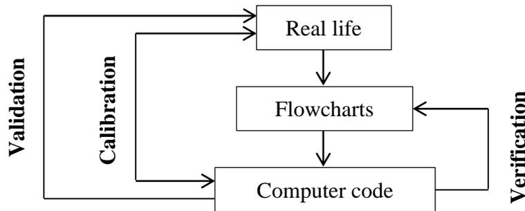
**Figure 7.1: Micro-simulation model verification, calibration and validation processes (May, 1990)**
