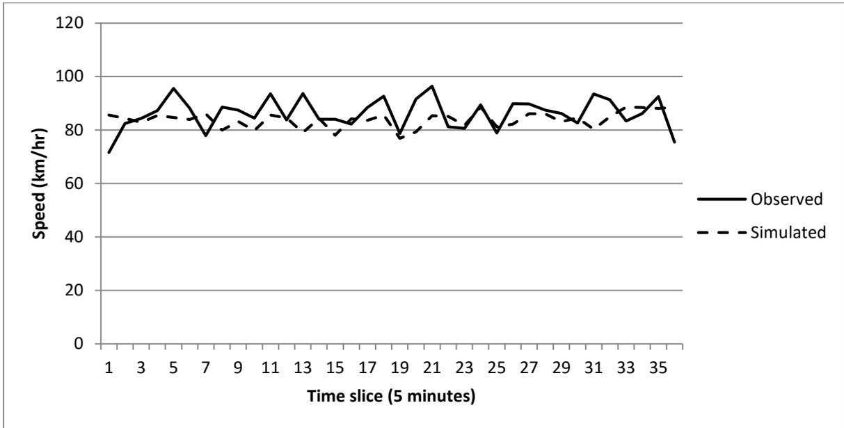
**Figure 7.34: Validation - simulated versus observed speed data (M67, lane closure)**
