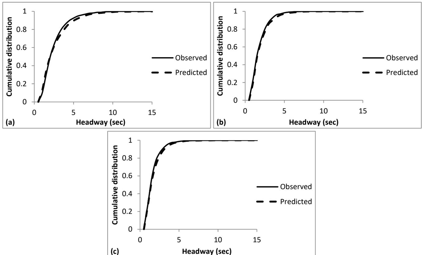
**Figure 3.2: Observed and predicted cumulative headway distributions for Site No. 14 - data set 3 (M42) in (a) lane 1, (b) lane 2 and (c) lane 3 using the shifted negative exponential model**
