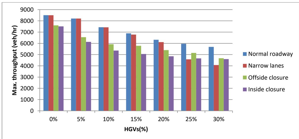
Figure 8.10: Effect of TTMSs on 4-lanes roadworks section capacity for different HGVs%
