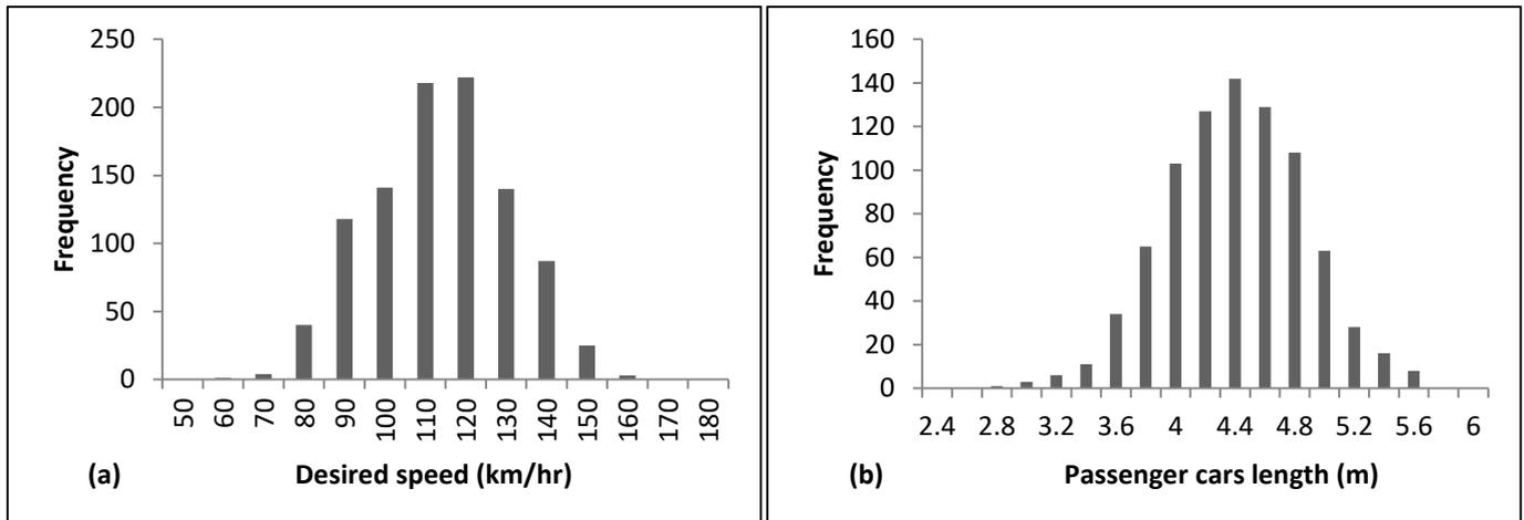
**Figure 7.3: Verification - simulated (a) desired speed distribution (b) passenger cars length distribution**
