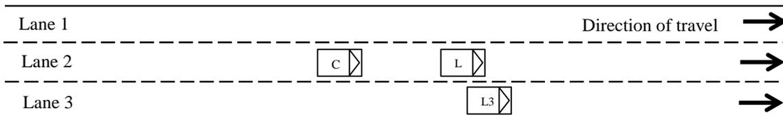
**Figure 6.11: Illustration of the surrounding vehicles that affect the lane-changing process for vehicle C (DLC toward faster lane)**
