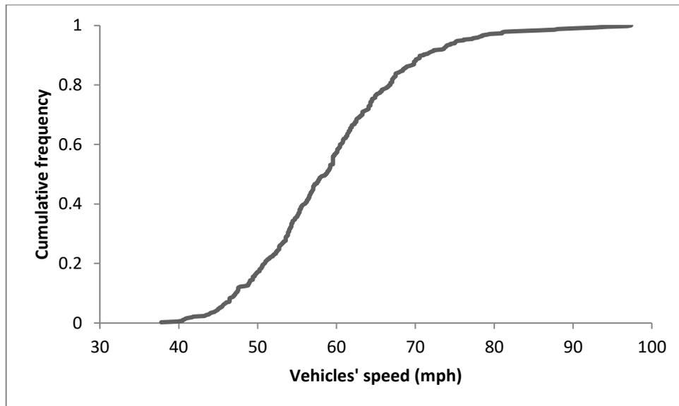
**Figure 3.10: Cumulative distribution for drivers' speeds based on data from the M67 (Site No. 2)**
