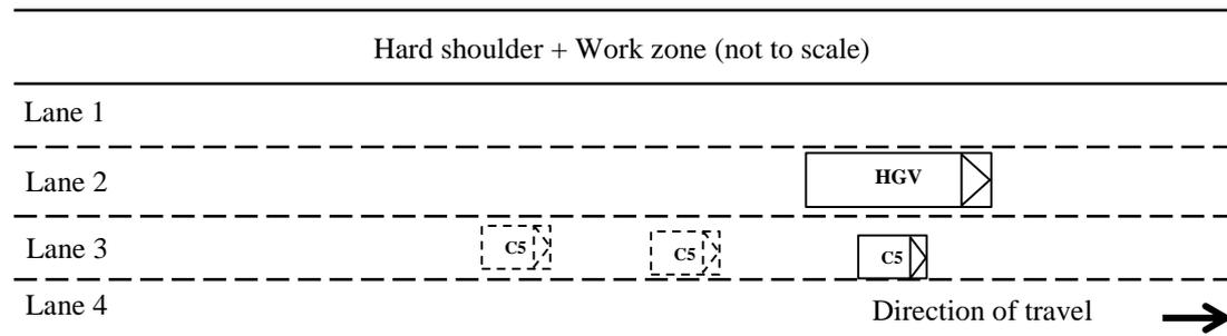
**Figure 4.8: Vehicles’ positions on motorway section with narrow lanes (“repositioning” behaviour)**
