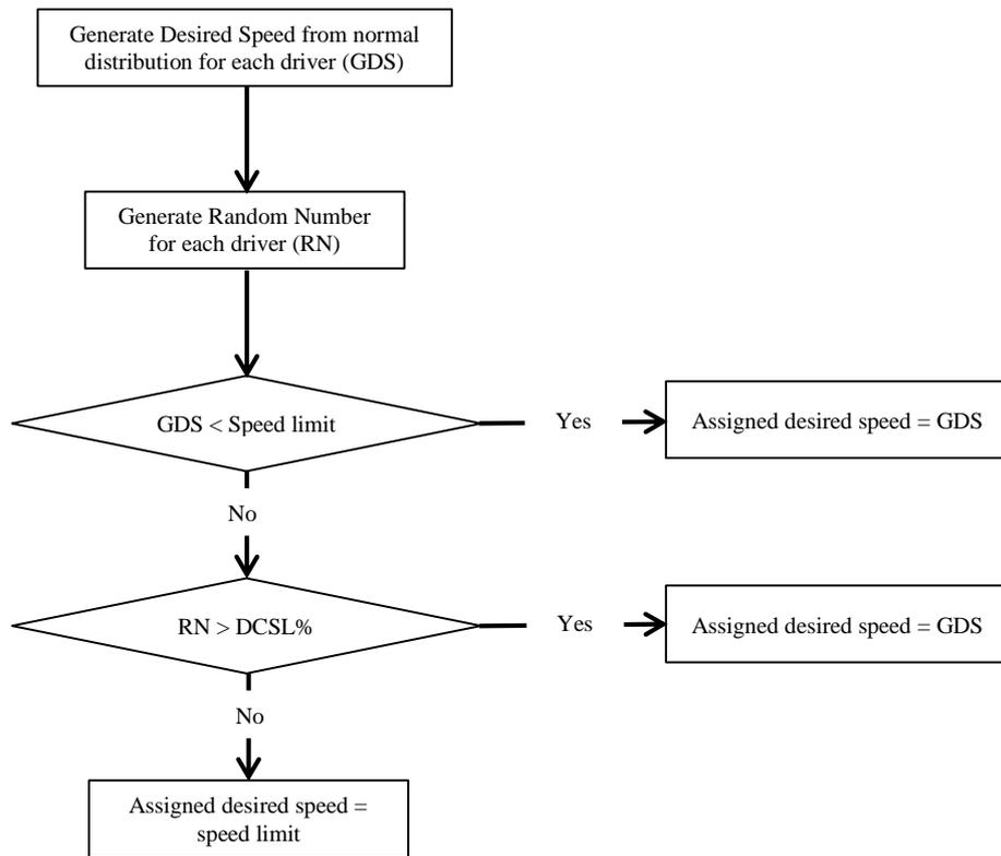
**Figure 6.8: Method of assigning driver's desired speed**
