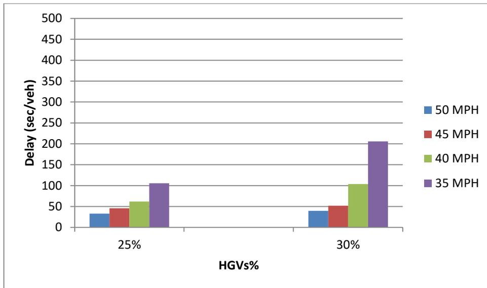
**Figure 8.25: Effect of roadwork speed limits (with 100% complying with speed limits) on 4 lanes section delay (narrow lanes)**
