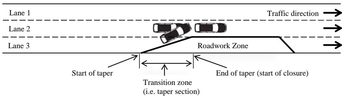
**Figure 5.6: Illustration of vehicles' overlapping on each other in the S-Paramics model (i.e. visual representation at the taper)**
