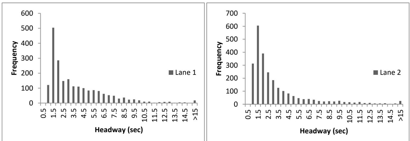
**Figure 7.4: Verification - simulated headway distribution for a 2-lane normal motorway section**
