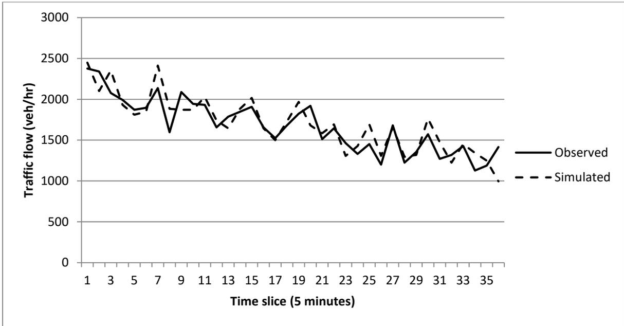
Figure 7.23: Validation - simulated versus observed traffic flow data (M25, data set 2)
