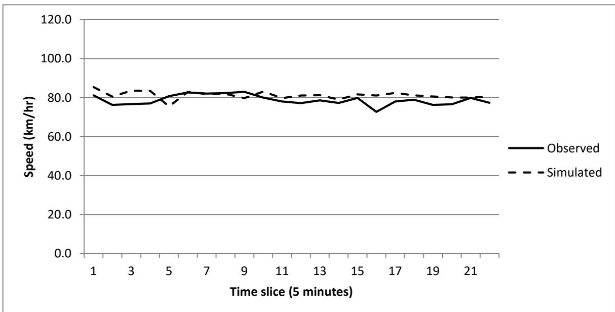
**Figure 7.37: Validation - simulated versus observed speed data (M62, narrow lanes)**
