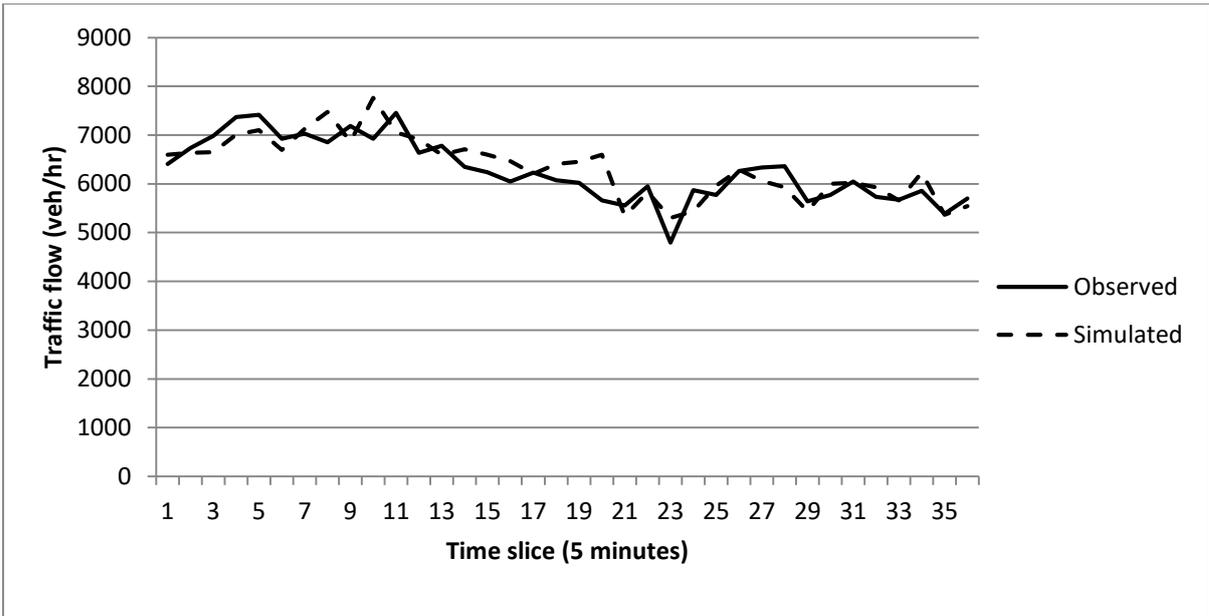
**Figure 7.20: Validation - simulated versus observed traffic flow data (M25, data set 1)**
