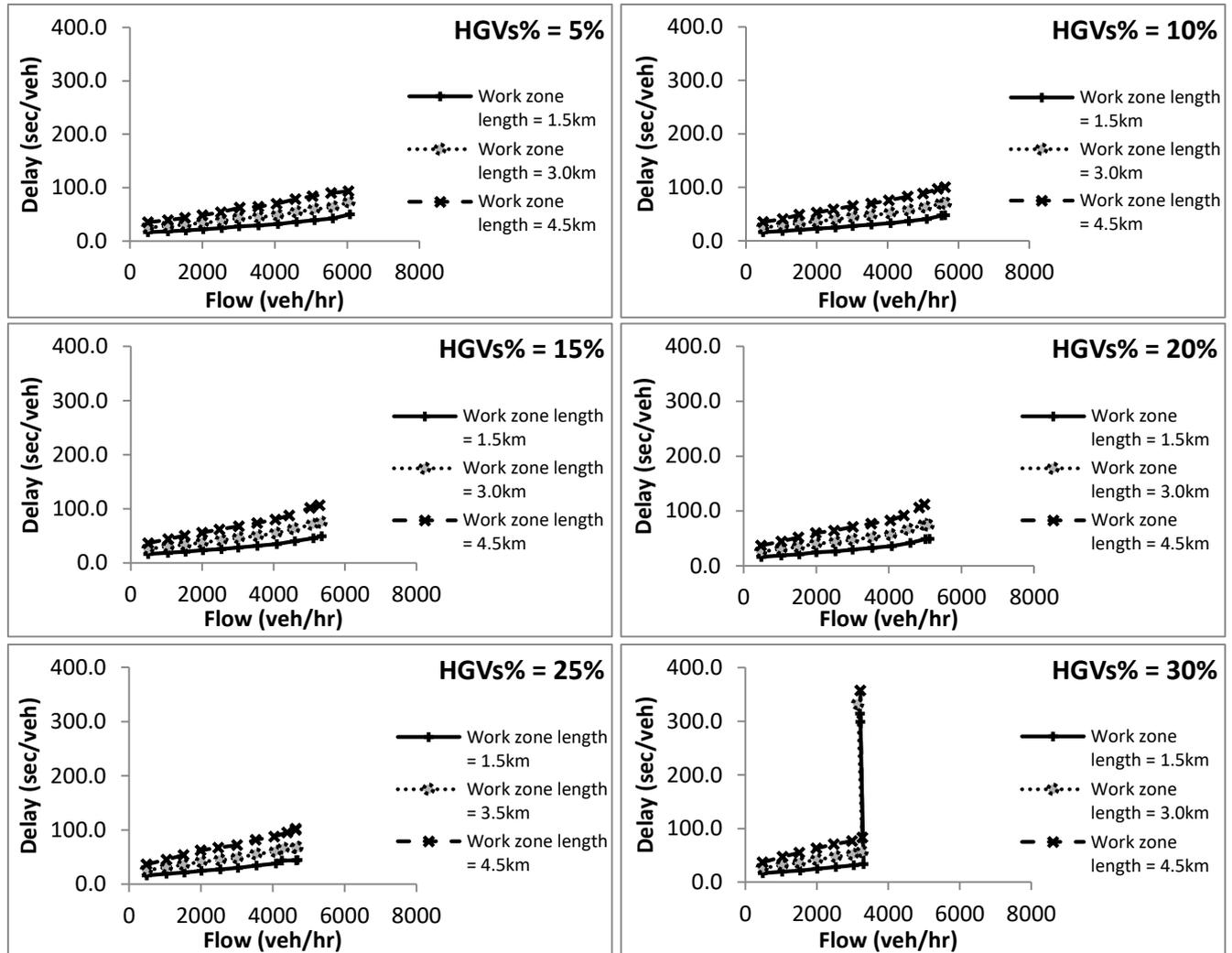
**Figure 8.13: Effect of roadwork zone lengths on average delay for 3-lanes motorway roadwork section with narrow lanes**
