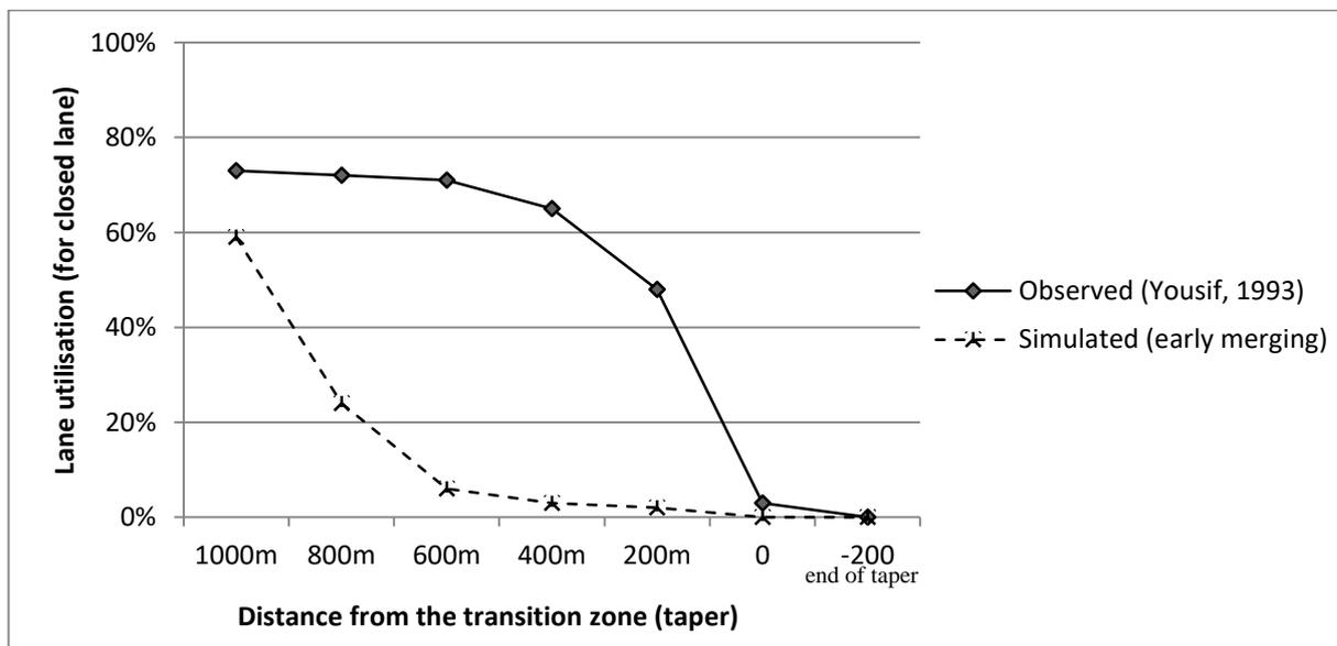
**Figure 7.13: Simulated (early merging) versus observed lane utilisation data from the A4232**
