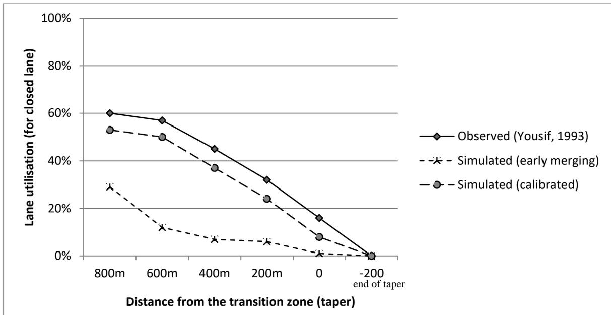
**Figure 7.15: Calibration - simulated (early merging and calibrated, N-CD%=95% & D2LC=600m) versus observed lane utilisation data (M4)**
