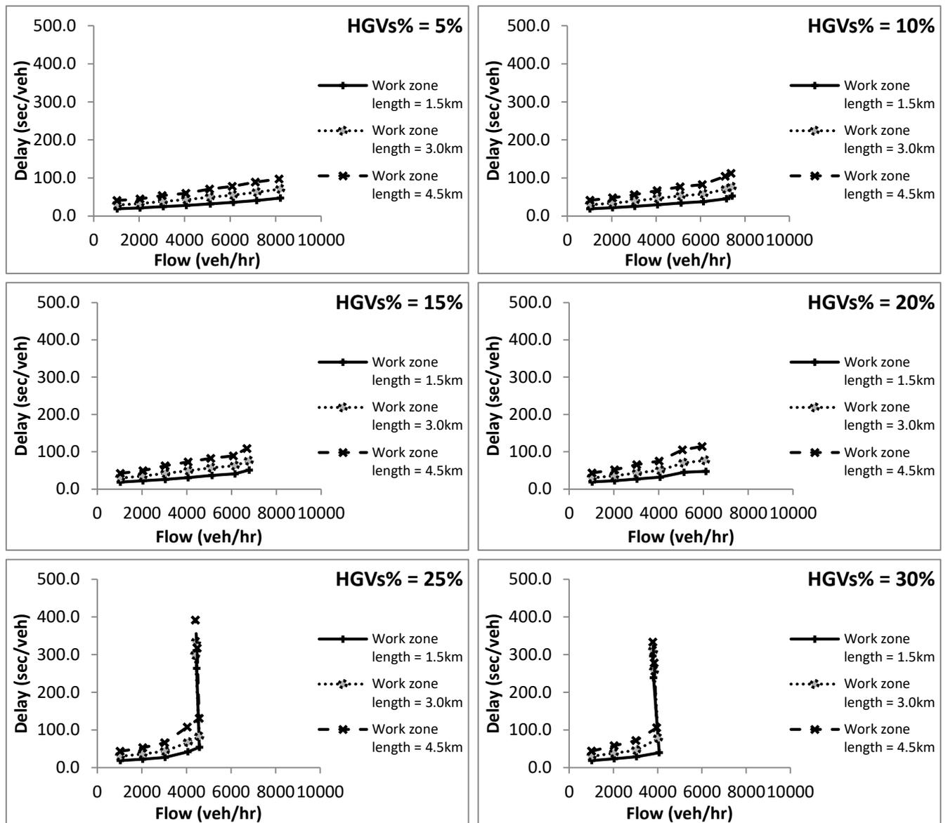
**Figure 8.15: Effect of roadwork zone lengths on average delay for 4-lanes motorway roadwork section with narrow lanes**
