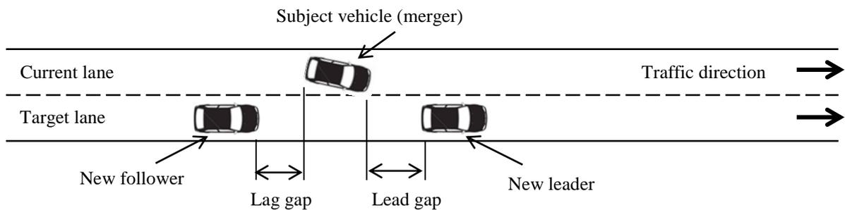
**Figure 2.5: Illustration of lag and lead gaps**
