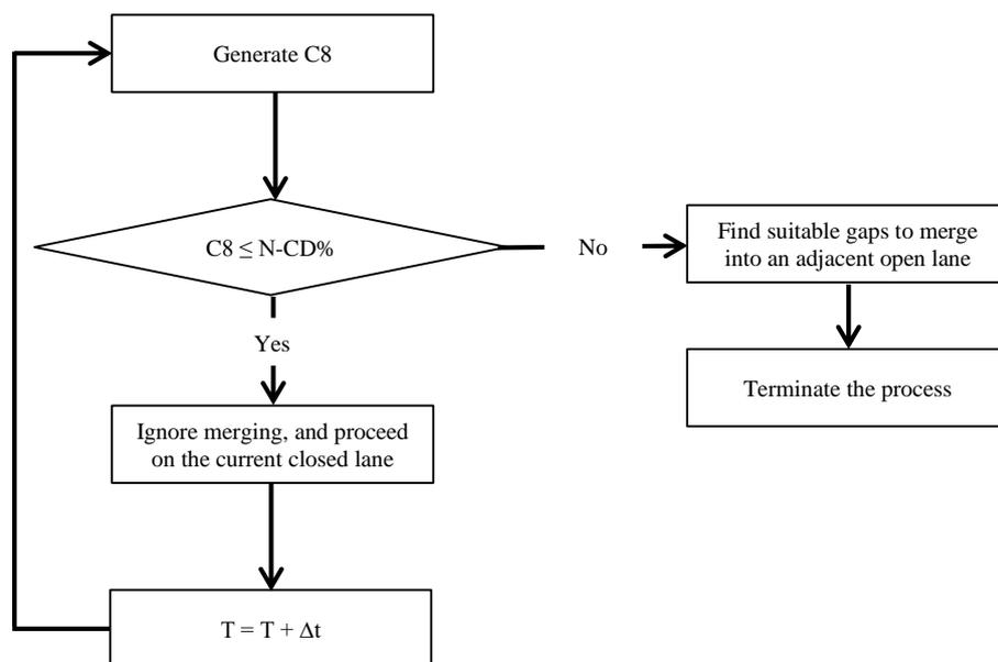
**Figure 7.12: Method of modelling non-complying drivers with merging signs**
