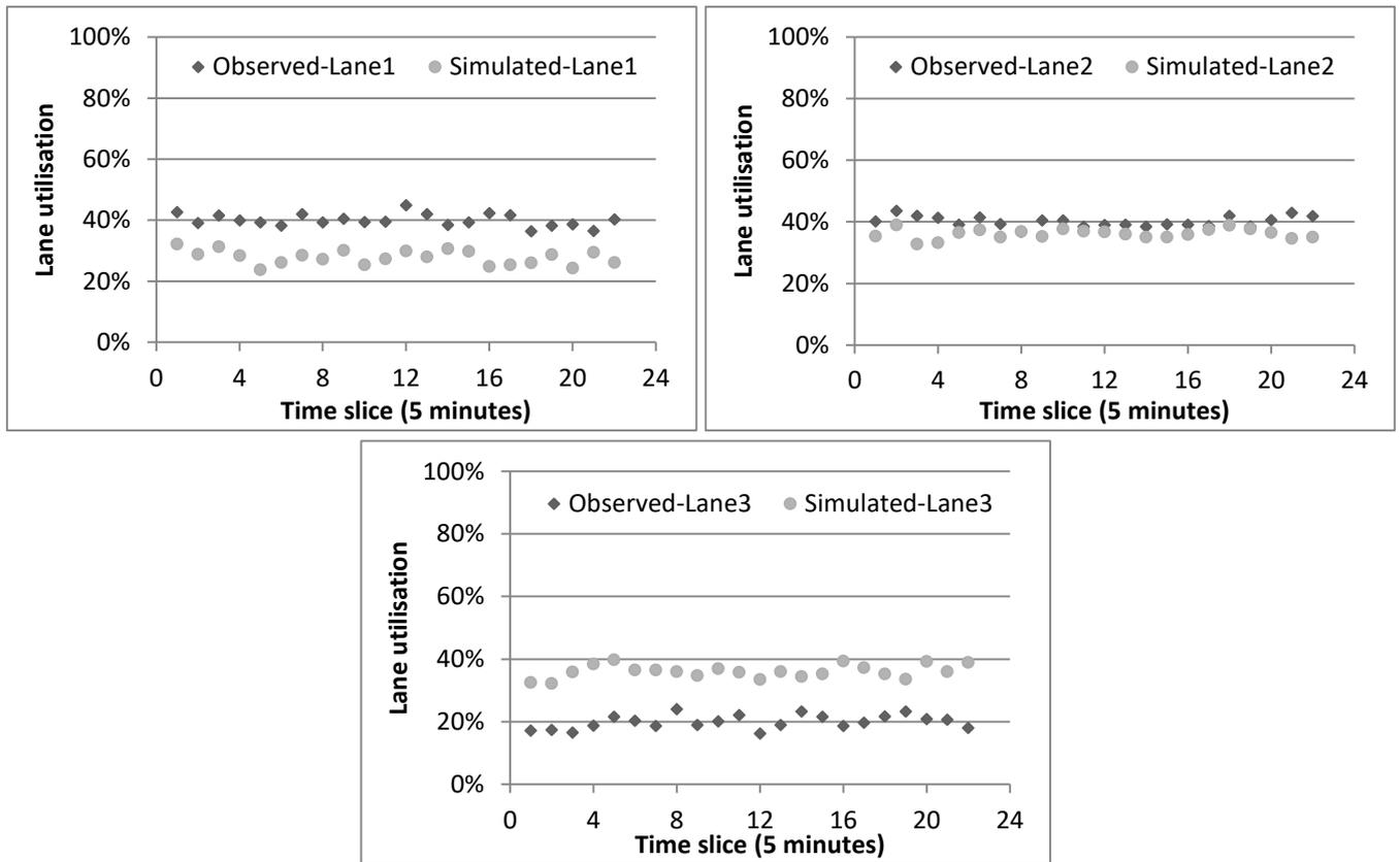
**Figure 7.38: Validation - simulated versus observed lane utilisation data for lanes 1, 2 and 3 on the M62 (narrow lanes)**
