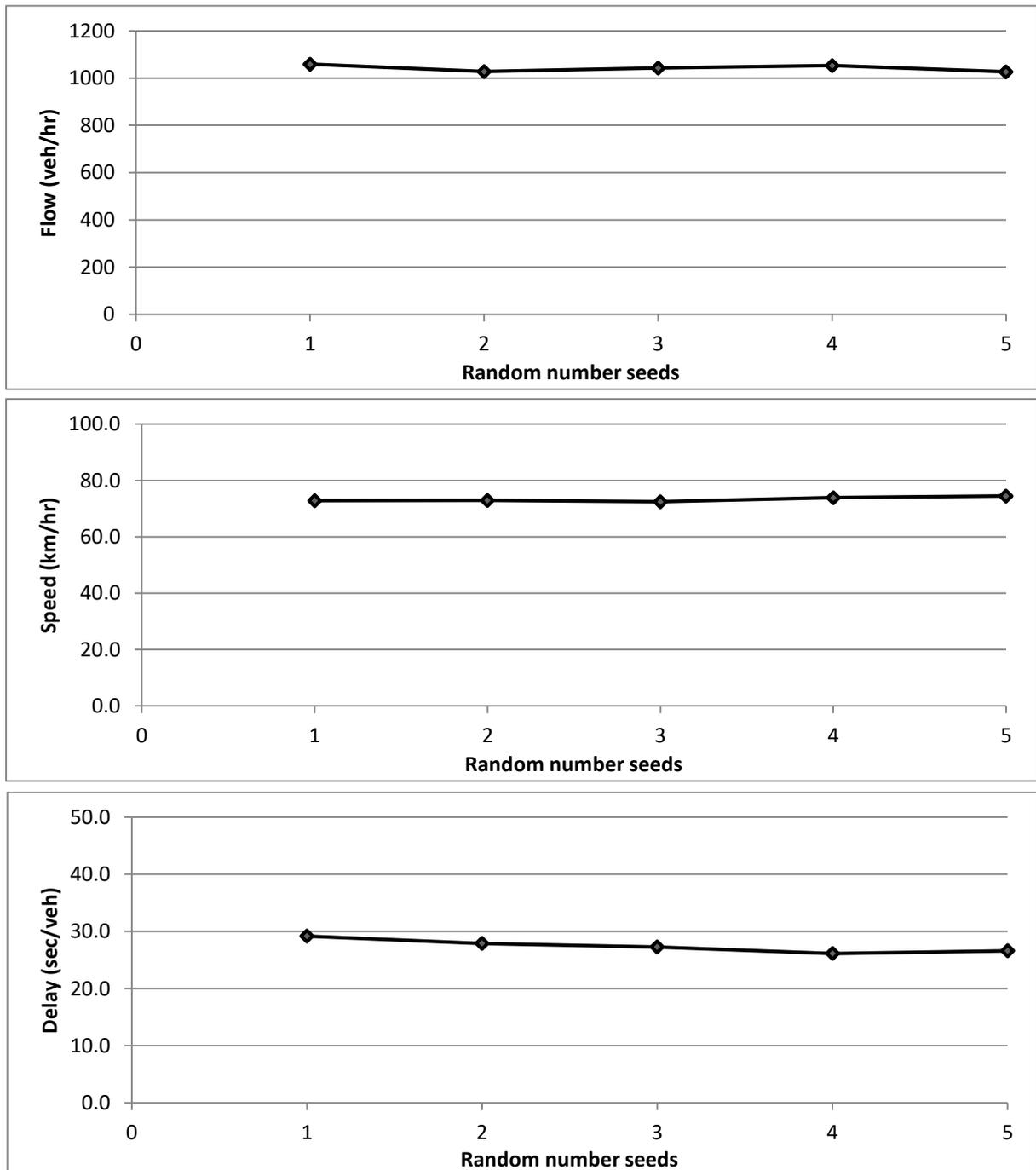
**Figure 7.6: Verification - sensitivity of simulation results for varying random seeds**
