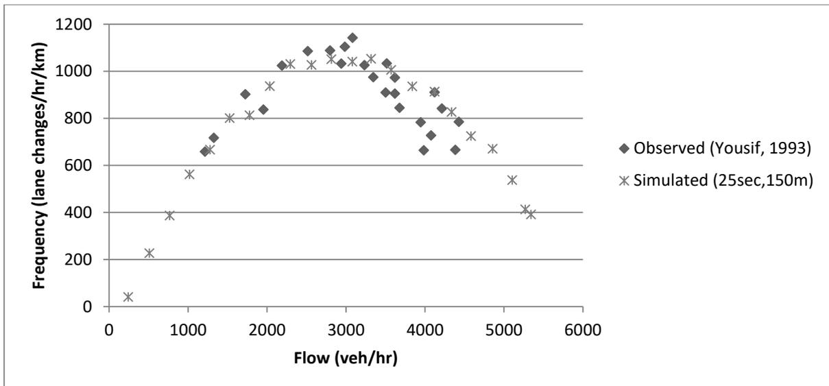
**Figure 7.11: Calibration - simulated versus observed lane changing frequency data for a 3-lanes normal sections**
