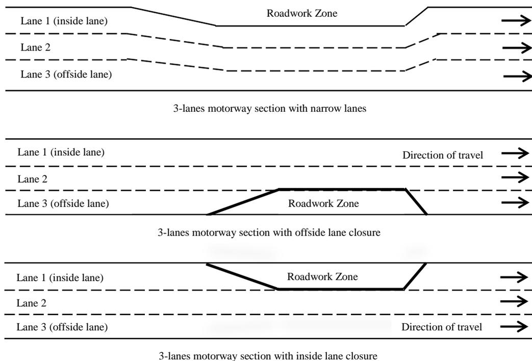
**Figure 8.5: Schematic layouts of the tested 3-lanes motorway roadwork sections**
