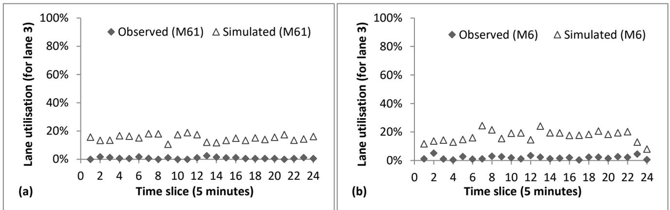
**Figure 5.5: Simulated versus observed lane utilisation data at the start of the transition zone for lane 3 for both data sets (a) M61 and (b) M6**
