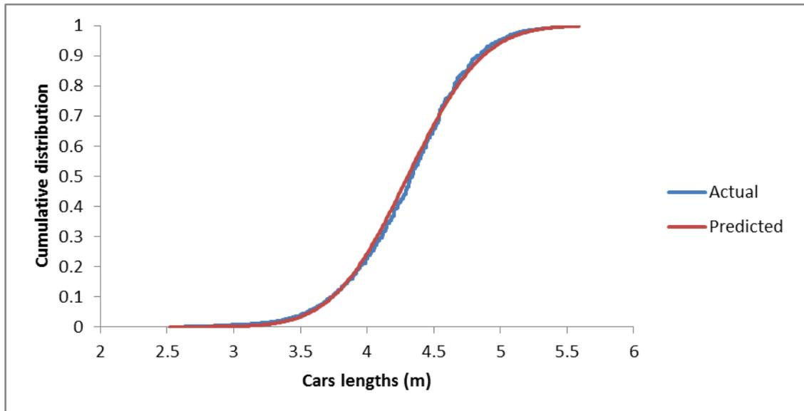
**Figure 6.5: Cumulative distribution for car lengths based on data from the M25**
