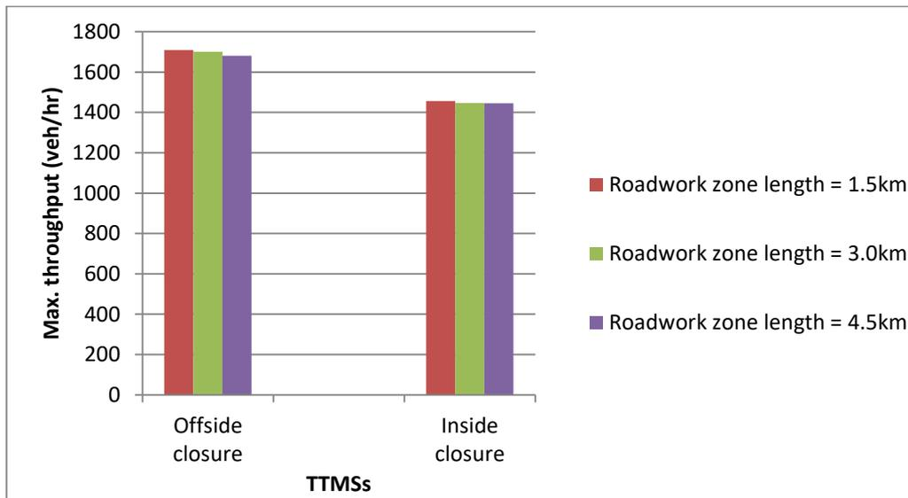
**Figure 8.16: Effect of roadwork zone lengths on 2-lanes section capacity (lane closures)**
