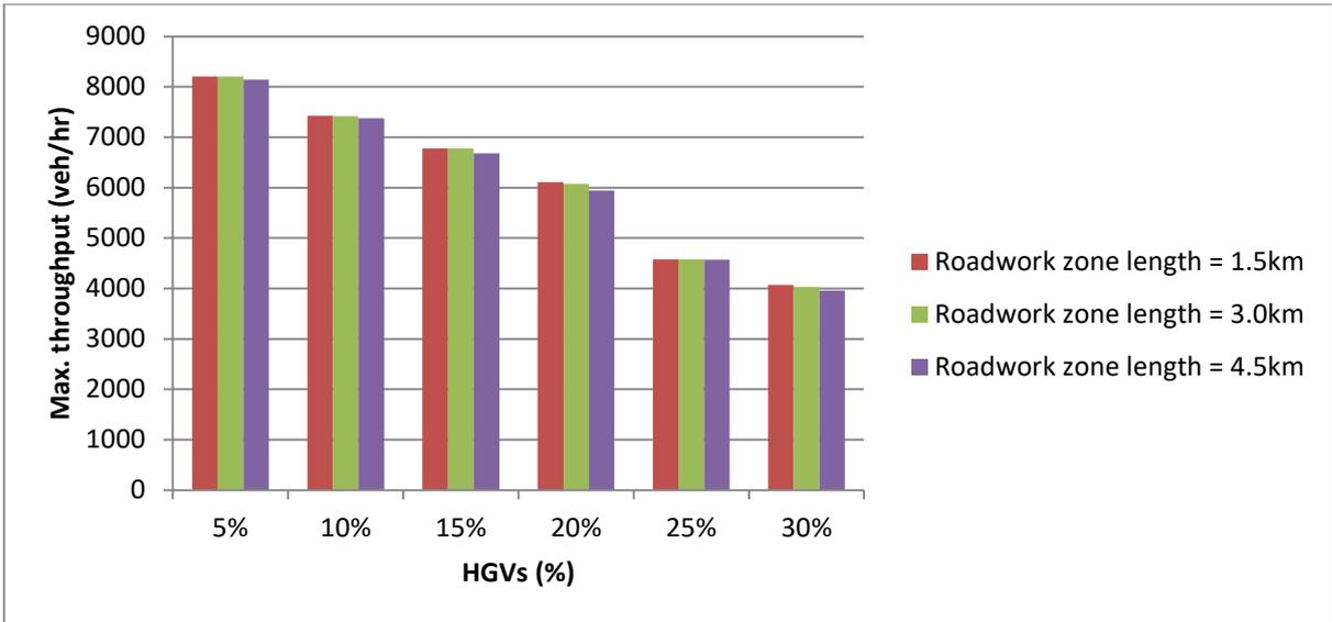
**Figure 8.14: Effect of roadwork zone lengths on 4-lanes section capacity (narrow lanes)**
