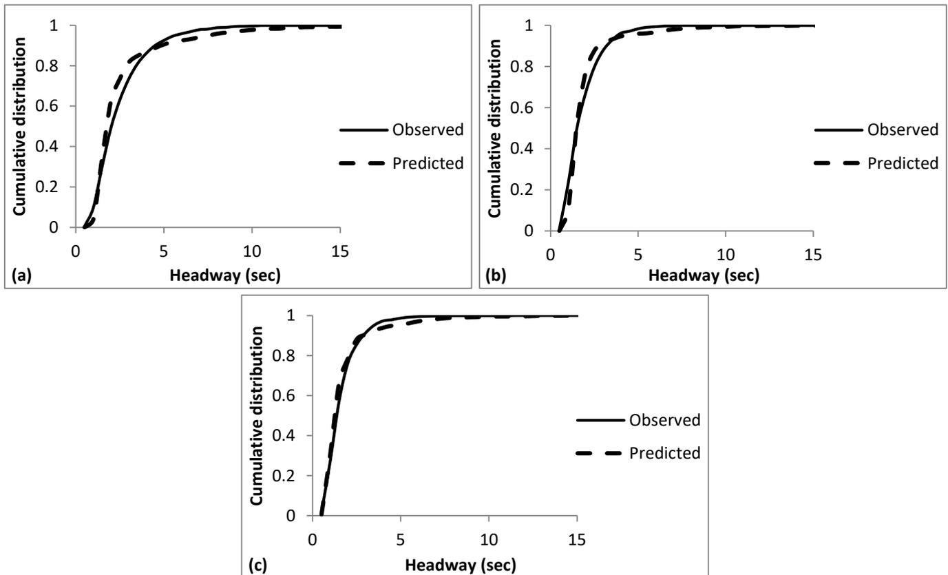
**Figure 3.3: Observed and predicted cumulative headway distributions for Site No. 14 - data set 3 (M42) in (a) lane 1, (b) lane 2 and (c) lane 3 using generalised queuing model**
