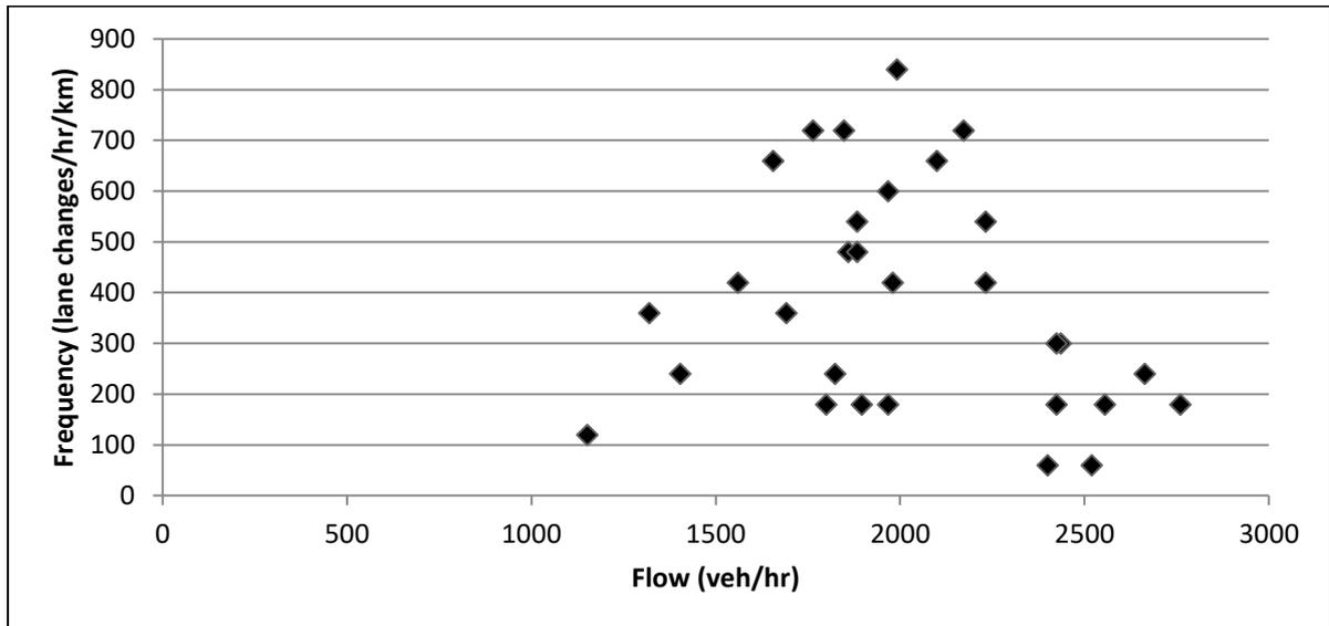
**Figure 3.7: Frequency of lane changing for the M602 (2-lane motorway) (Site No. 10)**
