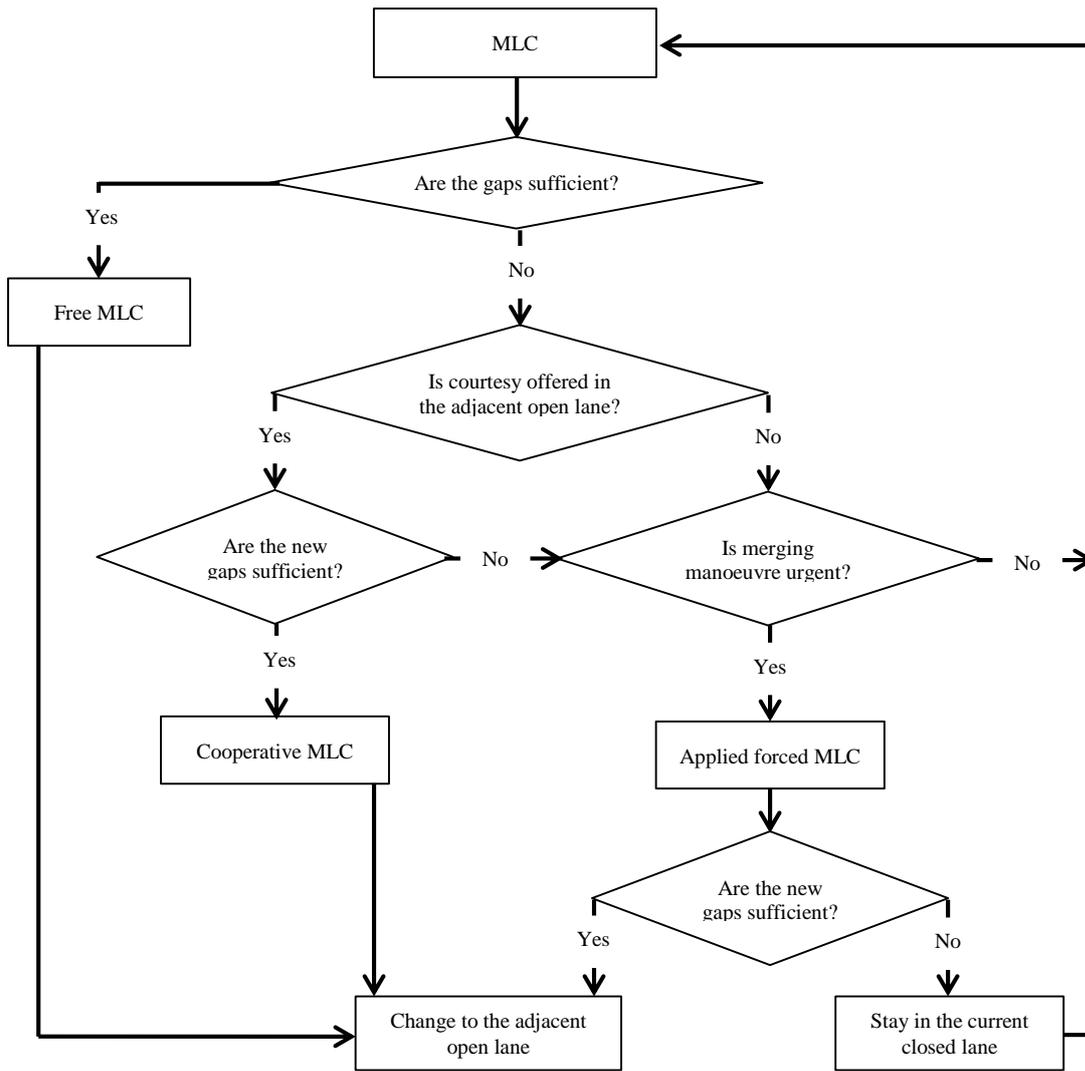
**Figure 6.15: The developed MLC structure**
