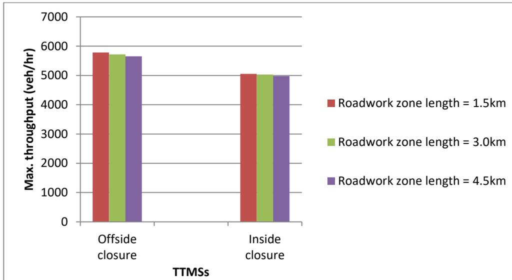
**Figure 8.20: Effect of roadwork zone lengths on 4-lanes section capacity (lane closures)**
