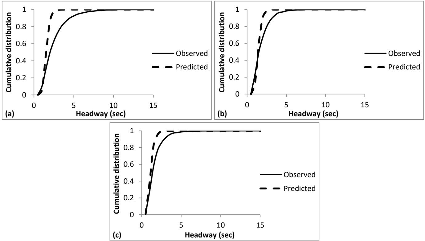
**Figure 3.4: Observed and predicted cumulative headway distributions for Site No. 14 - data set 3 (M42) in (a) lane 1, (b) lane 2 and (c) lane 3 using the lognormal model**
