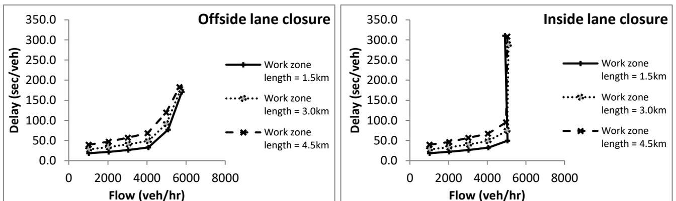
**Figure 8.21: Effect of roadwork zone lengths on average delay for 4-lanes motorway roadwork section with offside/inside lane closure**
