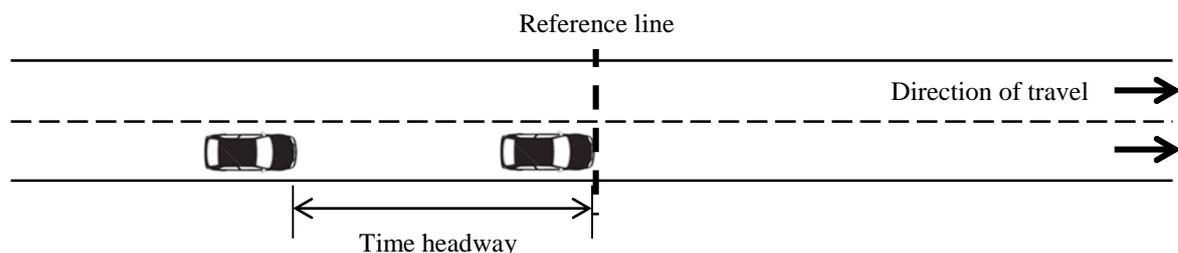
**Figure 2.7: Illustration of time headway**
