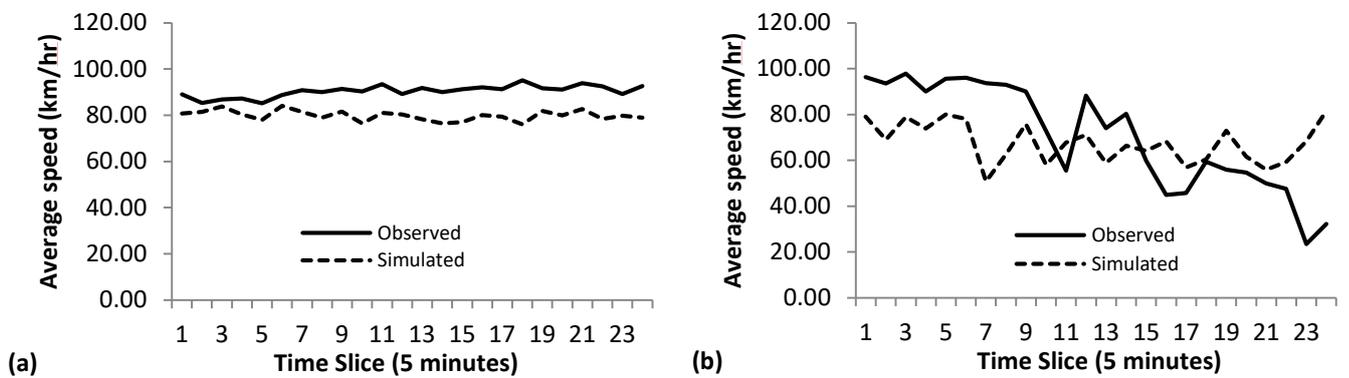
Figure 5.2: Simulated versus observed speed based on data from (a) M61 and (b) M6
