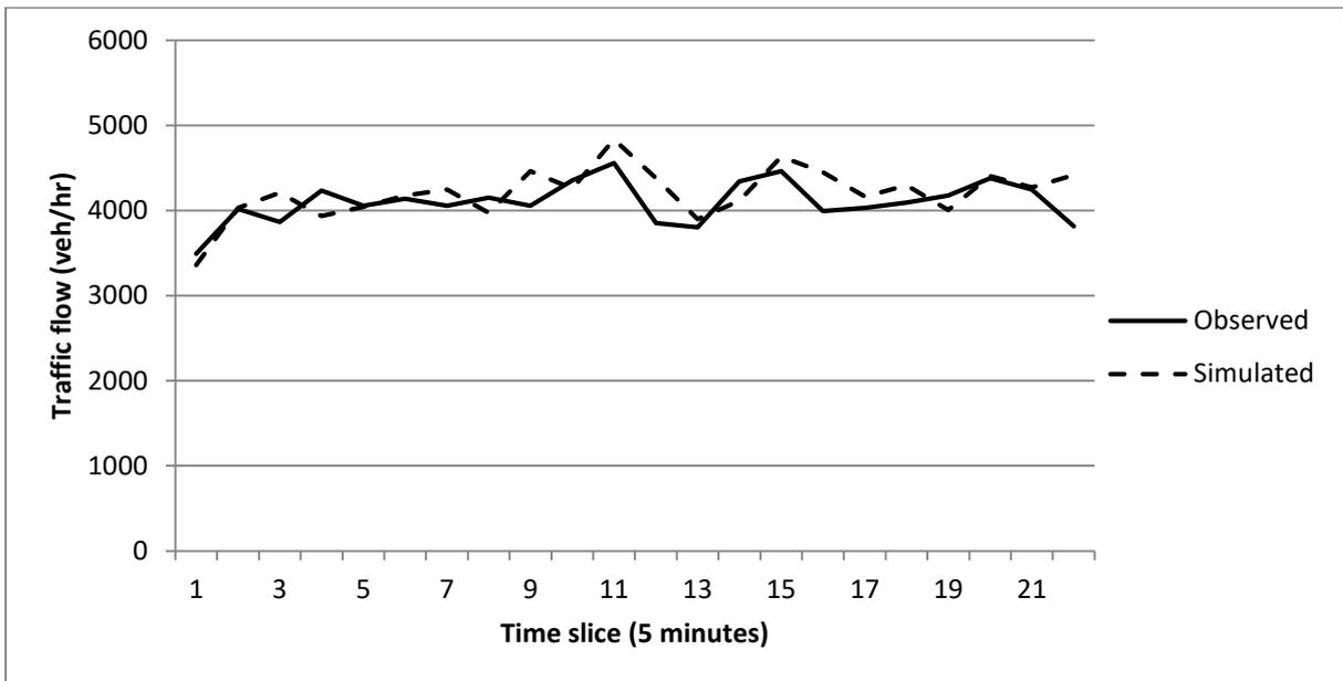
**Figure 7.36: Validation - simulated versus observed traffic flow data (M62, narrow lanes)**
