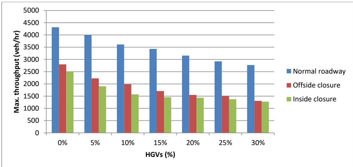
**Figure 8.3: Effect of TTMSs on 2-lanes roadwork sections capacity for different HGVs%**
