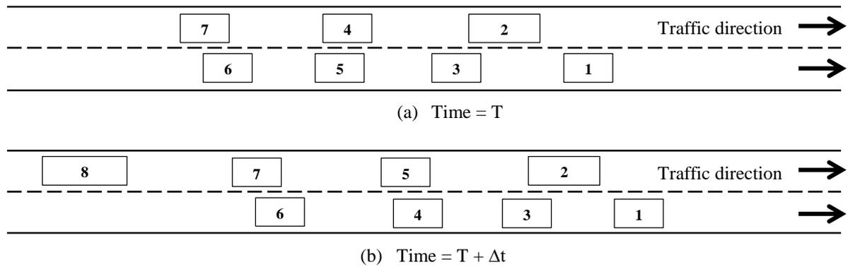
**Figure 6.2: (a) Numbering and (b) renumbering the vehicles in the system at each  $\Delta t$**
