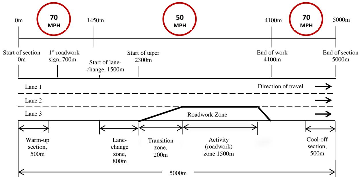
**Figure 8.1: Typical layout used in testing the effect of different TTMSs**
