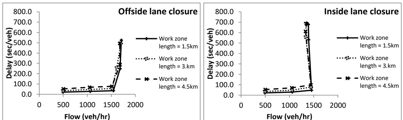
**Figure 8.17: Effect of roadwork zone lengths on average delay for 2-lanes motorway roadwork section with offside/inside lane closure**
