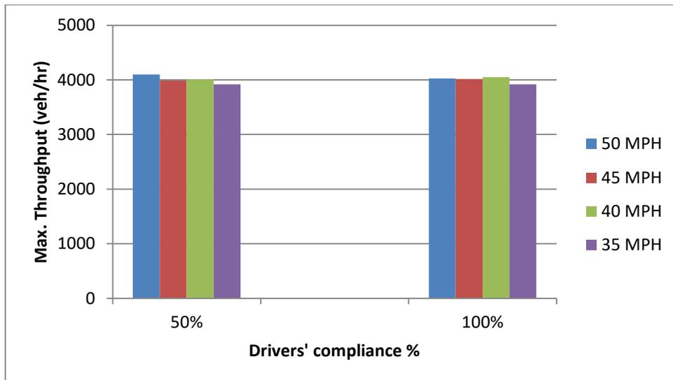
**Figure 8.26: Effect of roadwork speed limits on 3-lanes section capacity (lane closure)**
