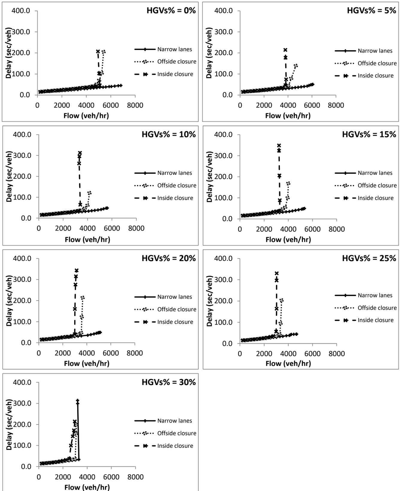
Figure 8.7: Effect of flow rates, HGVs% and TTMSs on average delay for 3-lanes motorway roadwork sections
