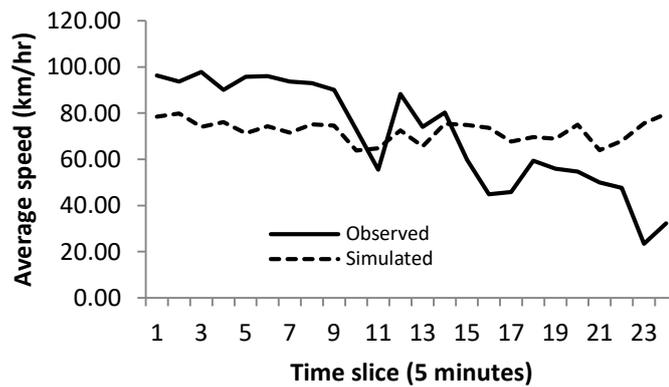
Figure 5.3: Validation - simulated versus observed speed based on data from the M6
