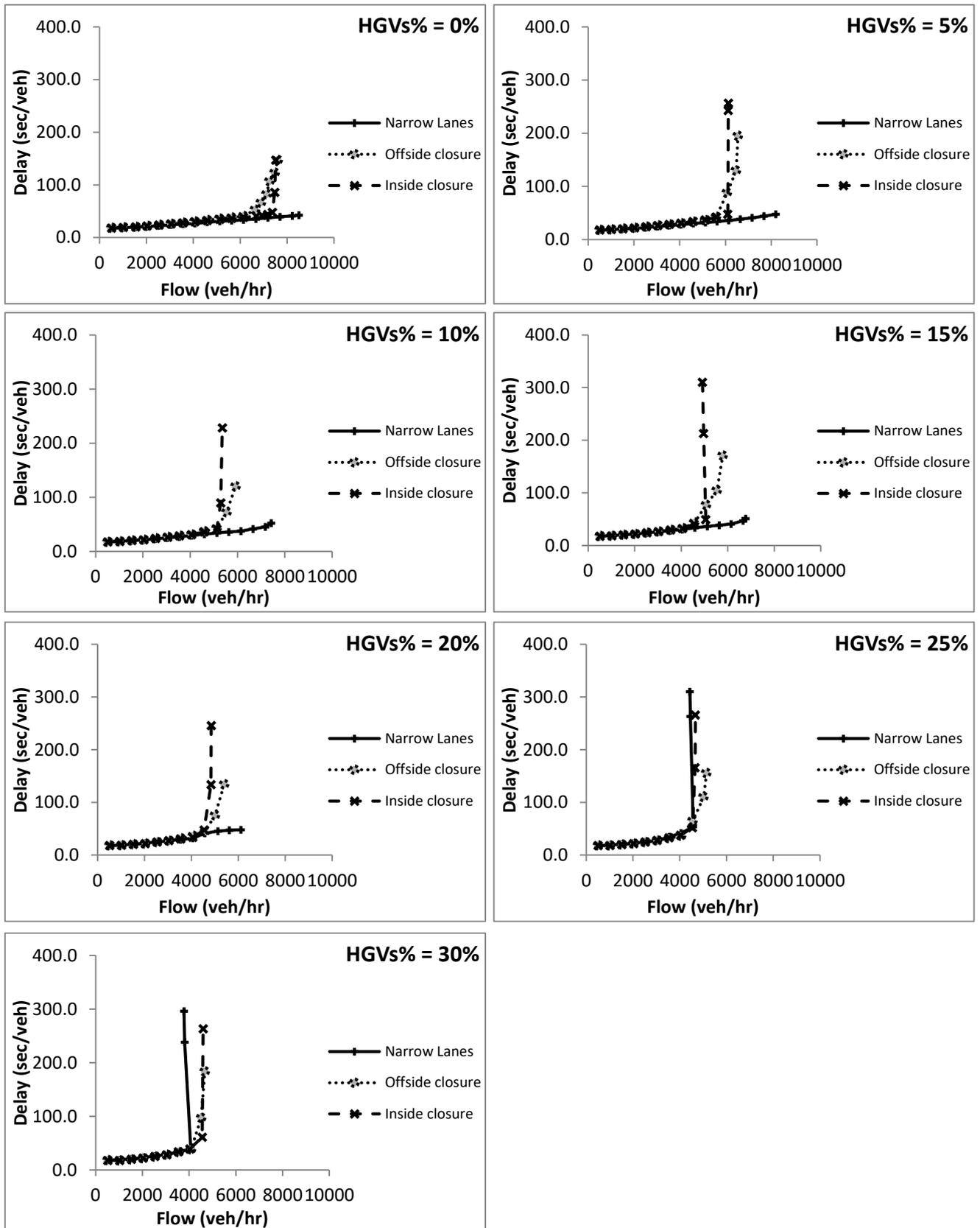
Figure 8.11: Effect of flow rates, HGVs% and TTMSs on average delay for 4-lanes motorway roadwork sections
