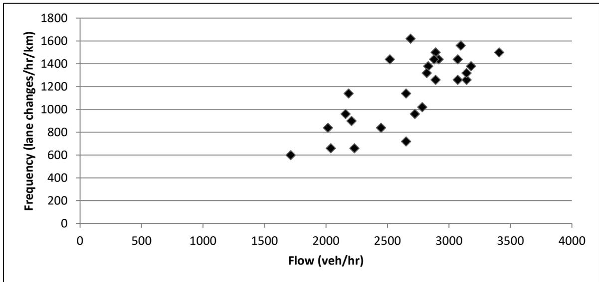
**Figure 3.6: Frequency of lane changing for the M60 (3-lane motorway) (Site No. 8)**
