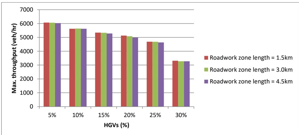
**Figure 8.12: Effect of roadwork zone lengths on 3-lanes section capacity (narrow lanes)**
