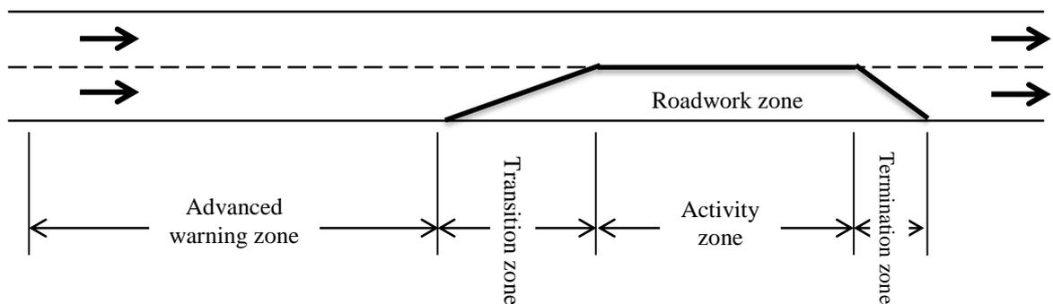
**Figure 2.1: Illustration of motorway roadwork site layout operated by lane closure**
