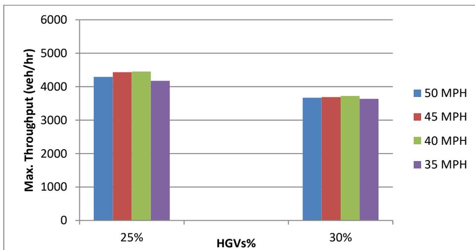
**Figure 8.22: Effect of roadwork speed limits (with 50% complying with speed limits) on 4 lanes section capacity (narrow lanes)**
