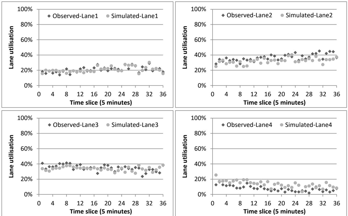
**Figure 7.25: Validation - simulated versus observed lane utilisation data for lanes 1, 2, 3 and 4 on the M25 (data set 2)**
