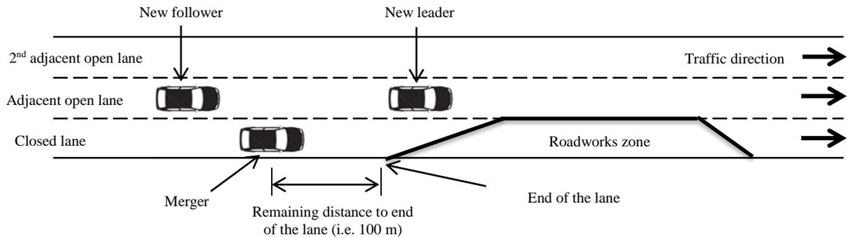
**Figure 6.16: Illustration of the urgency of merging manoeuvre**
