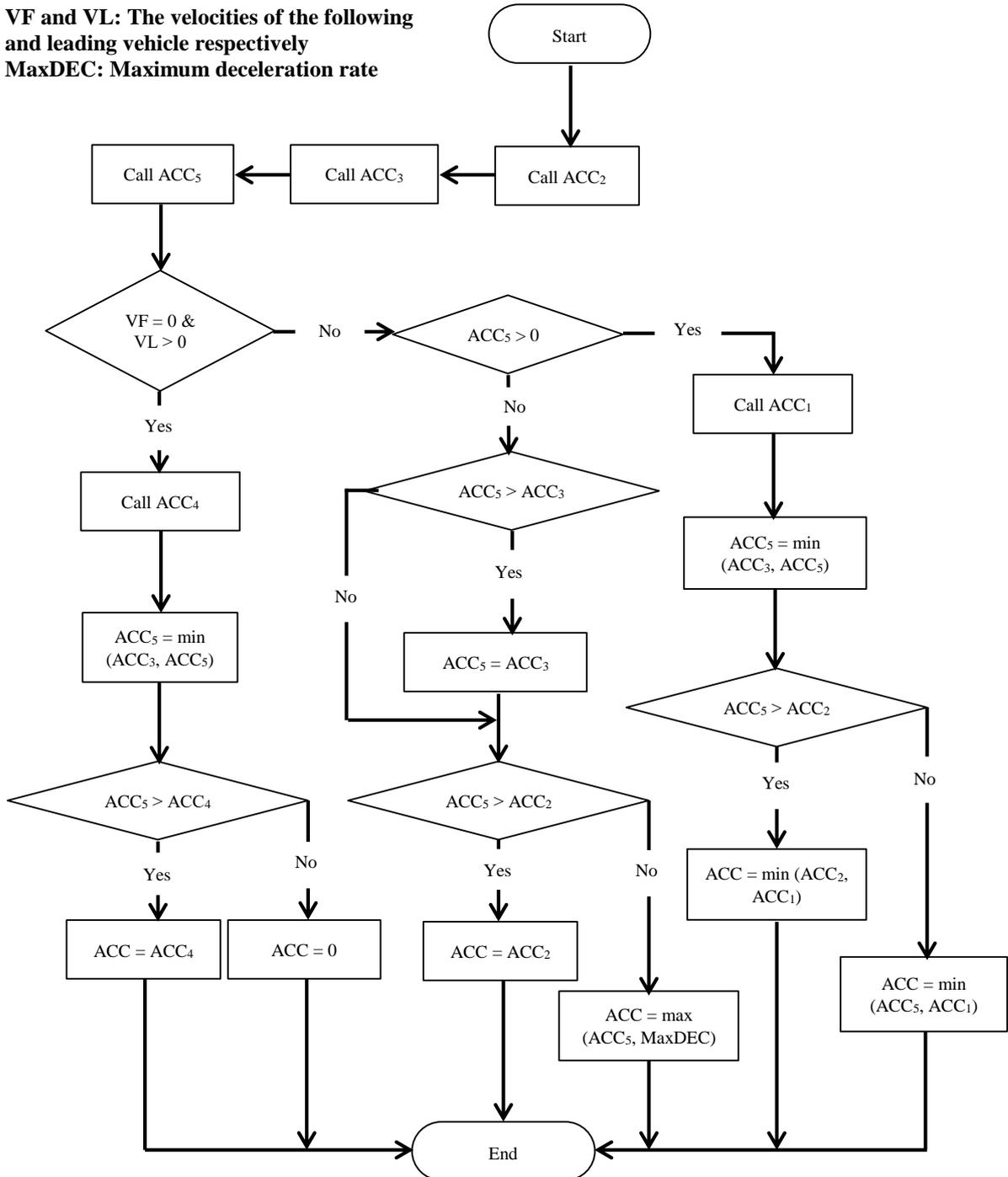
**Figure 6.10: The car-following sub-model flow chart**
