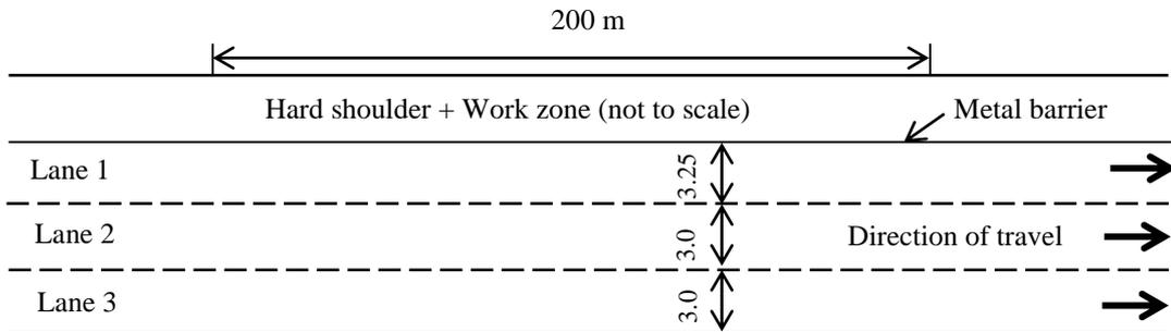
**Figure 4.3: Schematic layout of the M62 roadwork site**
