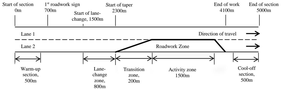
**Figure 7.32: Illustration of the simulated section layout (based on the M67 site)**
