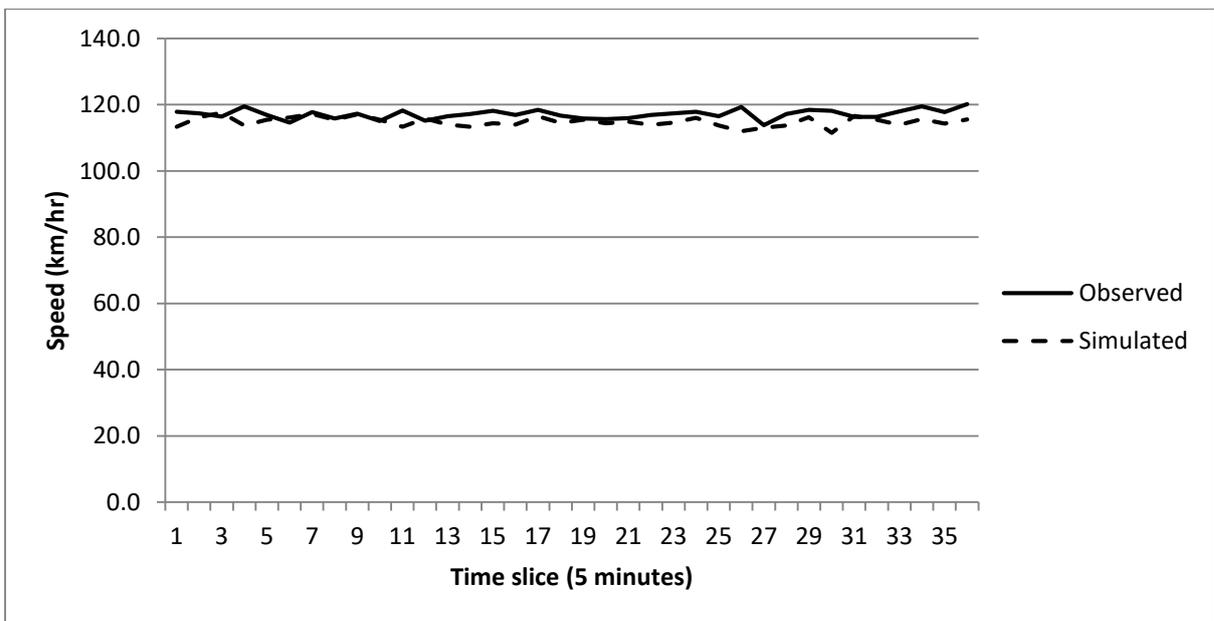
Figure 7.24: Validation - simulated versus observed speed data (M25, data set 2)
