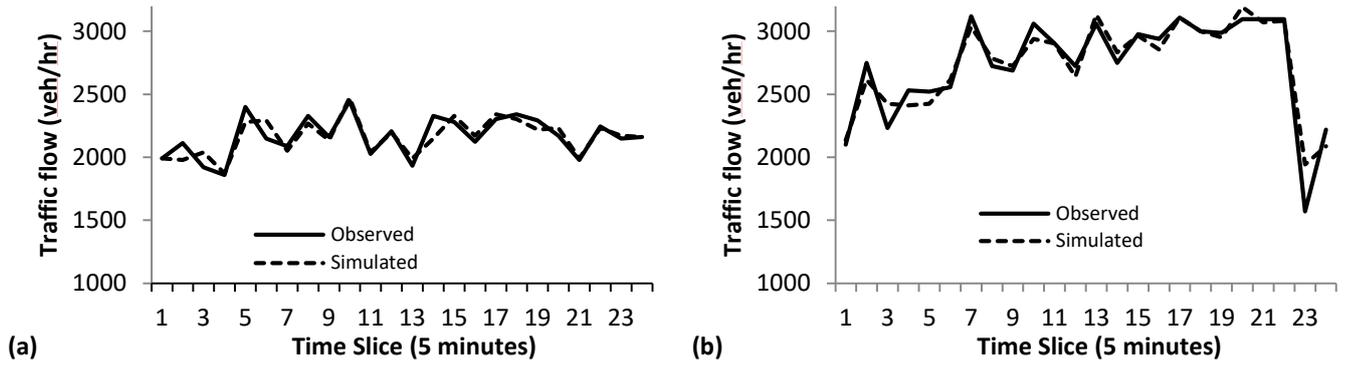
Figure 5.1: Simulated versus observed flow based on data from (a) M61 and (b) M6
