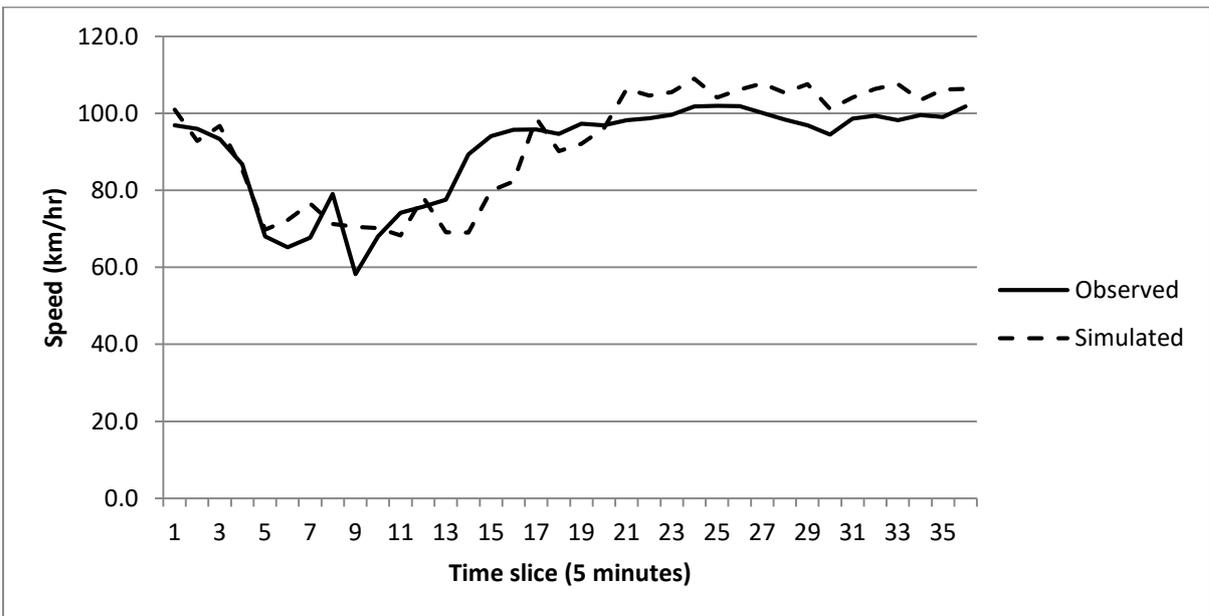
**Figure 7.21: Validation - simulated versus observed speed data (M25, data set 1)**
