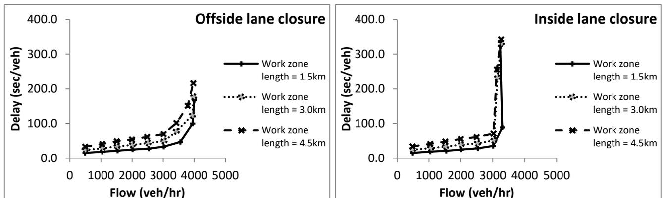
**Figure 8.19: Effect of roadwork zone lengths on average delay for 3-lanes motorway roadwork section with offside/inside lane closure**
