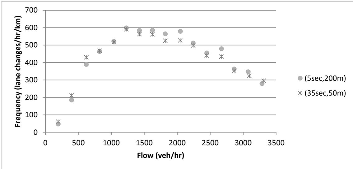
**Figure 7.8: Calibration - simulated lane changing frequency for a 2-lanes normal motorway section under arbitrary values of THRT and THRD**
