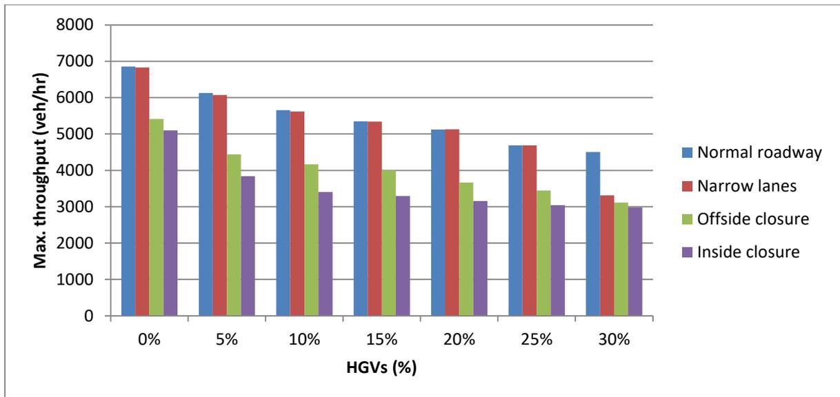
**Figure 8.6: Effect of TTMSs on 3-lanes roadworks section capacity for different HGVs%**
