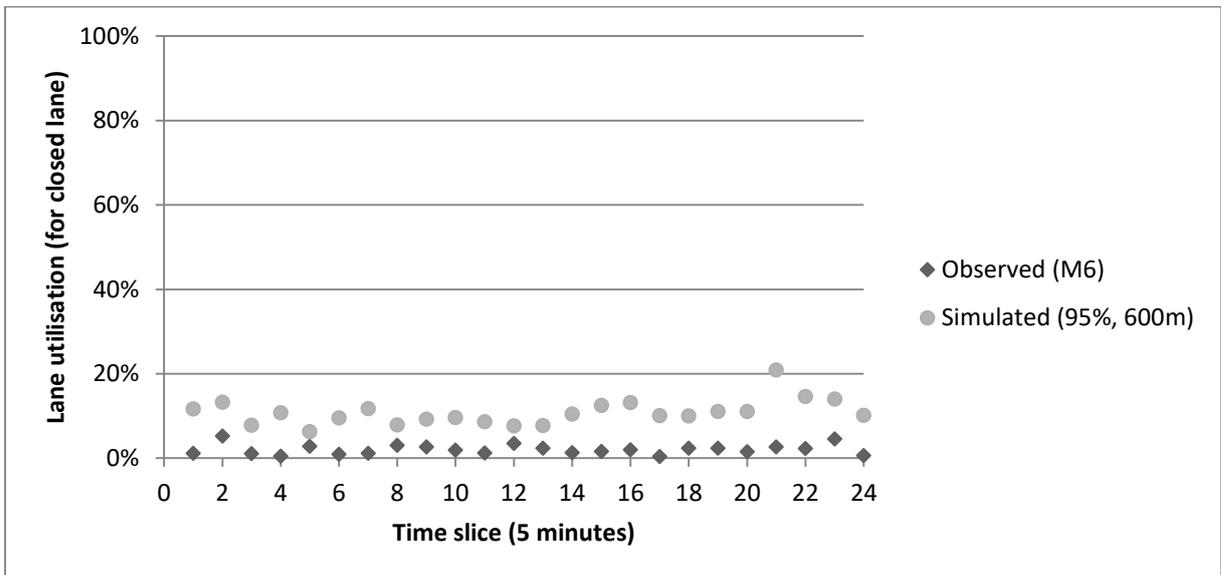
**Figure 7.16: Calibration - simulated (N-CD%=95% & D2LC=600m) versus observed lane utilisation data (M6) at the start of the transition section**
