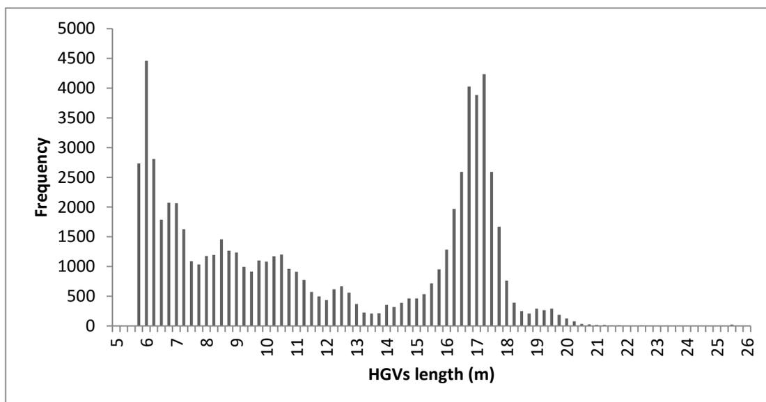
**Figure 6.4: Distribution of HGV lengths based on data from the M25 (Site No. 13)**
