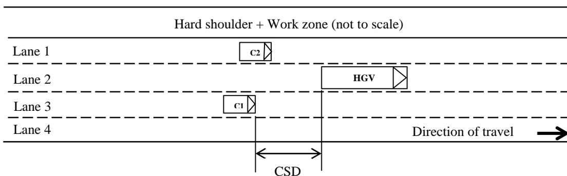
**Figure 4.4: Vehicles’ positions on motorway sections with narrow lanes (“avoiding” case)**
