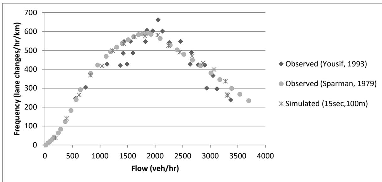
**Figure 7.10: Calibration - simulated versus two sets of observed lane changing frequency data for a 2-lanes normal sections**
