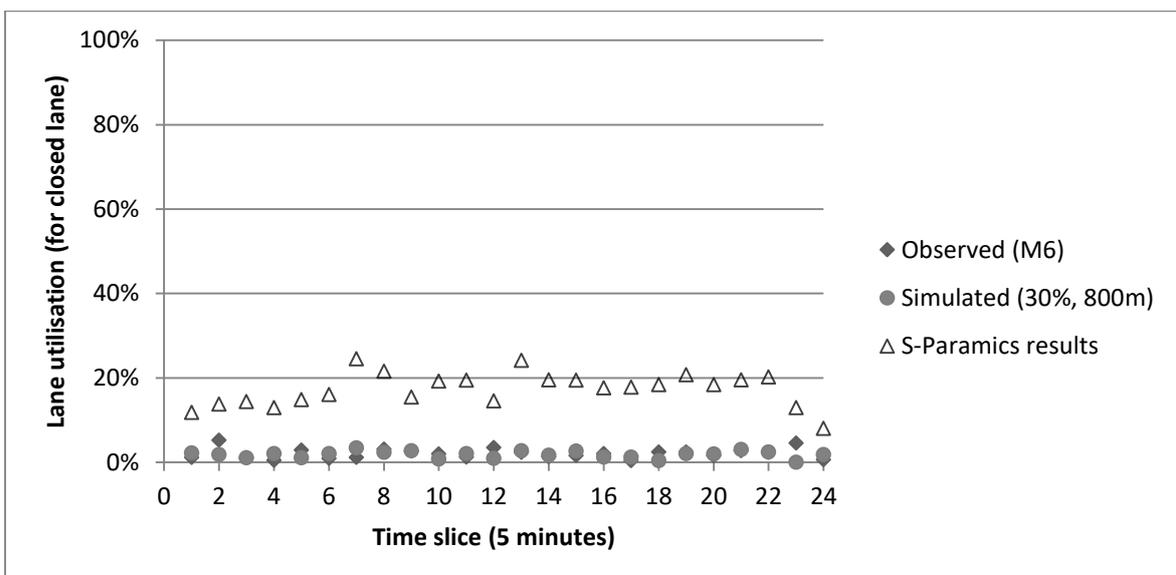
**Figure 7.17: Calibration - simulated (N-CD%=30% & D2LC=800m) versus observed lane utilisation data (M6) at the start of the transition section**
