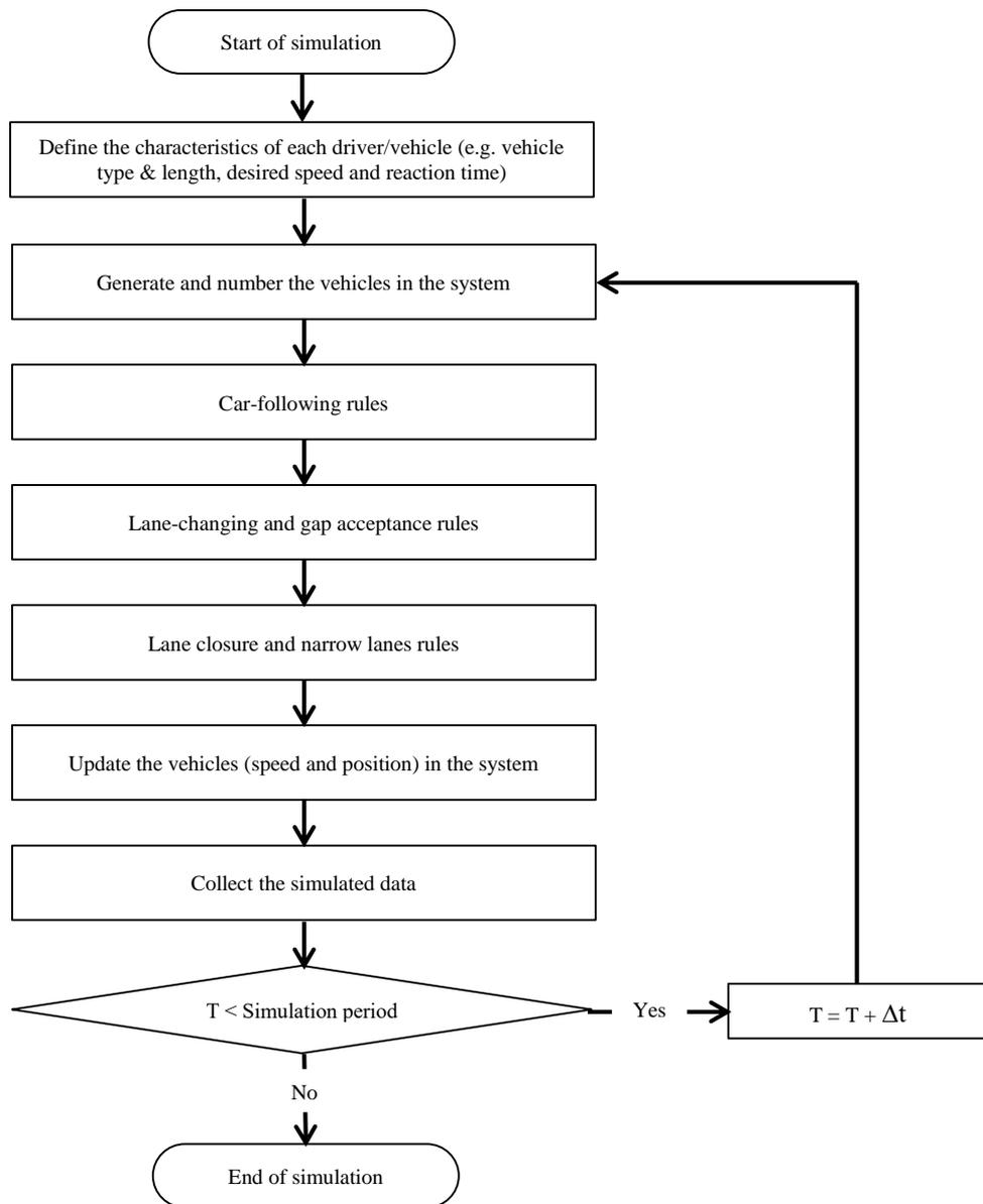
**Figure 6.1: General structure of the newly developed micro-simulation model**
