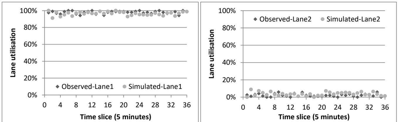
**Figure 7.35: Validation - simulated versus observed lane utilisation data for lanes 1 and 2 on the M67 (lane closure)**
