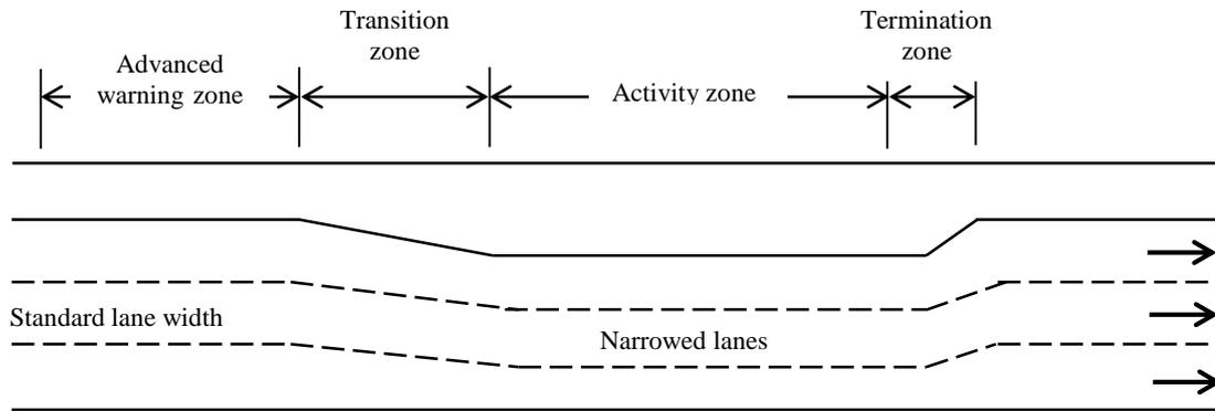
**Figure 4.1: Illustration of motorway roadwork site layout operated by narrowing lanes**
