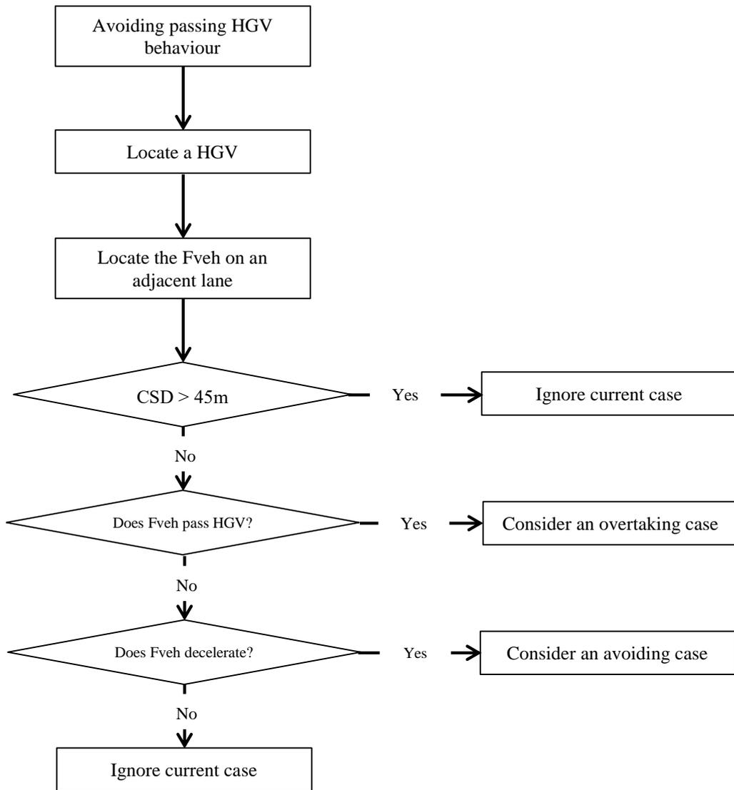
**Figure 4.5: Method of estimating avoiding passing HGV**
