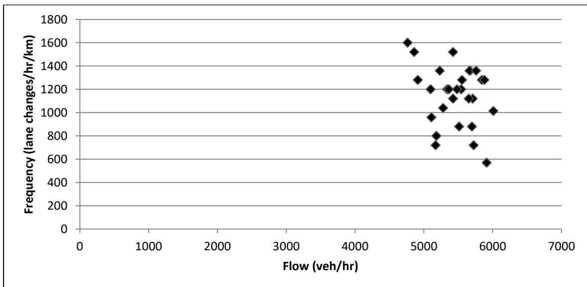
**Figure 3.5: Frequency of lane changing for the M6 (4-lane motorway) (Site No. 9)**
