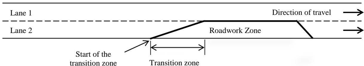
**Figure 7.31: Illustration of the M67 roadwork site layout**
