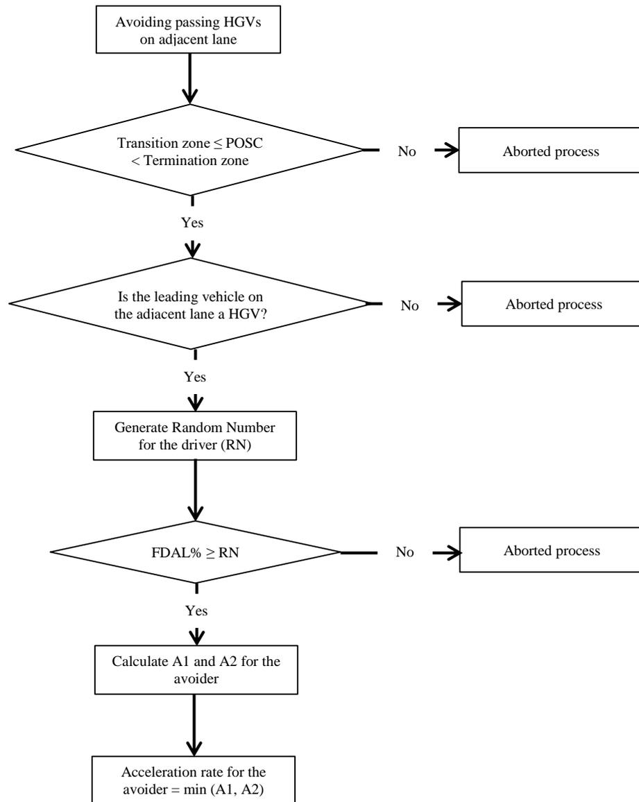
**Figure 6.20: Flow chart for modelling the “avoiding” of passing HGVs on adjacent lane**
