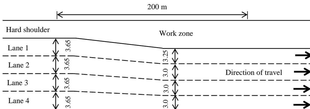
**Figure 4.2: Schematic layout of the M6 roadwork site**
