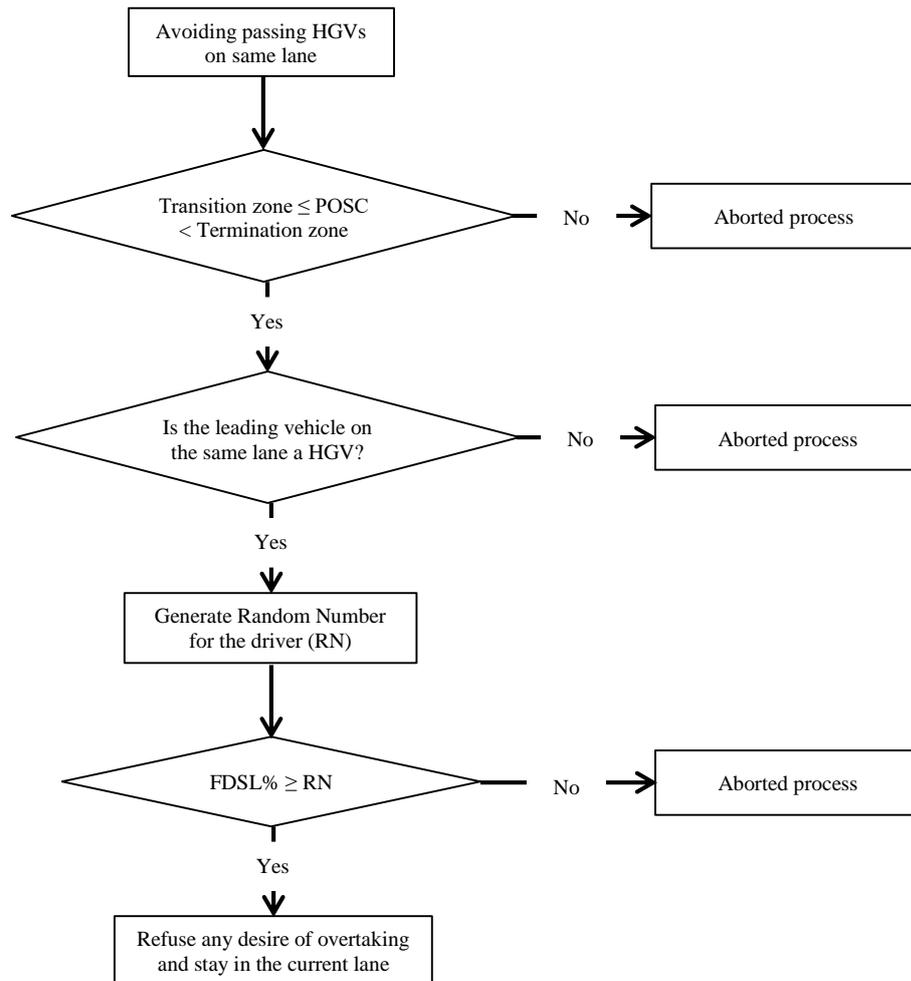
**Figure 6.22: Flow chart for modelling the “avoiding” of overtaking HGVS on the same lane**
