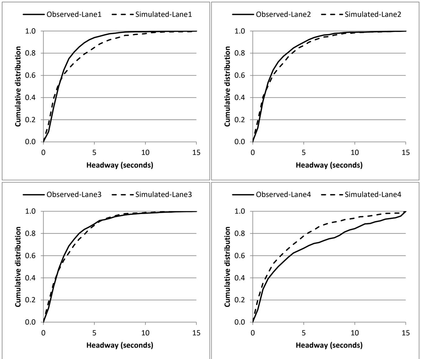
**Figure 7.19: Calibration - simulated versus observed cumulative distribution of headways in lanes 1, 2, 3 and 4 on the M6**
