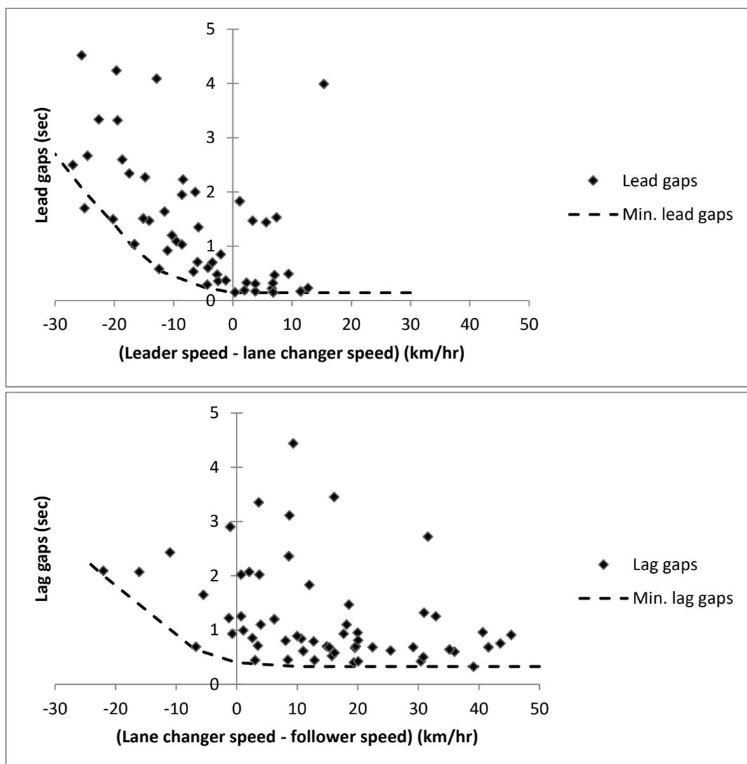
**Figure 3.8: Relationship between relative speeds on the size of accepted lead and lag gaps based on data from the M67 (Site No. 2)**
