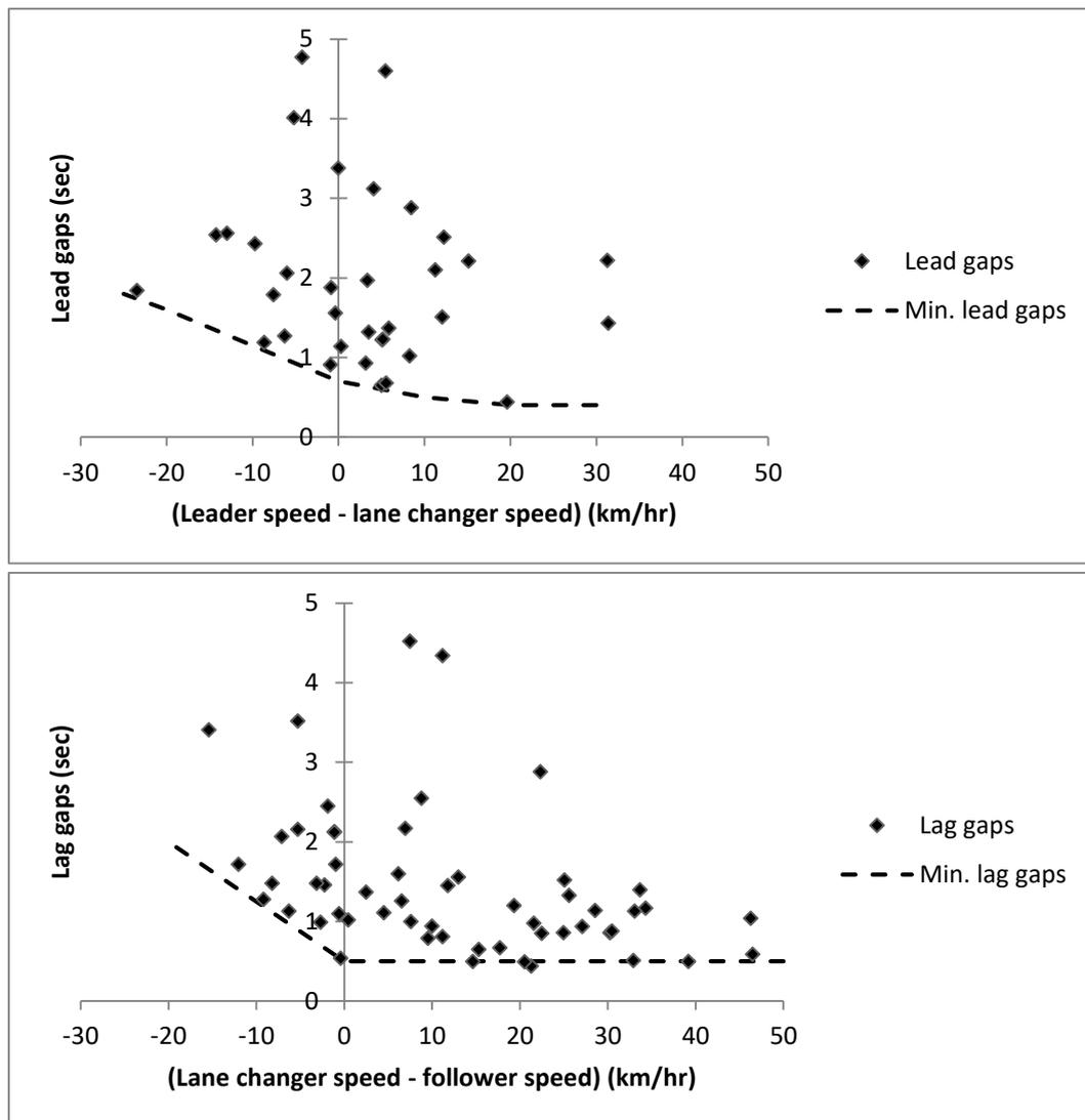
**Figure 3.9: Relationship between relative speeds on the size of accepted lead and lag gaps based on data from the M61 (Site No. 4 and 5)**
