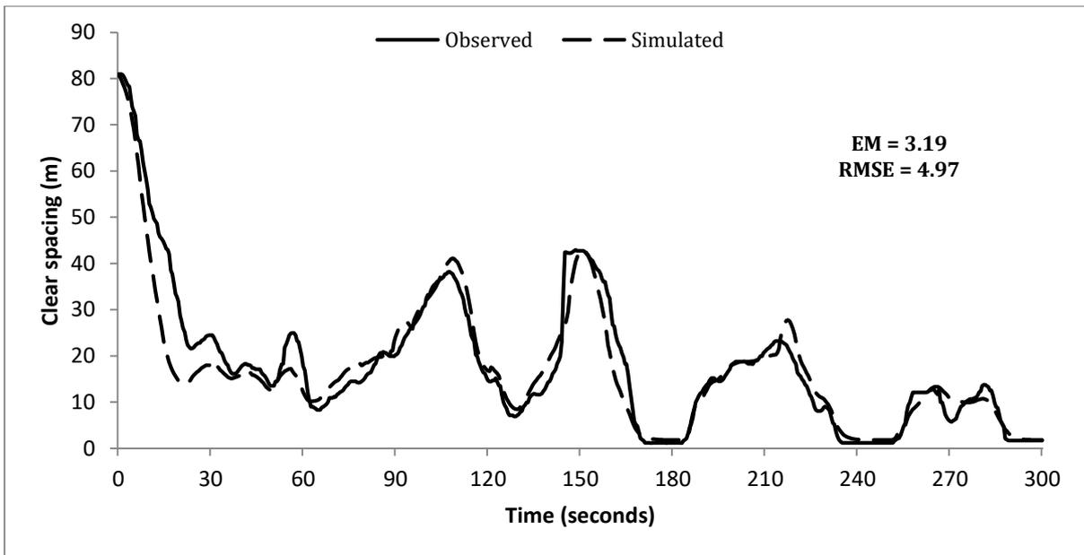
**Figure 7.7: Calibration - simulated versus observed clear spacing based on data from Panwai and Dia (2005)**
