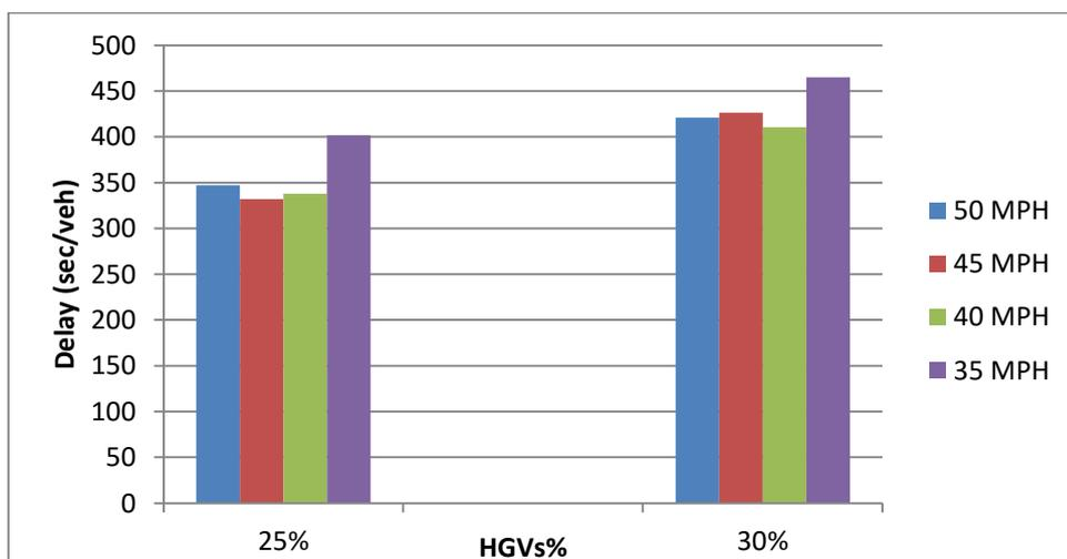
**Figure 8.23: Effect of roadwork speed limits (with 50% complying with speed limits) on 4 lanes section delay (narrow lanes)**
