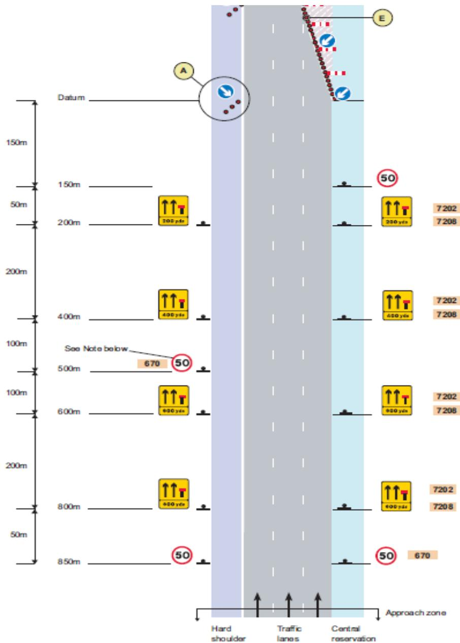
Figure 6.18: Signage layout at roadwork sections (Traffic Signs Manual - Chapter 8, 2009)
