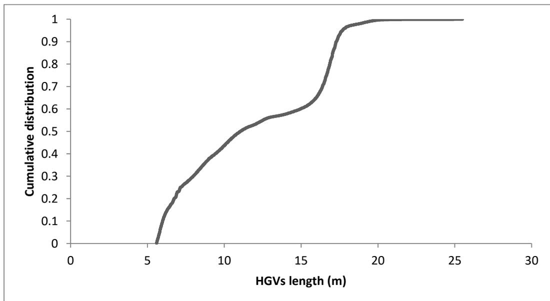
**Figure 6.6: Cumulative distribution for HGV lengths based on data from the M25**
