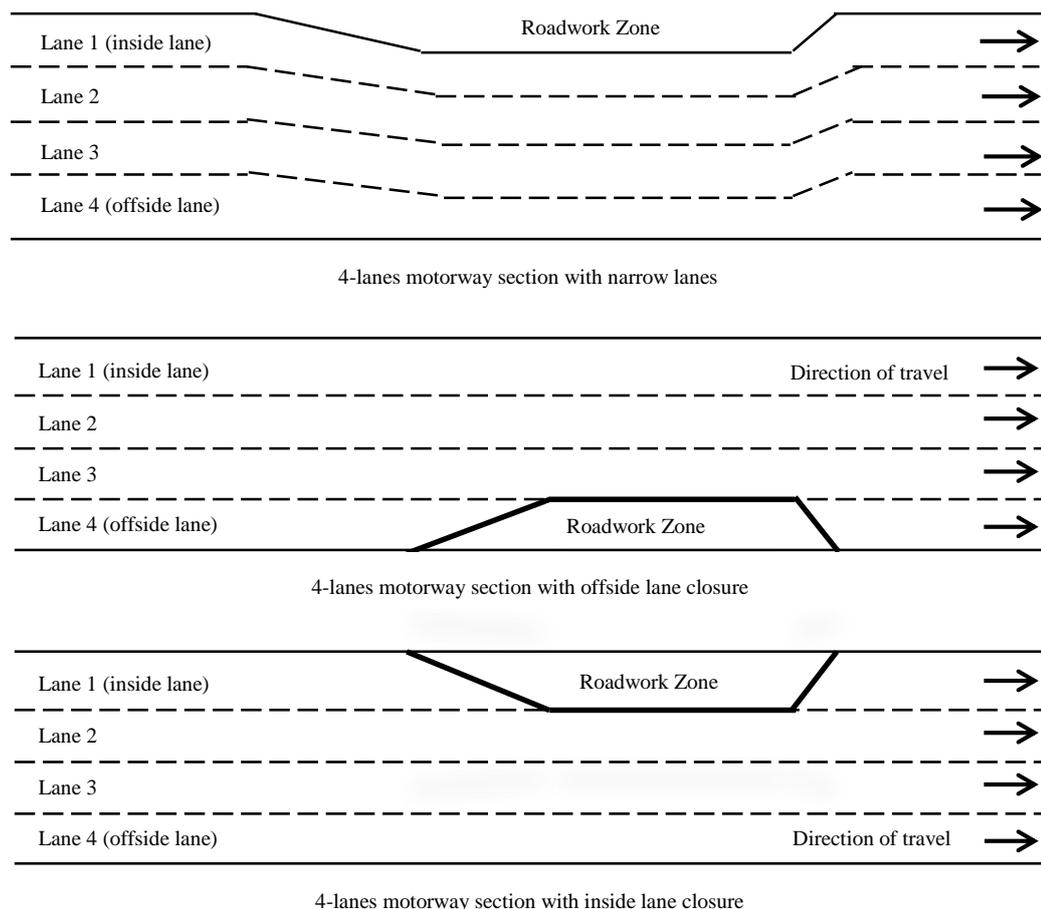
**Figure 8.9: Schematic layouts of the tested 4-lanes motorway roadwork sections**
