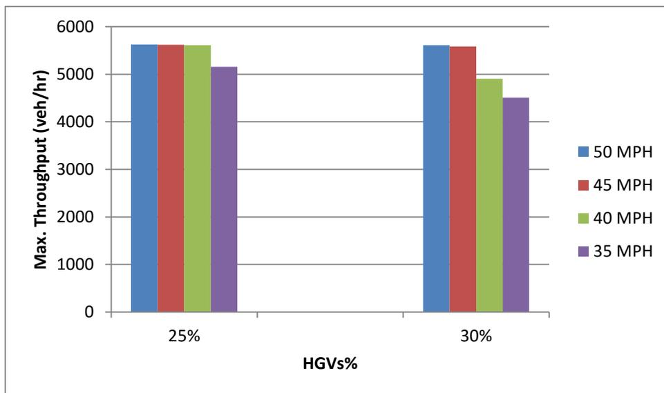
**Figure 8.24: Effect of roadwork speed limits (with 100% complying with speed limits) on 4 lanes section capacity (narrow lanes)**
