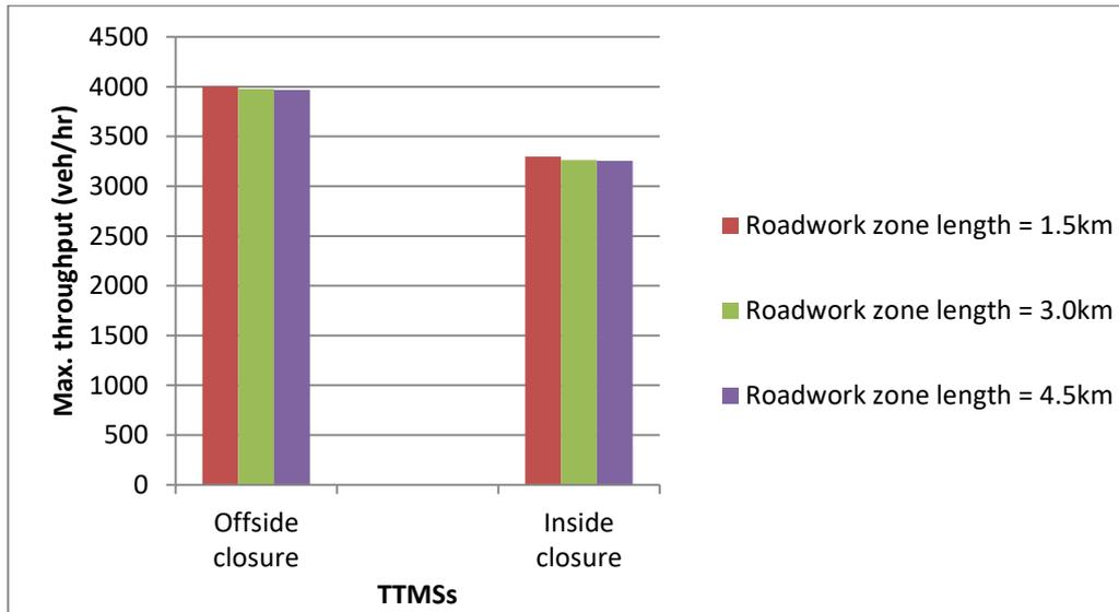
**Figure 8.18: Effect of roadwork zone lengths on 3-lanes section capacity (lane closures)**
