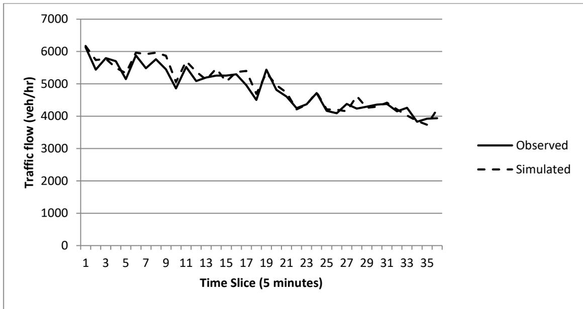
**Figure 7.18: Calibration - simulated versus observed traffic flow data (M6, J31 – J32)**
