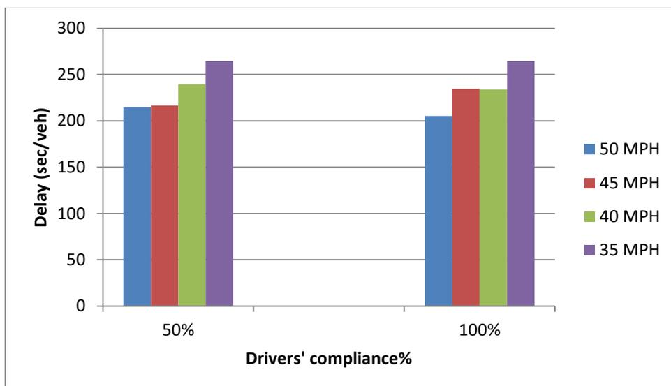
**Figure 8.27: Effect of roadwork speed limits on 3-lanes section delay (lane closure)**
