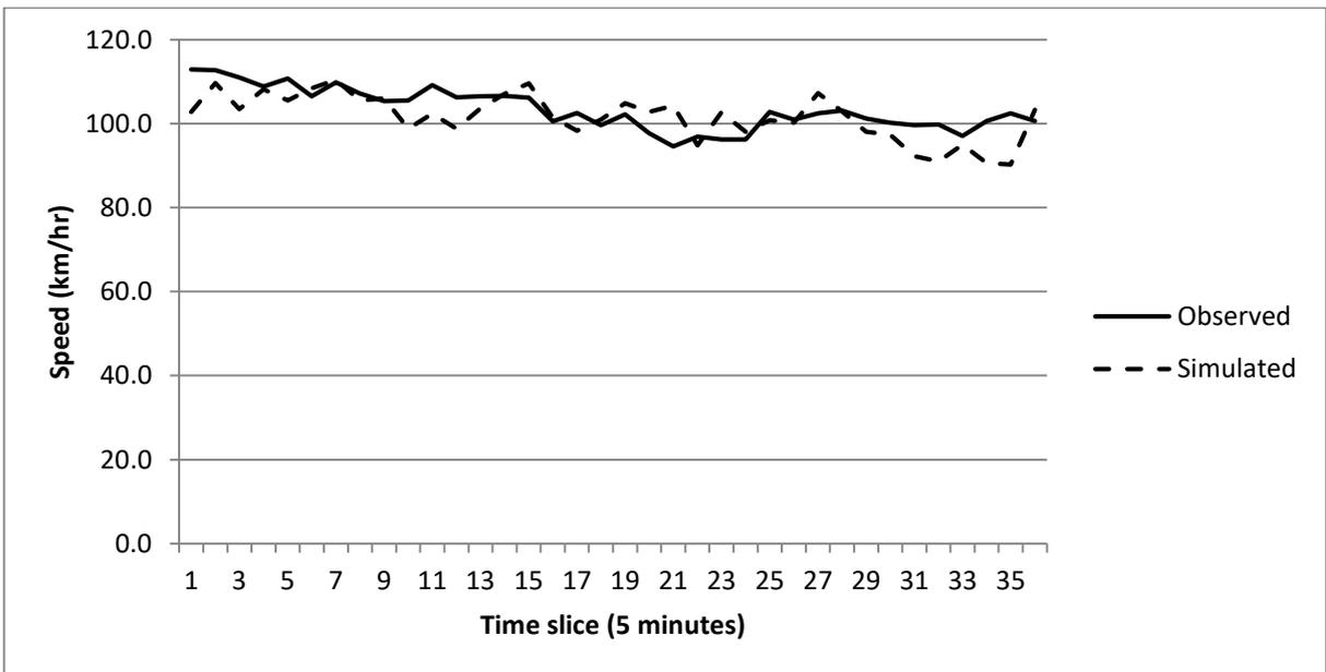
Figure 7.27: Validation - simulated versus observed speed data (M42)
