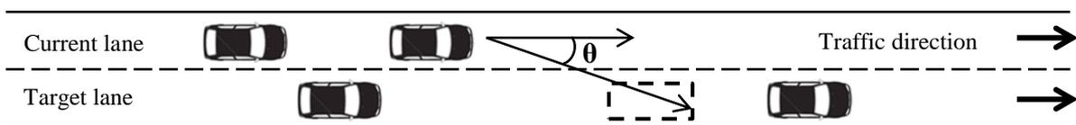
**Figure 2.4: Illustration of the turning angle ( $\theta$ ) of the subject vehicle**
