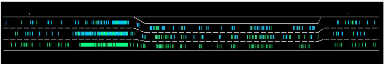
**Figure 8.8: Typical screenshot from the developed simulation model (3-lanes motorway roadworks section with narrow lanes scheme at high flows and high HGVs%)**
