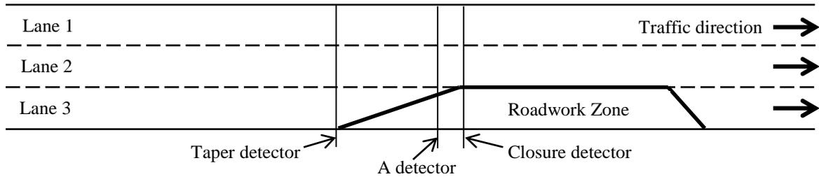
**Figure 5.4: Illustration of loop detectors positions**
