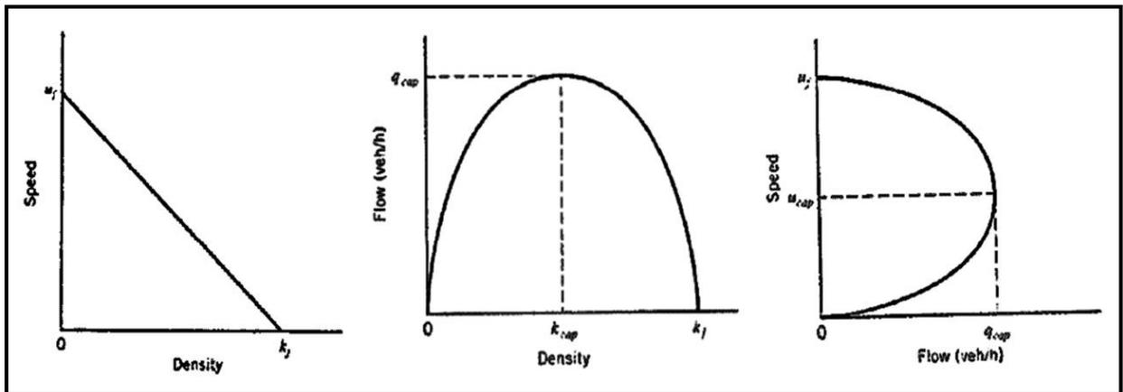
**Figure 2.2: Fundamental diagrams of speed-density, flow-density and speed-flow (Mannering and Washburn, 2012)**
