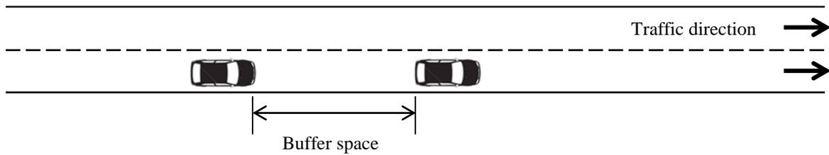
**Figure 6.9: Illustration of the safety buffer space**
