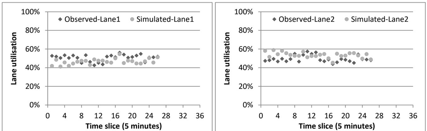
Figure 7.30: Validation - simulated versus observed lane utilisation data for lanes 1 and 2 on the M602
