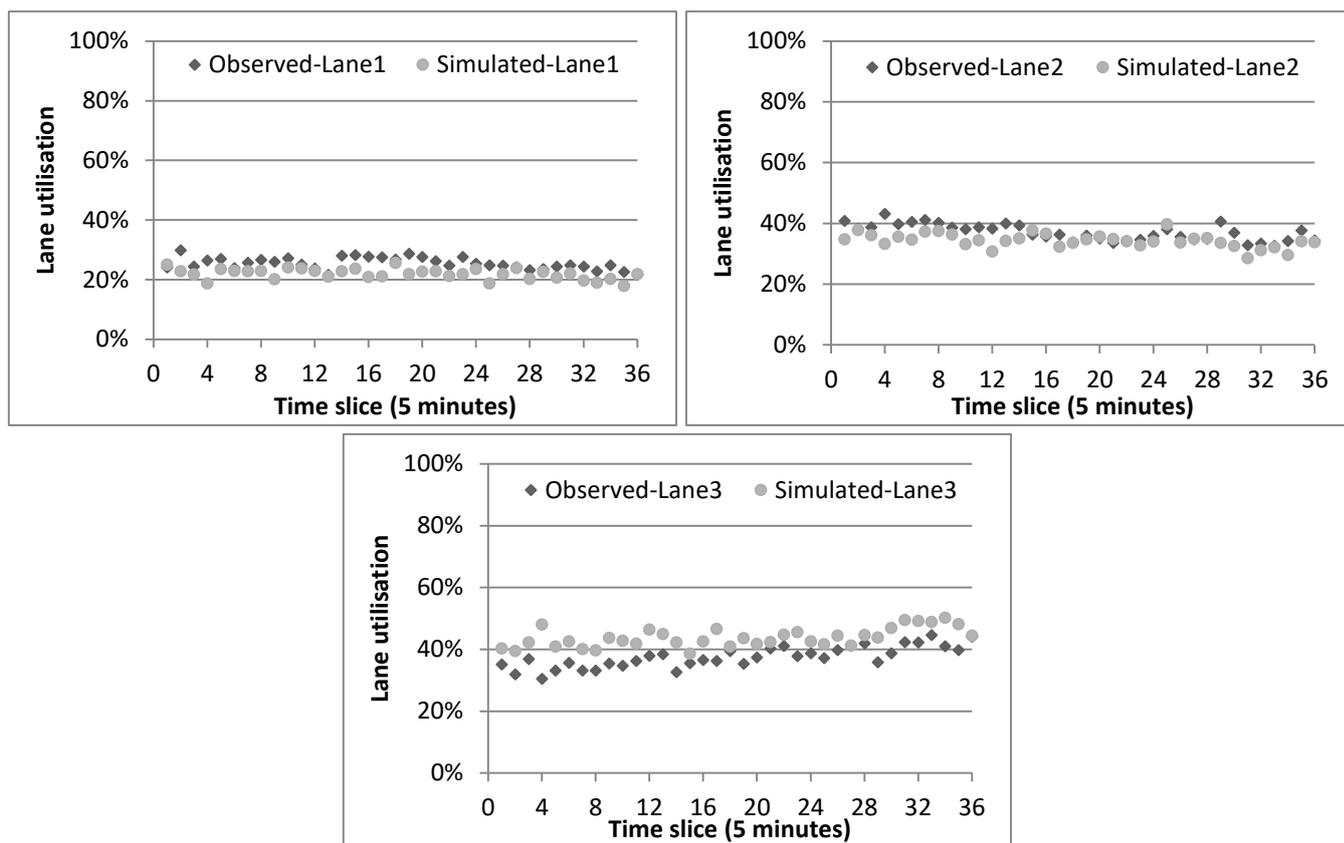
**Figure 7.28: Validation - simulated versus observed lane utilisation data for lanes 1, 2 and 3 on the M42**
