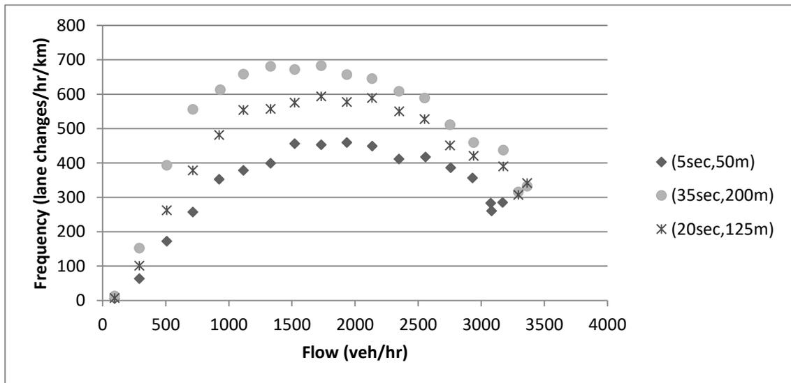
**Figure 7.9: Calibration - simulated lane changing frequency for a 2-lanes normal motorway section under high, low and average values of THRT and THRD**
