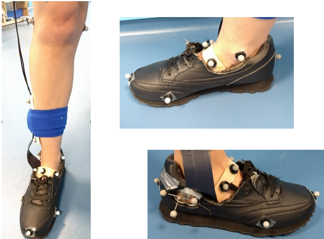
Figure 3.7 Location of anatomical markers; posterior heel, 1 st & 5 th metatarsal heads, 2 nd toe, medial and lateral knee condyles and malleoli, and tracking markers; shank, calcaneus and midfoot.
