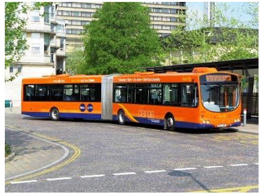
Figure 5-12: Typical example of 160-passengers capacity BRT Rolling Stock in Christchurch
